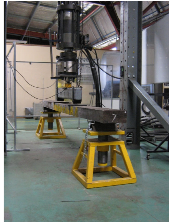
Figure 2. Four point bending test setup in laboratory
