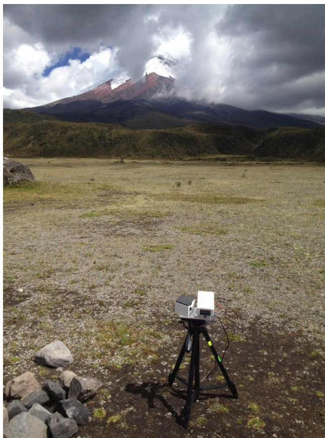
Figure 5. Raspberry Pi camera-based spectrometer applied to measurements of sulphur dioxide gas release from Cotopaxi volcano, Ecuador.
