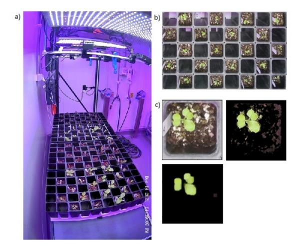
**Figure 1:** Experimental setup in ground-based laboratory – a) experimental rig, b) top view image from visible colour camera, c) basic image processing to segment plant leaves from the background
