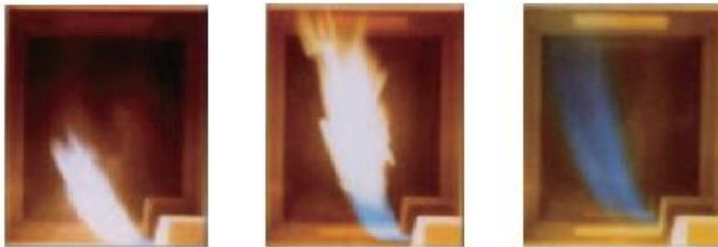
Figure (New) Combustion air temperature of 1100 °C and O 2 concentration (Gupta et al., 1999)
