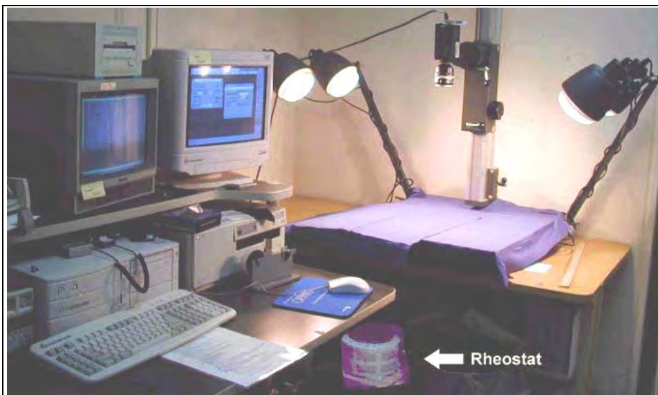
Figure 4.6: Typical image analysis system: camera with uniform lighting or scanner to capture image, computer with program to evaluate fabrics and monitor to visually evaluate images.
