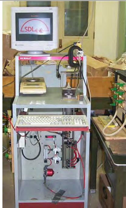
Figure 3.3 The Shirley Developments LTD. Micromat Fineness and Maturity Tester (FMT), a dual-compression instrument 84 (ASTM, 1994). Photo supplied by J. Montalvo 85 (Montalvo, 2002).
