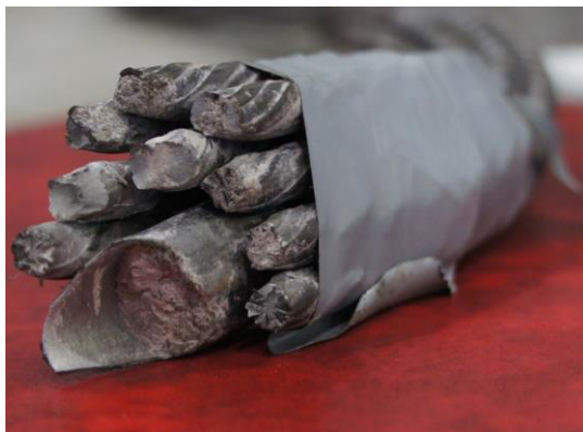
Fig. 7. Tensile and shear failure of cable bolt.
