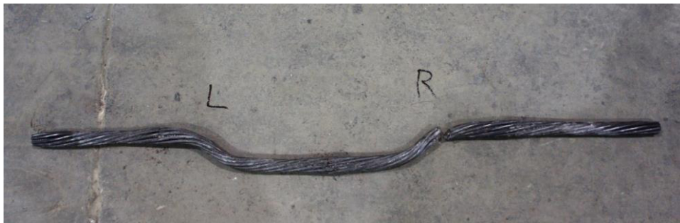
Fig. 6. Failure angle of cable bolt.
