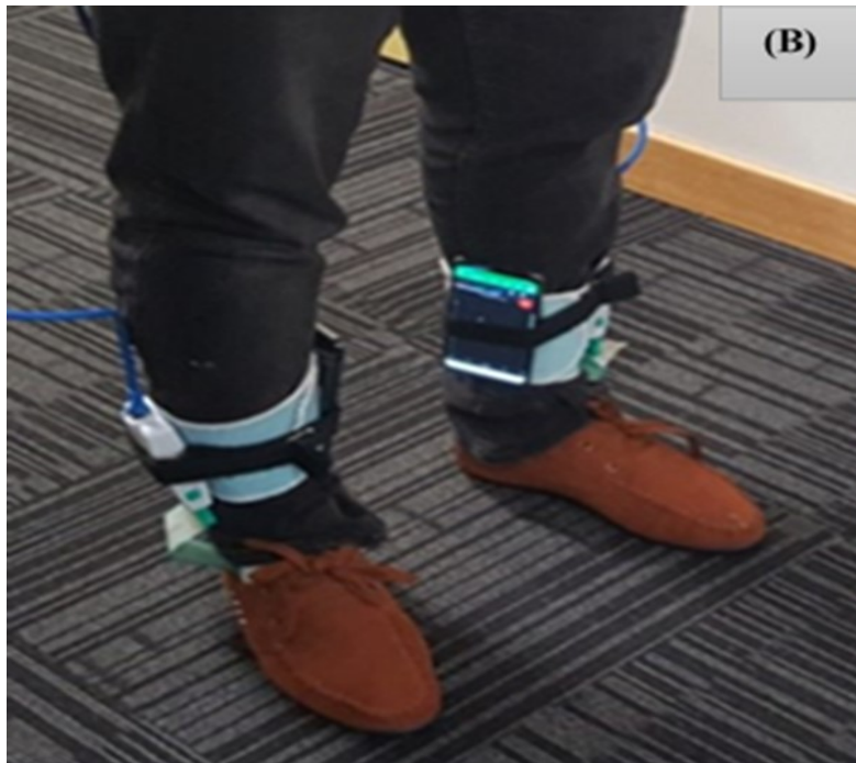
Figure 3.16: A and B: An example for two people wearing insole sensors and smartphones during the test
