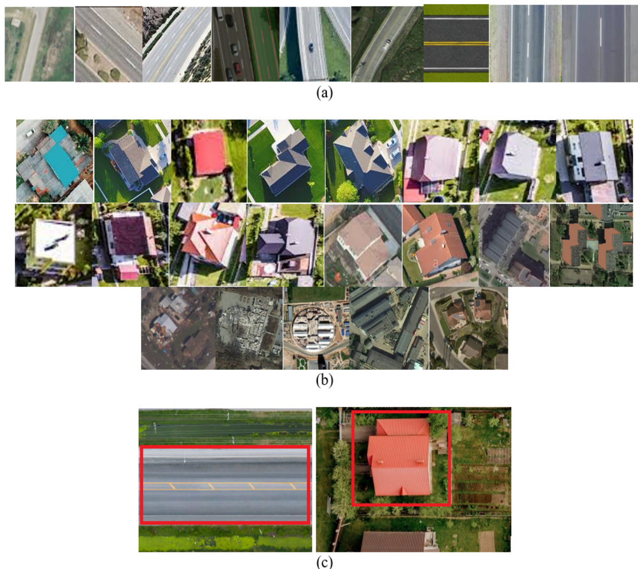
Figure 7. (a) Subset of aerial road images used for training (b) Subset of aerial building images used for training (c) Haar Cascade Classifier Results.
