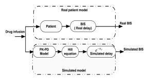
Fig. 3. The representation of the real and simulated BIS
