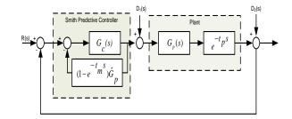
Fig. 4. The control structure with the Smith predictor
