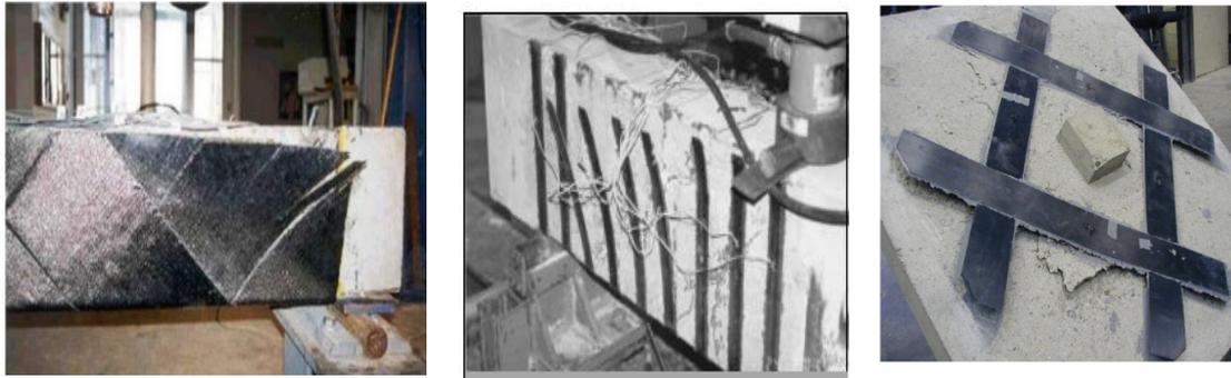
(a) FRP rupture with debonding
