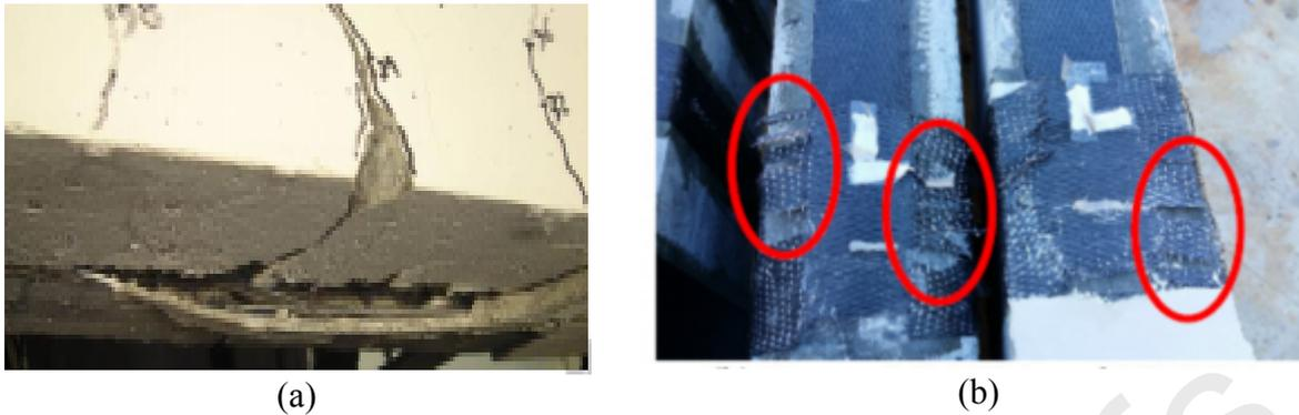
Fig. 17 Rupture of (a) NSM FRP strips and (b) EB sheets [122,139]
