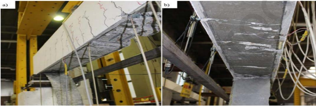
Fig. 15 Debonding failure at the (a) FRP-concrete (b) concrete-adhesive interfaces [138]
