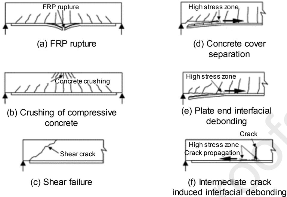
Fig. 12 Typical failure modes of FRP-strengthened structures [124]
