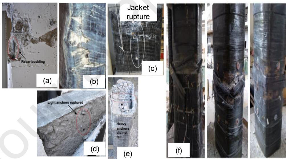
Fig. 3 A typical FRP-wrapped column under axial compression: (a) Concrete crushing in the control specimen, (b, c, f) FRP rupture and (d) anchor rupture [46,48,49]
