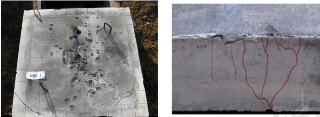
(a) Blast damage of a control specimen      (b) Blast damage of a FRP-retrofitted specimen
