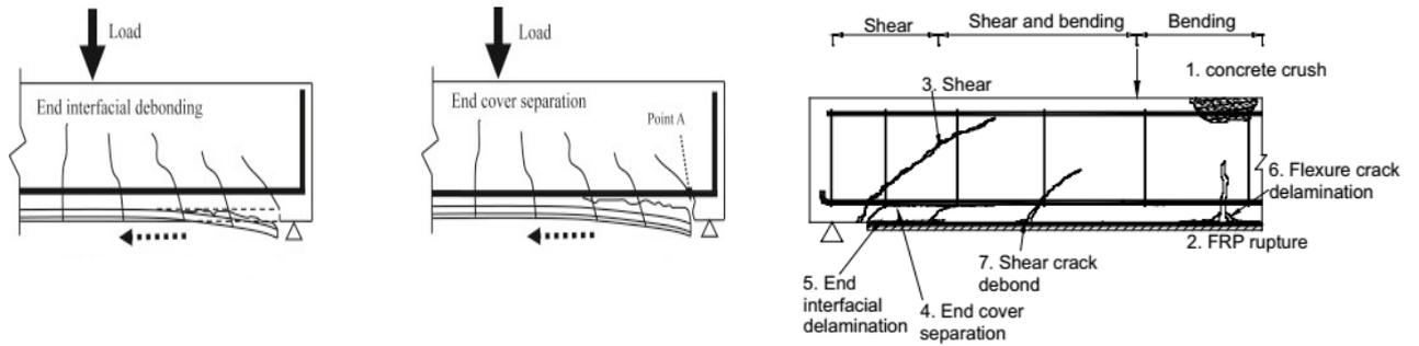
Fig. 14 Debonding failure of FRPs: (a) NSM technique [53] and (b) EB system [137]
