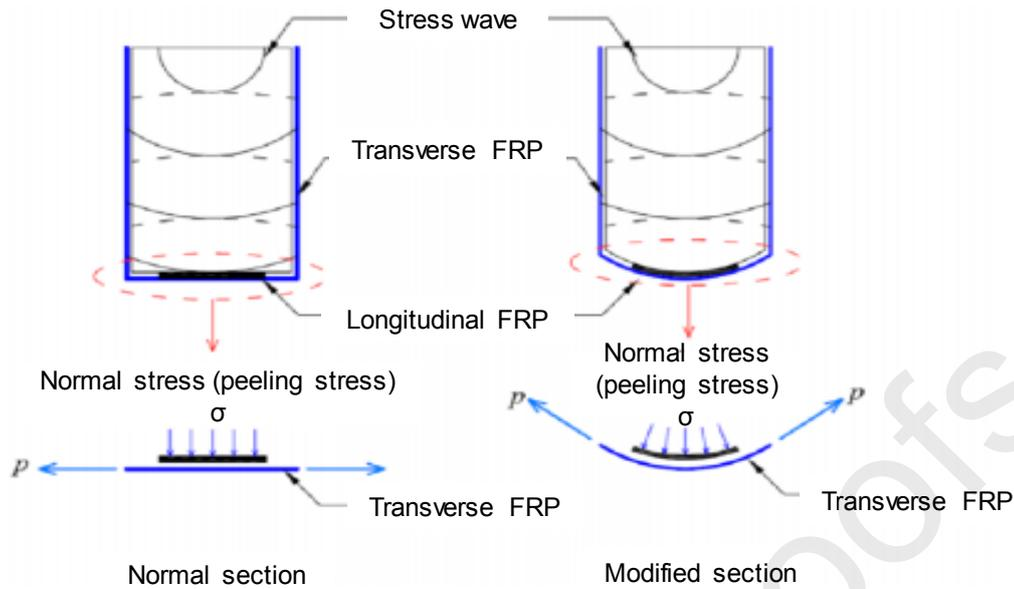
Fig. 16 Debonding mechanism under impact [122]
