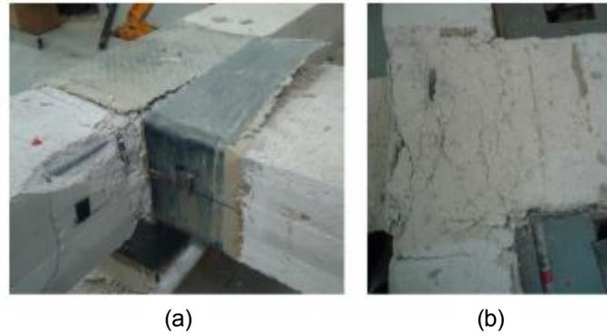
Fig. 9 A typical FRP-wrapped beam-column joint under loading (a) before and (b) after the removal of the FRP sheet [35]
