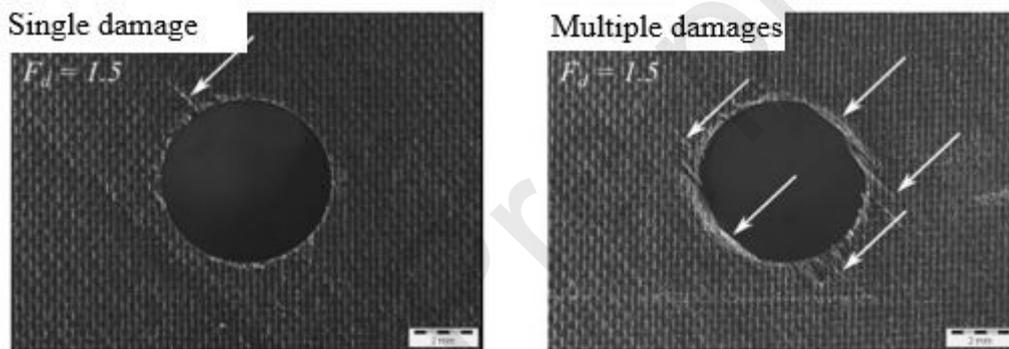
Fig. 18 Fibre damage during drilling of holes in CFRP [162]
