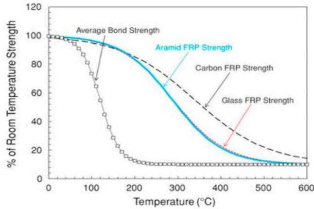
Fig. 11 Variations in FRP bond strengths with temperature [8]
