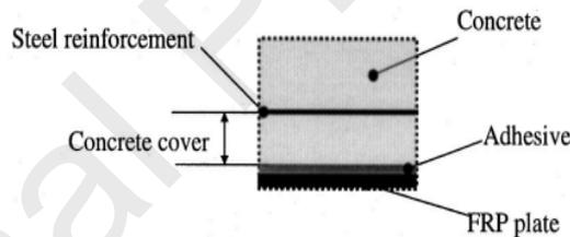
Fig. 13 Potential failure zones in FRP-strengthened concrete systems [125]
