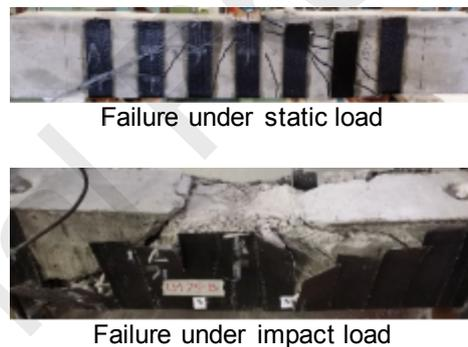
Fig. 6 Typical failure of FRP-strengthened RC beams under impact loading [69]
