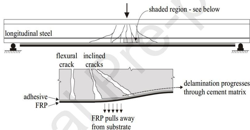
Fig. 8 A typical FRP-strengthened beam under fatigue loading [78]
