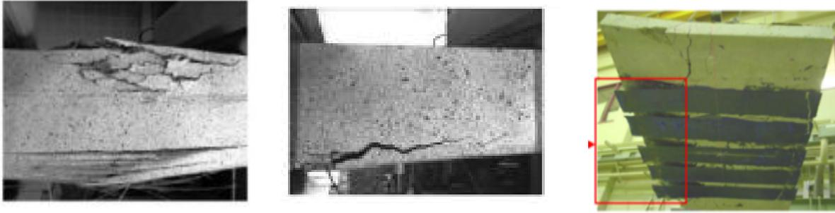
(a) Compression crushing with FRP rupture
