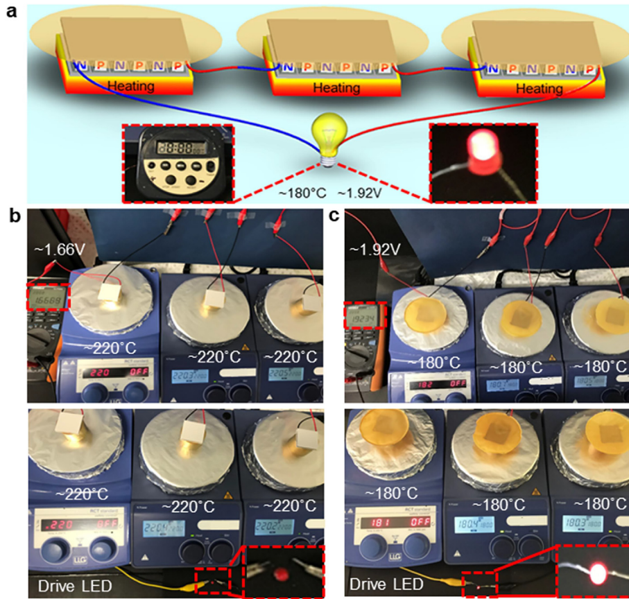
Fig. 5. Tandem connection for practical cooling from high temperature and thermal energy utilization. (a) The scheme of BN50-PI50 for efficient high temperature heat dissipation and practical thermal energy conversion. (b) The optical picture of practical tandem of an air-cooling based TE module. (c) The optical picture of a practical tandem of BN50-PI50 loaded TE module.
