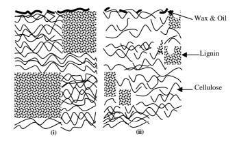
FIGURE 02: Typical structure of (i) untreated and (ii) alkalized cellulose fibre (Leonard & Martin, 2002).
