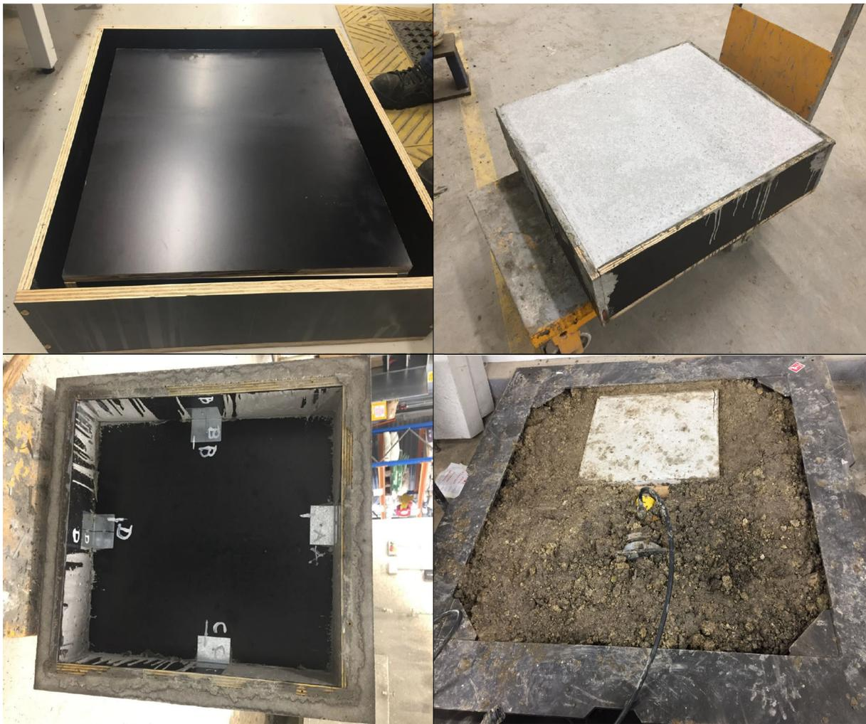
**FIGURE 8** Formwork and casting of the concrete test specimen.
