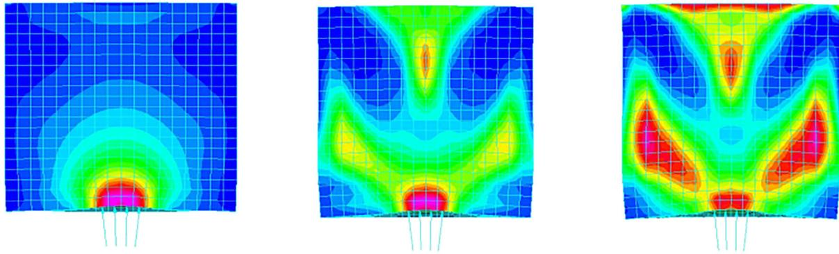
FIGURE 18 Comparison of crack propagation in experimental results with strain concentrations in numerical model.
