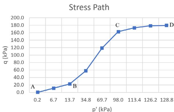
FIGURE 16 Stress path of Mohr Coulomb soil model during horizontal load application.
