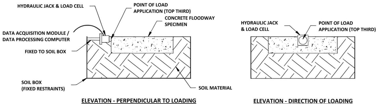
**FIGURE 9** Sketch indicating how the load was applied to the test specimens.
