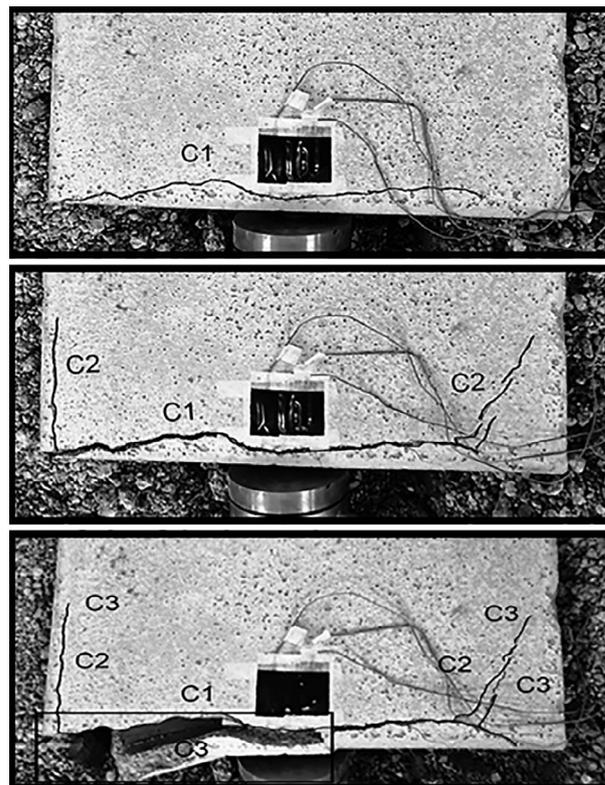
FIGURE 11 Crack propagation within concrete floodway Specimen 2.
