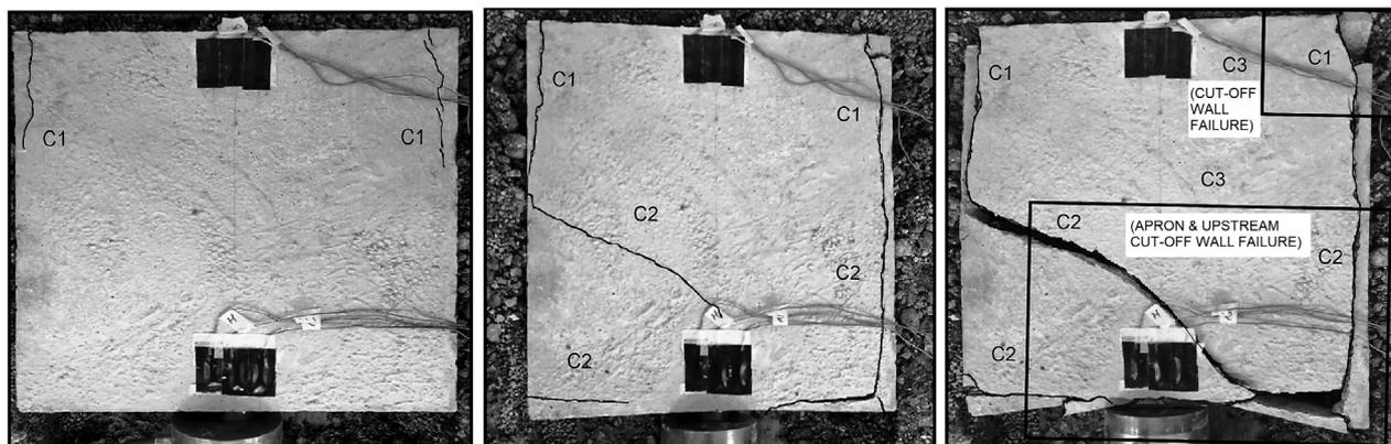
FIGURE 10 Crack propagation within concrete floodway Specimen 1.
