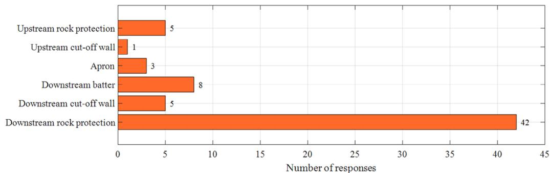
FIGURE 4 Survey question: In your experience which floodway component is most susceptible to damage during an extreme flood event? What is the likely cause of this damage? (Greene et al., 2020b).
