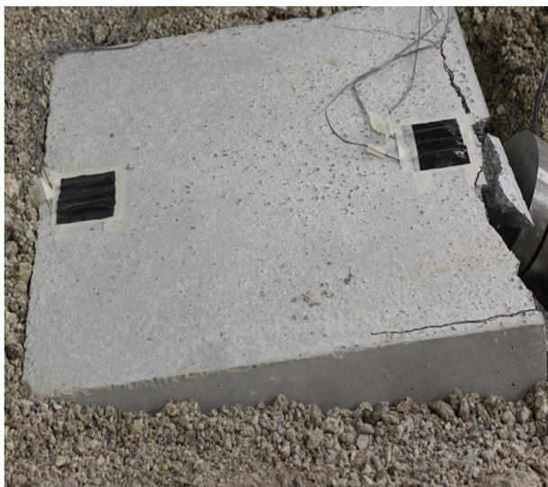
**FIGURE 12** Vertical displacement of concrete floodway Specimen 2 at failure.
