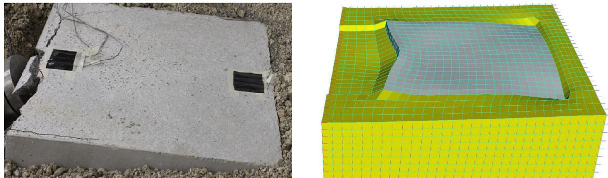
FIGURE 19 Visual comparison of vertical displacement between experiment and numerical model (10% exaggeration).
