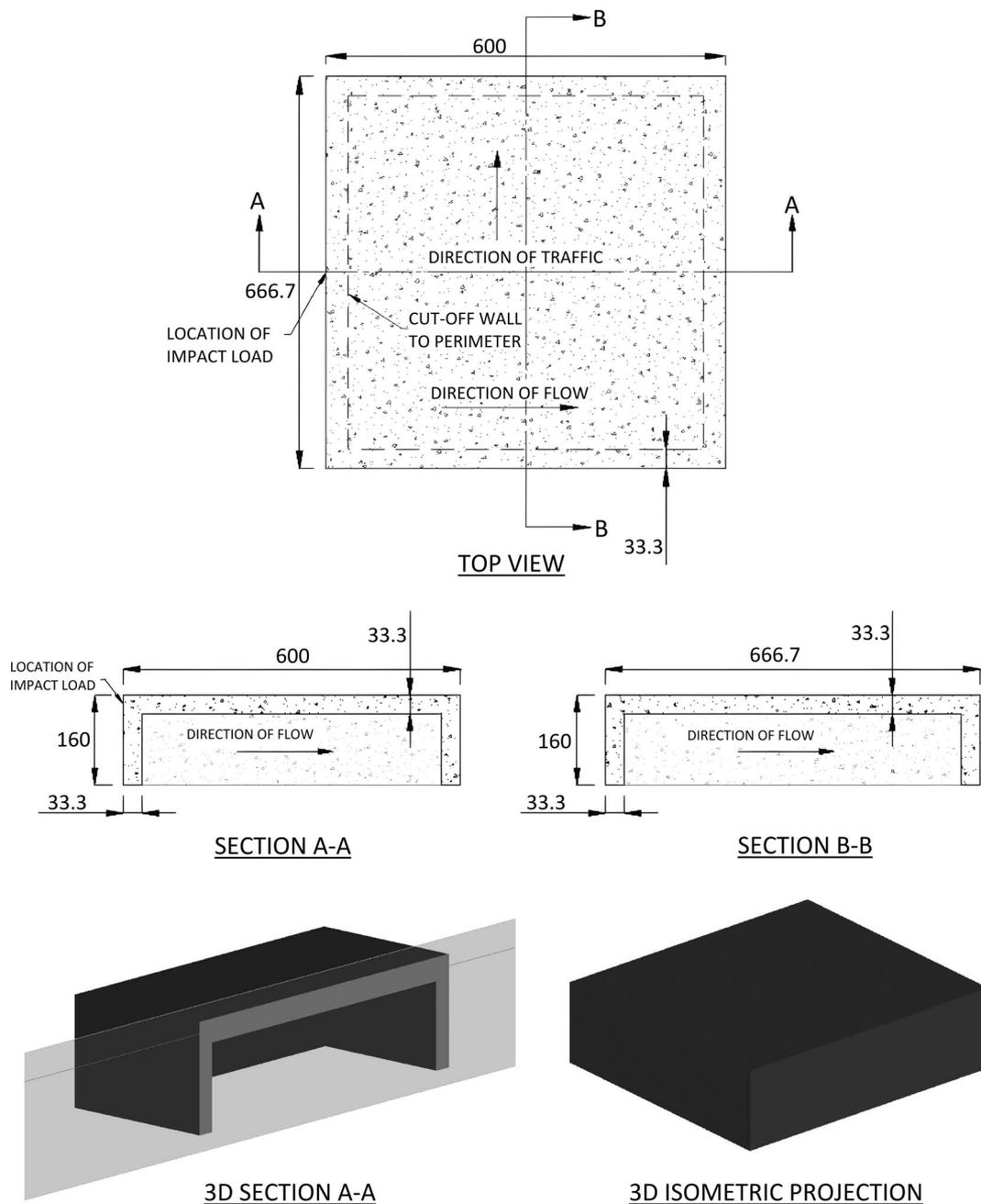
FIGURE 7 1:7.5 scale floodway apron model.
