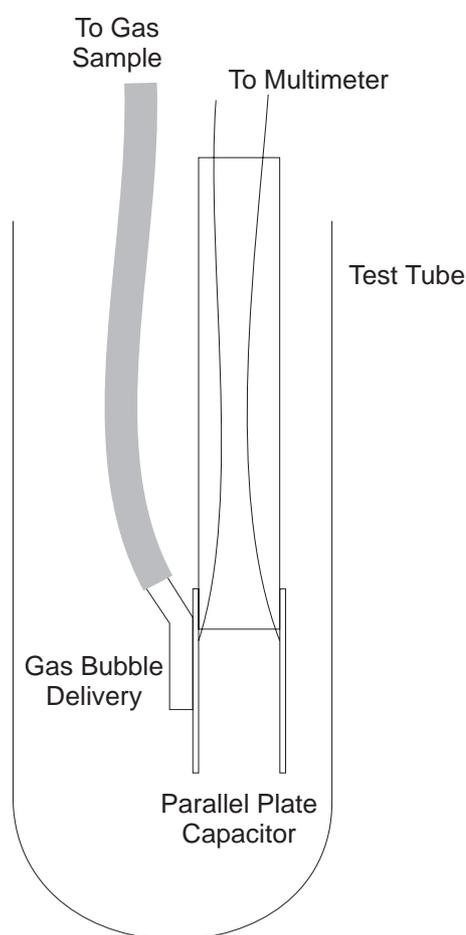
(b) Layout of the capacitor sensor within the test tube.
