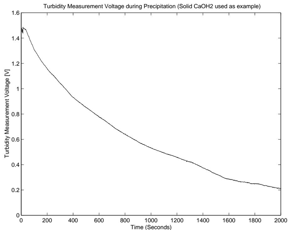
Figure 10.17: An example turbidity measurement of static precipitation as the cell filled with solid  $Ca(OH)_2$  precipitate was allowed to settle. Signal noise for the first 10 seconds was due to precipitate having just been injected into the cell causing turbulence, and some non-homogeneity of the solution.
