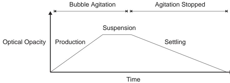
Figure 3.5: Conceptually observed amount of suspended  $CaCO_3$  within the test tube assembly (conceptual only).
