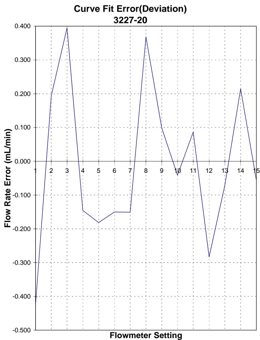
Figure F.6: 3227-20 flowmeter error between supplied calibration information and the theoretical calibration model.
