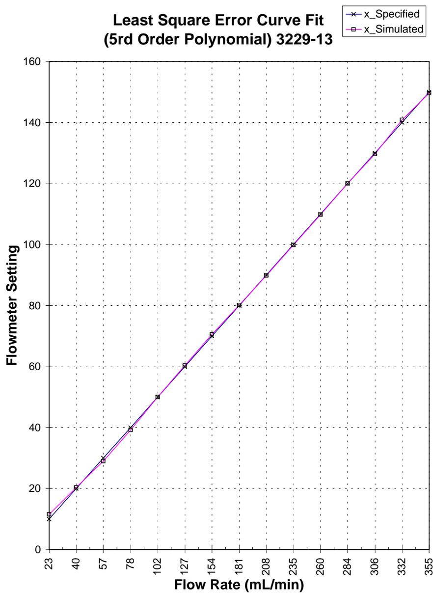
Figure F. 7: 3229-13 flowmeter calibration comparison between supplied calibration information and the theoretical calibration model.
