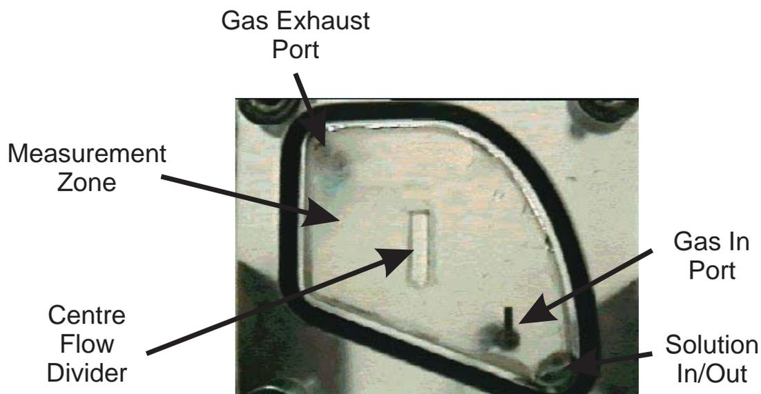
Figure 4.10: The empty ‘teardrop’ cell. Visible is the cell void, the center flow divider, and the three ports for the combined indicator chemical in/out (bottom), the sample gas in (towards the center), and sample gas out (top).
