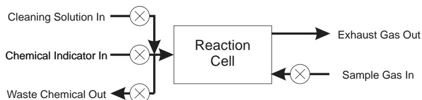
(c) Split input functions on one port with four upstream pumps. This was the configuration used for the Mk.II measurement instrument prototypes.
