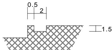
Figure A.2: Mechanical drawing for the 'oval' cell (units in mm). Also shown are the coordinates (in mm) for points within the cell.
