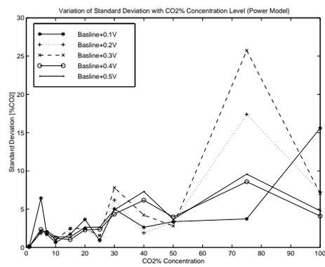
(b) Variation of standard error band ( $\pm\sigma_m$ ) for the power model.
