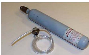
(b) Miniature gas cylinder used as the approximately 95%  $CO_2$  source.
