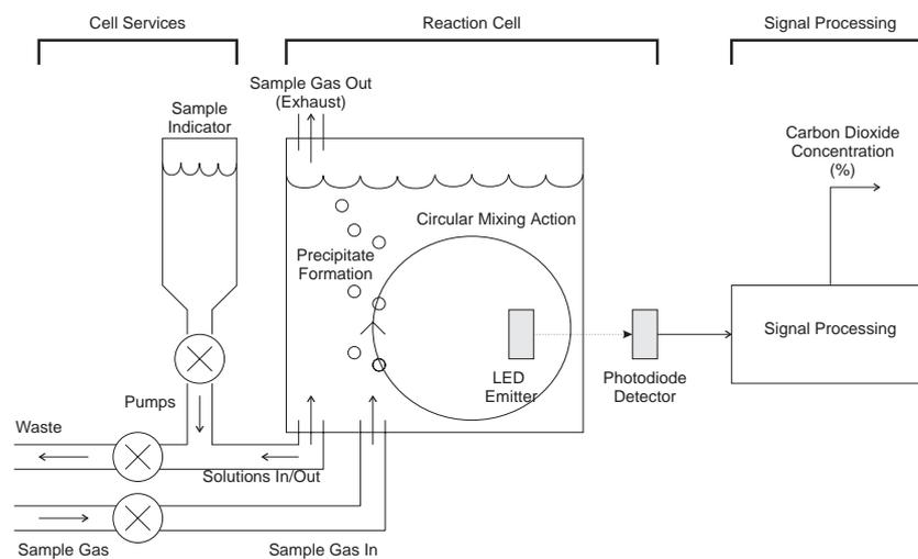
Figure 1.1: A simplified pictorial overview of the fundamental  $CO_2$  sensor system.
