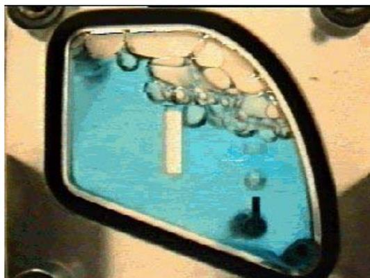
(c) 53 seconds after commencement of bubble injection. Blue dye was injected 38 seconds after commencement of bubble injection.
