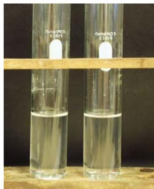
(a) Fresh indicator solution (Approx 1.7 molar). Shown is the reaction chamber (right) and the control tube (left).
