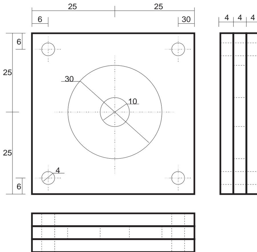
Figure A.4: Mechanical drawing for the ‘circular’ cell (units in mm). The “O” ring groove construction method is the same as presented in Figure A.3 and milled into the two outer plates. The inner 10mm ‘island’ is glued to one of the outer plates.
