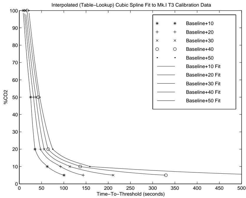
Figure B.11: Interpolated cubic spline fit curves to measured 'T3' threshold times.
