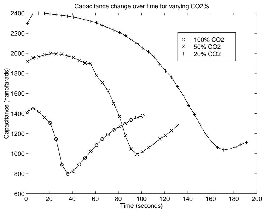
Figure D.2: Causal effect between carbon dioxide concentration and capacitance over time.
