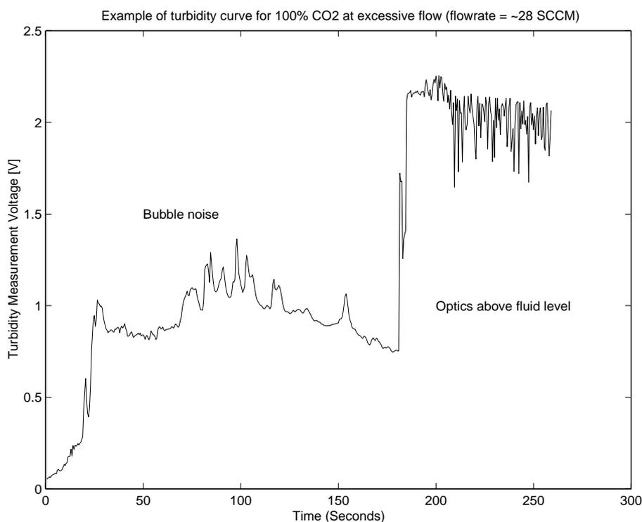
Figure 10.20: An example turbidity measurement during excessive sample gas flowrate.
