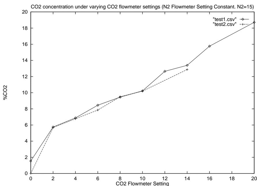
Figure F.9: Measured  $CO_2$  concentration in the supply gas stream while varying  $CO_2$  flowrate and holding  $N_2$  flowrate constant at setting 15.
