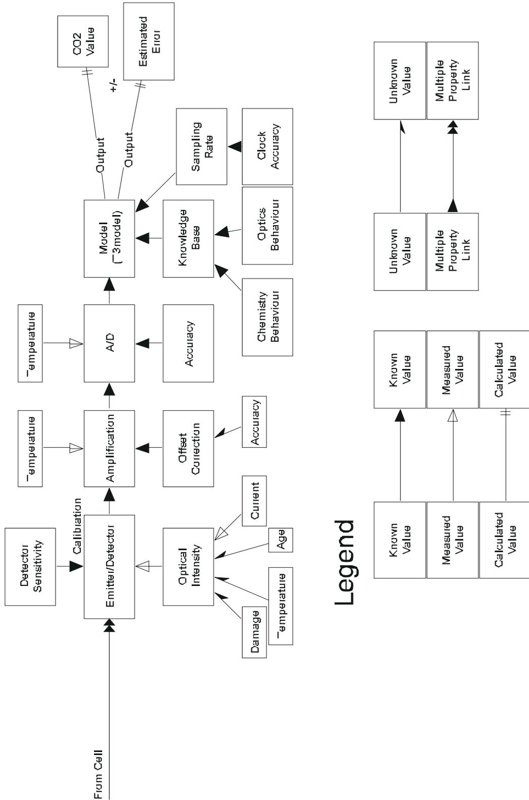
Figure 3.9: Overall instrumentation concept showing signal flows and all possible variables and influences. Continuation of Figure 3.8.
