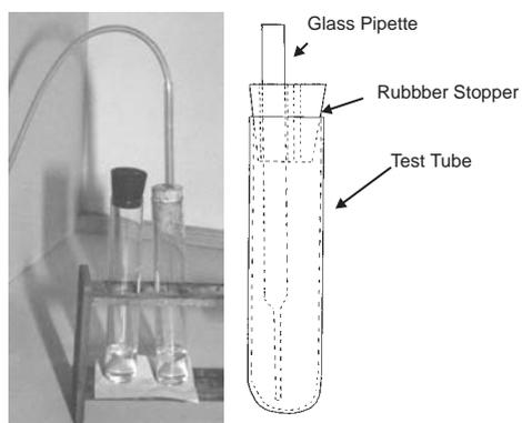
(a) Experimental configuration with the gas sample source seen in (b). A small glass pipette was used to inject the gas stream into the indicator solution.
