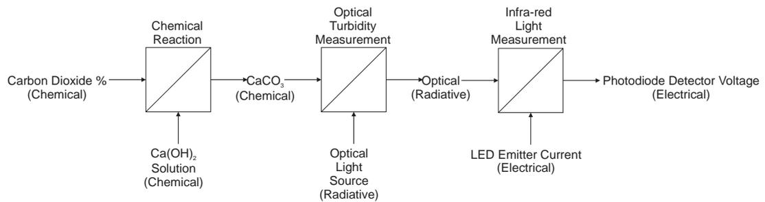
Figure 2.15: Specific transduction necessary for wet chemical analysis of  $CO_2$ . As shown, three transduction stages are necessary.
