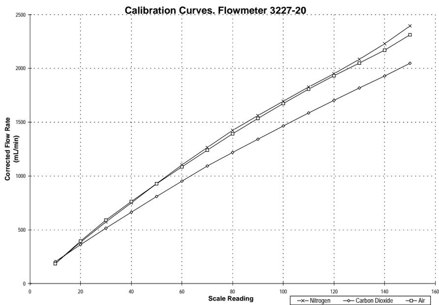
Figure F.3: 3227-20 flowmeter calibration curves for  $N_2$ ,  $CO_2$  and dry air.
