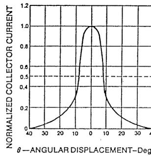
FIGURE 2—Normalized Collector Current vs Angular Displacement
