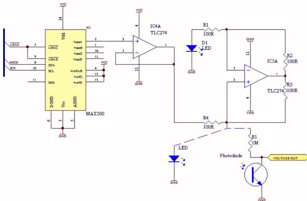
(b) The implementation of a Howland voltage controlled current source. Seen are the four stages for the LEDs and photodiodes for the two separately controllable emitter/detector pairs.
