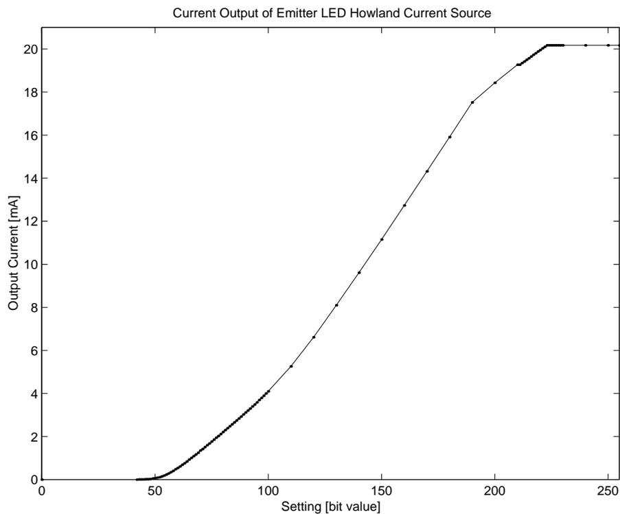
Figure 10.9: Output current from the voltage controlled current source. The actual data points used to compose the curve are shown. A deliberate increase in density of measurements at both the foot and knee of the curve was taken to improve the accuracy of the plot.
