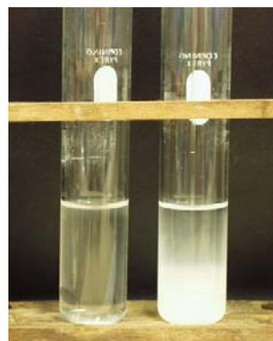
(f) Most of the precipitate has fallen out of suspension without bubble agitation (after approx 2400 seconds).
