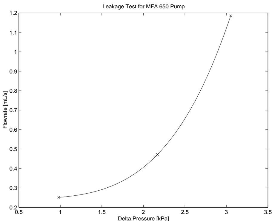
Figure 10.6: Three point plot of the flowrate through the static MFA-650 gear pump for a given port pressure differential.
