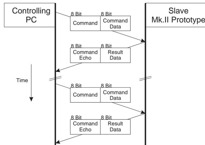
Figure 9.6: Pictorial view of the master/slave serial communications protocol developed. Two separate command exchange are shown.
