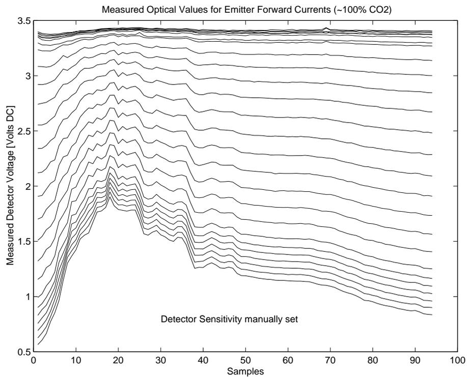
(a) Measured optical values from emitter current levels of 0 to 255 (bit value).
