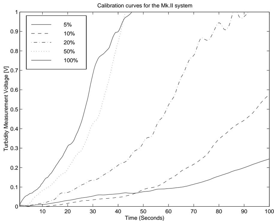
Figure 7.5: The five turbidity waveforms used to generate the Mk.II model.
