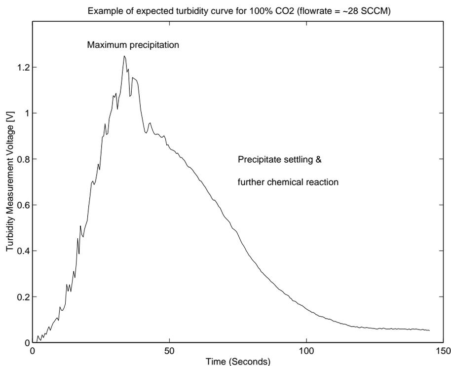
Figure 10.16: An example of the expected turbidity curve measured for 100%  $CO_2$  at a flowrate of 28 SCCM (Standard Cubic Centimeters per Minute) from initial gas injection through to eventual removal of the  $CaCO_3$  precipitate. Turbidity measurement noise during the first 40 seconds is due to non-homogeneous precipitate production and precipitate clumping.
