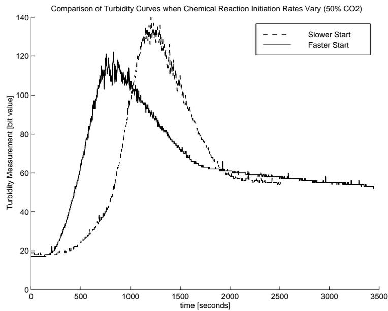
Figure 10.3: Turbidity measurement of 50%  $CO_2$  showing how slight variations in reaction rate during the initial stages of reaction shift the expected turbidity curve.
