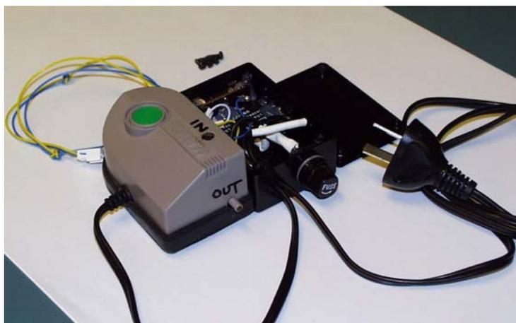
Figure 6.9: Photograph of the external ‘bellows’ type pump and its control system (lid has been removed for the photograph).
