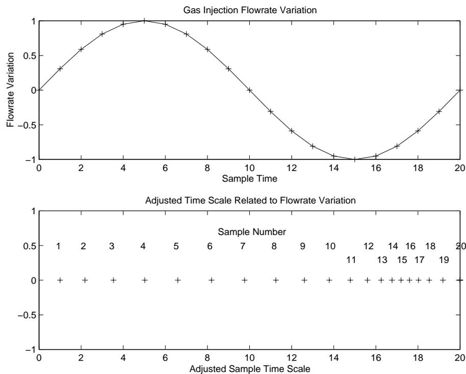
Figure 11.2: Flow rate related ‘adjusted time scale’ compensation for fluctuations in reaction rate caused by variable gas injection flow rates.
