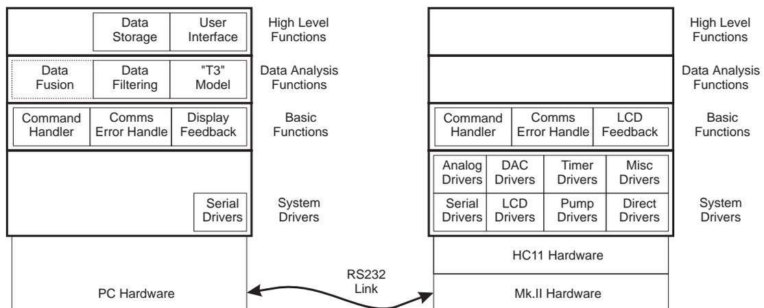
Figure 9.5: Pictorial view of the functional relationship between the master controlling program and the slave system.
