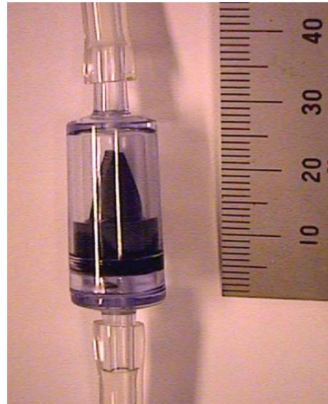
(b) Photograph of a typical check valve used within the  $CO_2$  measurement system.
