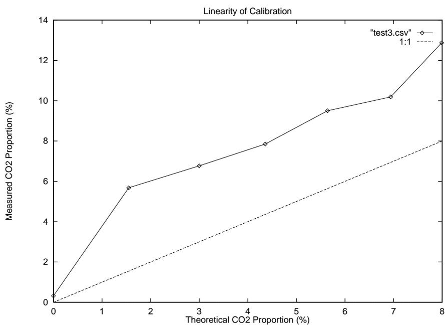
Figure F.10: Linearity of calibration scheme at low  $CO_2$  concentrations.
