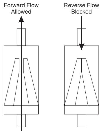
(a) The checkvalves used a small rubber valve to prevent backflow.
