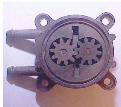
(a) Rotating inter-meshing gears in a specially designed channel, force fluid entrapped within the gear teeth from the inlet, around the outside of the channel, to the outlet.
