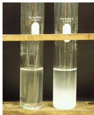
(e) Beginning of the suspension fallout without bubble agitation (after approx 1200 seconds).
