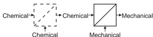
Figure 2.5: Energy flow representation of the potential mechanical transduction of  $CO_2$ .
