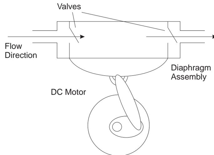
Figure 11.1: Example of a 'bellows' pump using a small DC motor for actuation.
