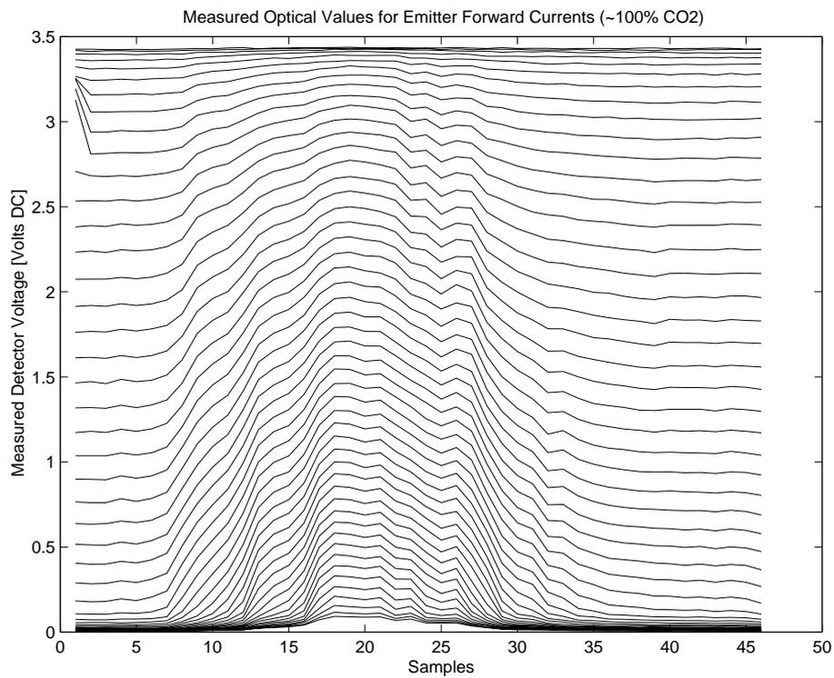
(a) Measured optical values from emitter current levels of 50 to 100 (bit value).
