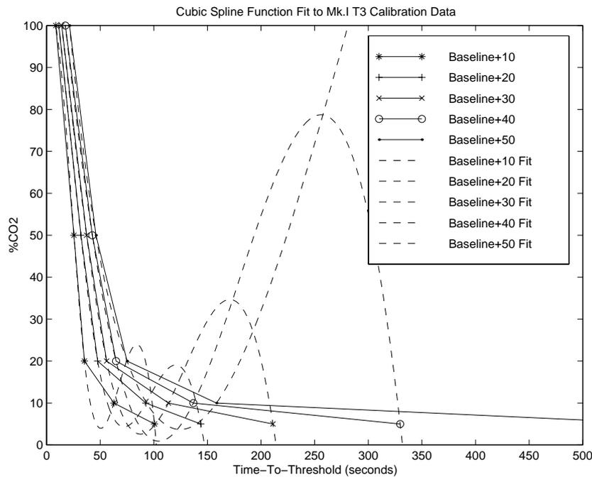
Figure B.7: Spline fit curves to measured ‘T3’ threshold times.
