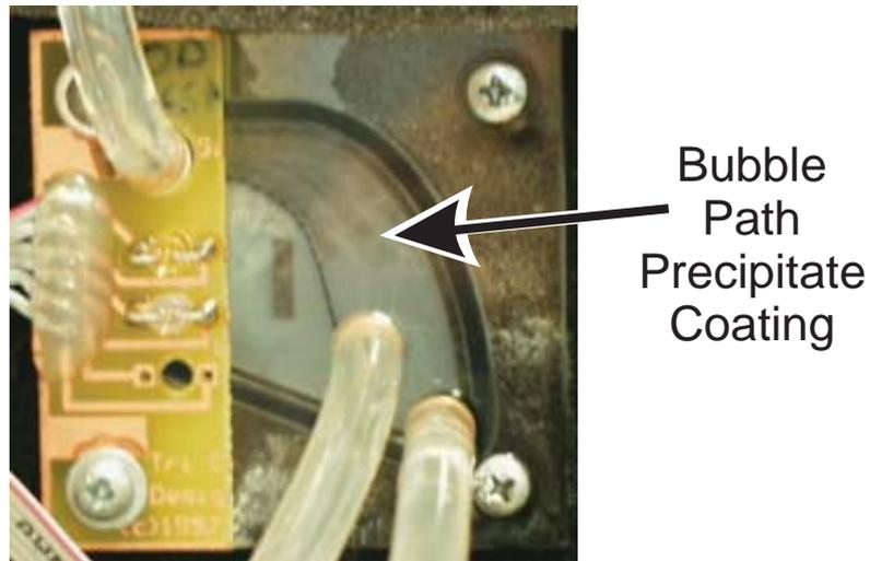
(a) Photograph of cell wall during the  $CaCO_3$  initiated optical drift tests. A significant precipitate coating (light grey) has developed in the bubble injection area (above middle tube) and following the path upward of the bubbles, plus general sheet precipitate covering the rest of the cell. (The circuit card out left carries the two sets of infra-red optics.)
