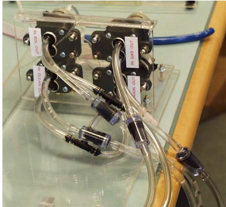
Figure 6.8: Photograph of the fluid/gas transport system used for the Mk.II prototype showing four pumps mounted on the perspex bracket) and four inline check valves (foreground).
