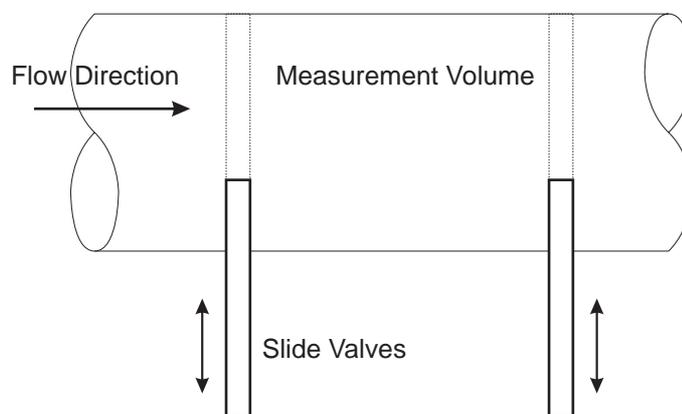
Figure 4.1: The first conceptual design for the chemical reaction cell. An inline flow cell using two slide valves to form the sides of the chamber. A center measurement area was reserved for the turbidity measurement.
