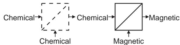
Figure 2.9: Energy flow representation of the potential chemical and then magnetic transduction of  $CO_2$ .
