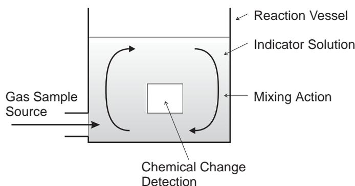
Figure 3.1: Conceptual overview of the components required for “wet chemical” analysis.
