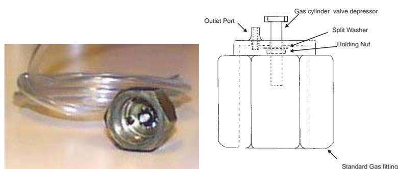
(c) Control Tap and exhaust hose coupling used to couple the gas cylinder to the glass pipette.
