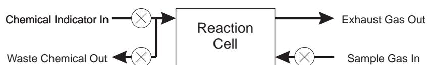
(a) Split input functions on one port with three upstream pumps. This was the configuration used for the Mk.I measurement instrument prototypes.
