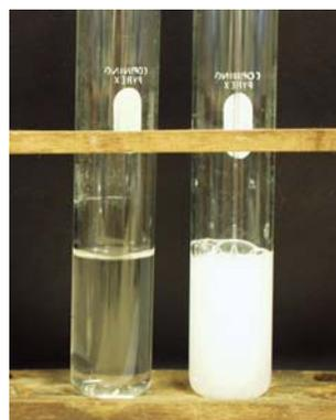
(d) The reaction chamber has reached maximum opacity (after approx 30 seconds), with the  $CaCO_3$  remaining in suspension due to the bubble motion.
