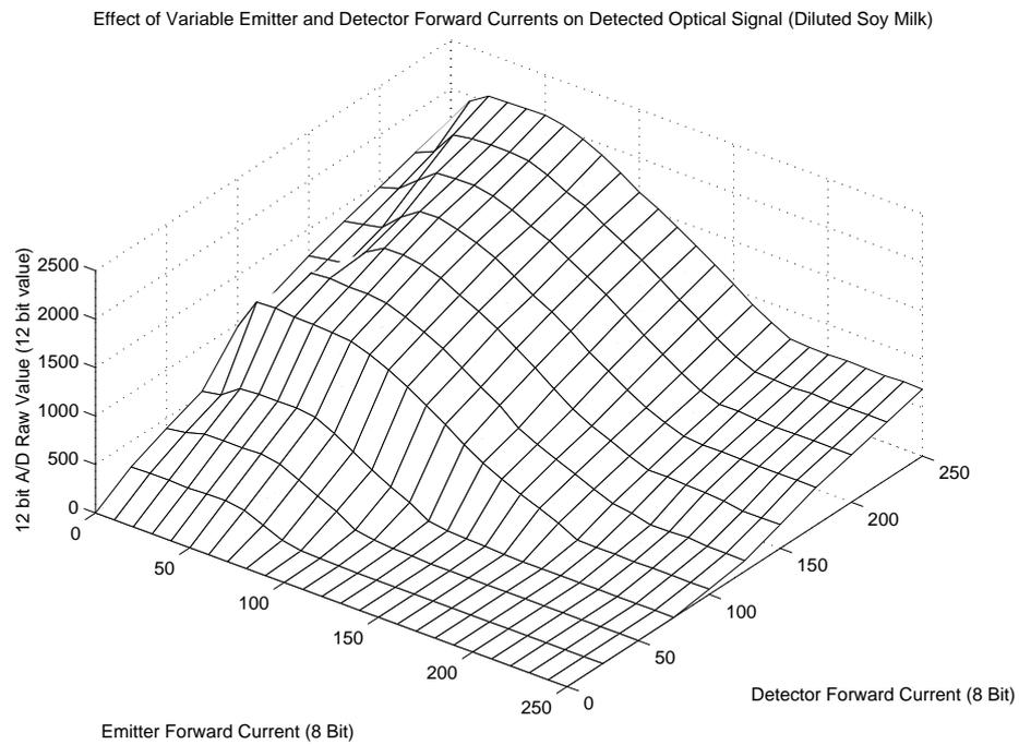
(a) Diluted soy based milk (simulating medium  $CaCO_3$  precipitation).
