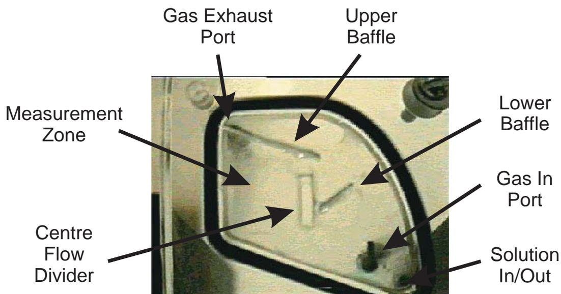
Figure 4.12: The empty ‘teardrop’ cell with two plastic baffles. Visible is the cell void, the center flow divider, and the three ports for the combined indicator chemical in/out (bottom), the sample gas in (towards the center), and sample gas out (top).
