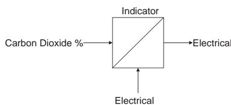
Figure 2.14: The overall form of the transduction necessary for the wet chemical analysis of  $CO_2$ .
