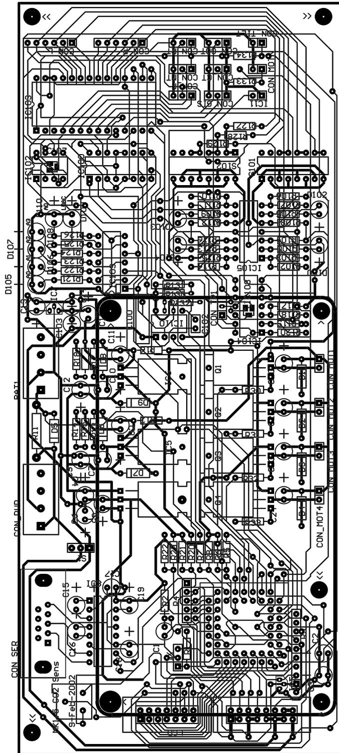
Figure A.27: Mk.II microcontroller board PCB.
