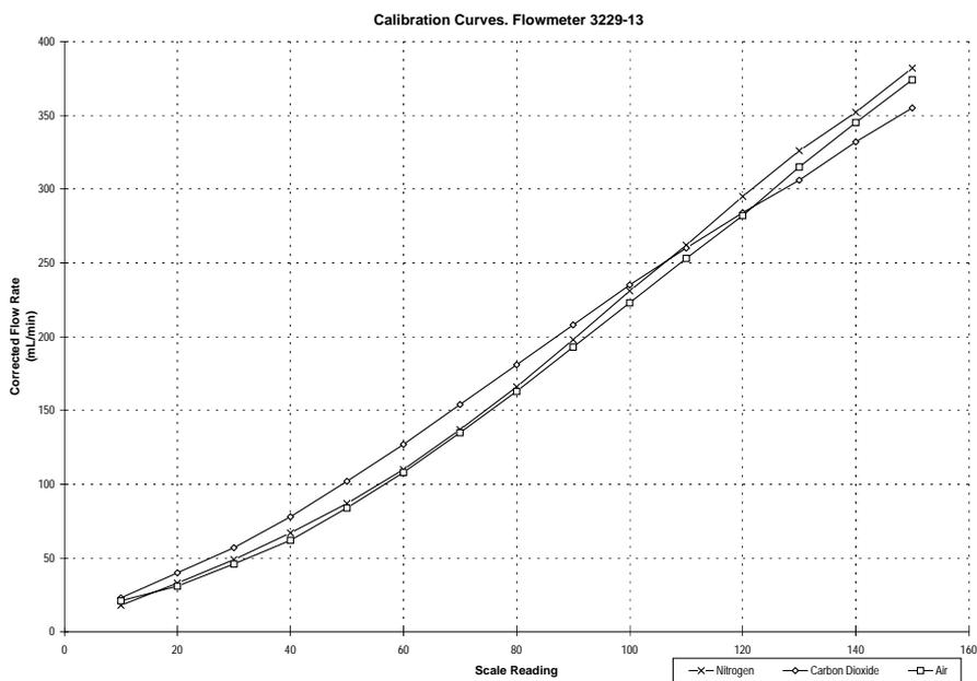
Figure F.4: 3229-13 flowmeter calibration curves for  $N_2$ ,  $CO_2$  and dry air.
