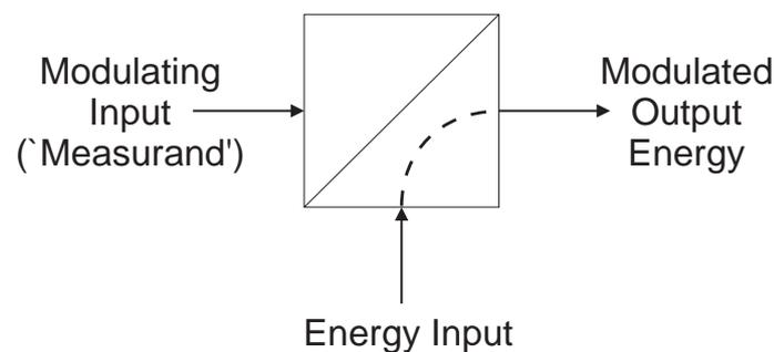
Figure 2.1: The generic representation for a general measurement transducer.
