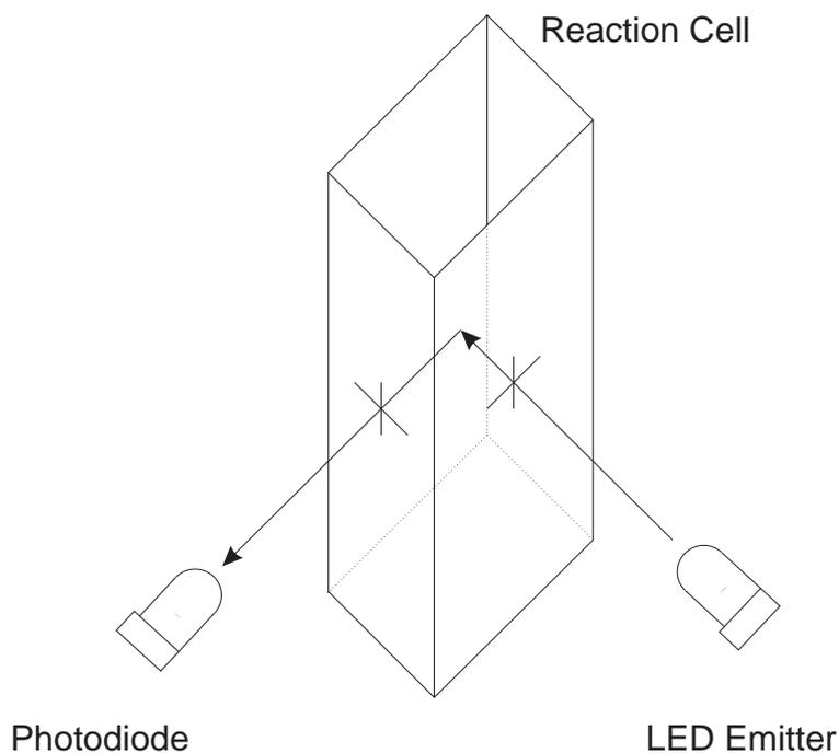
Figure 5.6: Example geometry of an off-axis optical sensor suitable for measurement of precipitate produced within a reaction cell. The emitter and detector alignment are rotated by  $90^\circ$  with the detector measuring optical scatter instead of transmissive attenuation.
