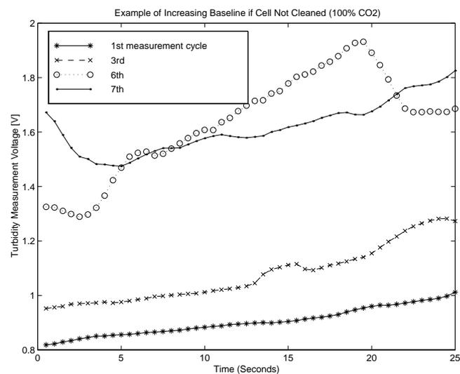
(b) Results from a sequence of turbidity measurements (at 100%  $CO_2$ ), neglecting to clean inbetween measurements. Baseline drift is shown for each subsequent turbidity measurement.
