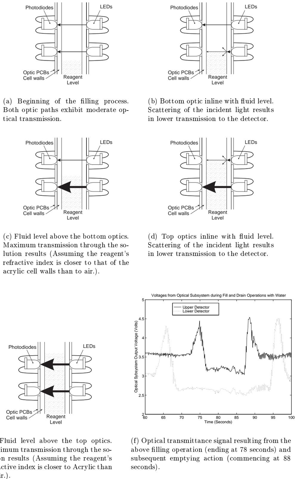
Figure 6.6: Example of the 'automated filling process' of the chemical reaction cell utilising information from the turbidity measurement optics.
