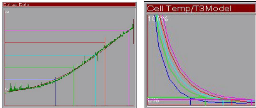
(a) Optical data, threshold points and times to each threshold. The horizontal axis shows time in seconds, whilst the vertical axis shows the arbitrary optical data values (A/D bits).
