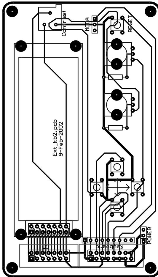
Figure A.29: Keyboard and display board PCB.
