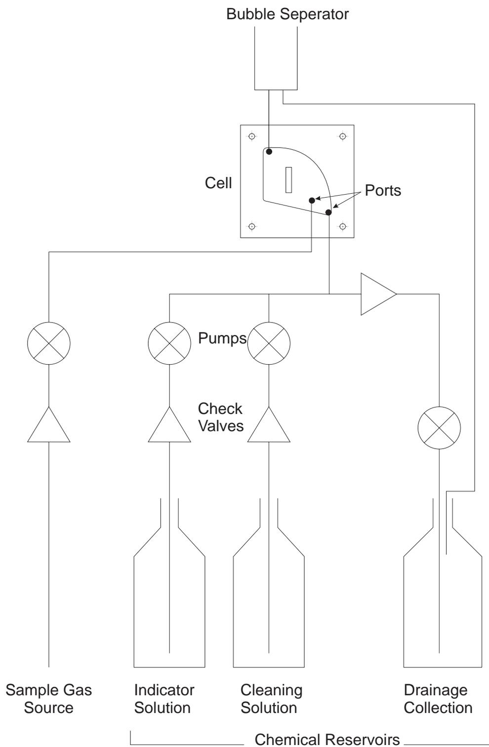
Figure 6.7: Interconnection scheme used for the Mk.II prototype.
