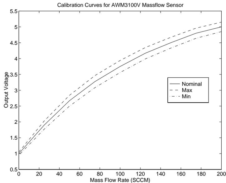
Figure 6.10: AWM3100V microbridge mass airflow sensor calibration curve.
