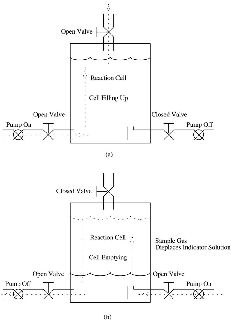
Figure E.1: The conceptual “constant volume” cell showing the cell void, the three ports, and valve/pump assemblies. (a) shows the cell during the filling operation, and (b) shows the cell during a measurement operation.
