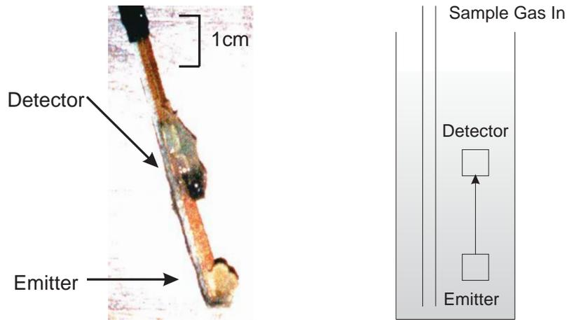
(a) A photograph of the sensor. (b) The measurement orientation.
