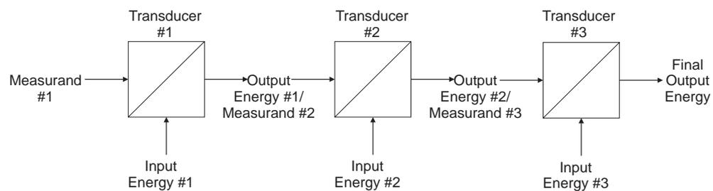
Figure 2.4: An example of a multi-stage transducer.
