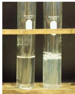
(b) Beginning of the bubbling process. The reaction chamber is starting to show signs of  $CaCO_3$  precipitation (after approx 12 seconds).
