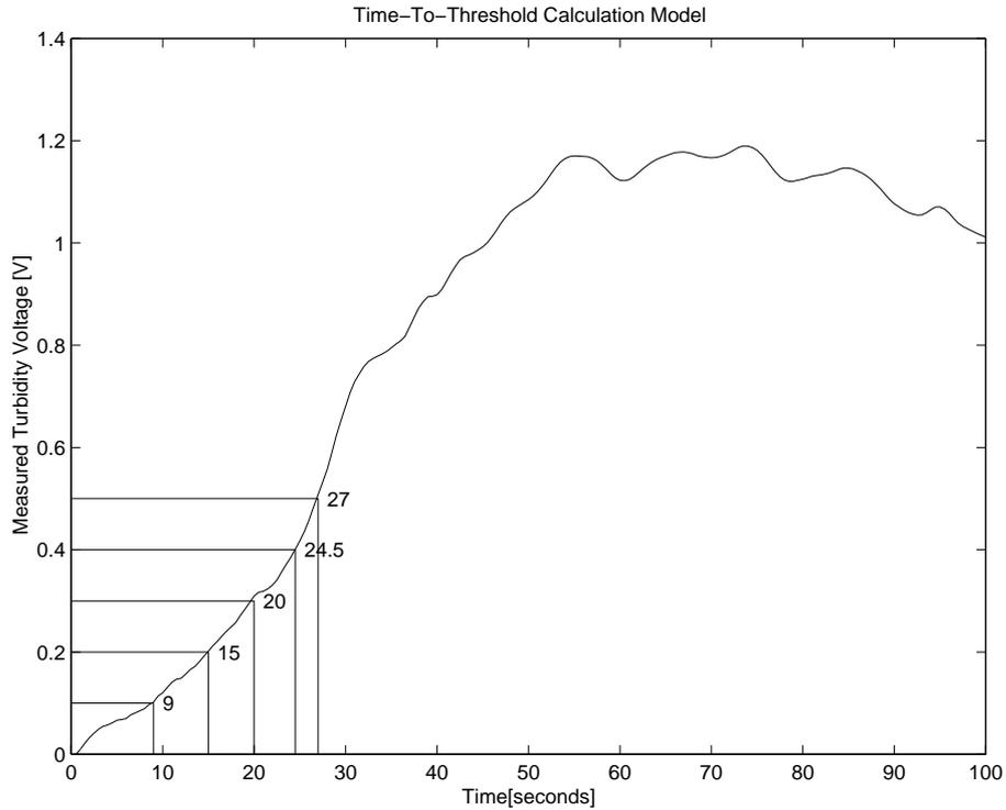
Figure 7.6: Example of a turbidity measurement from the Mk.II prototype for 100%  $CO_2$ .
