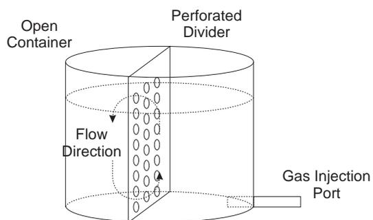
(a) Mechanical construction and expected flow directions.
