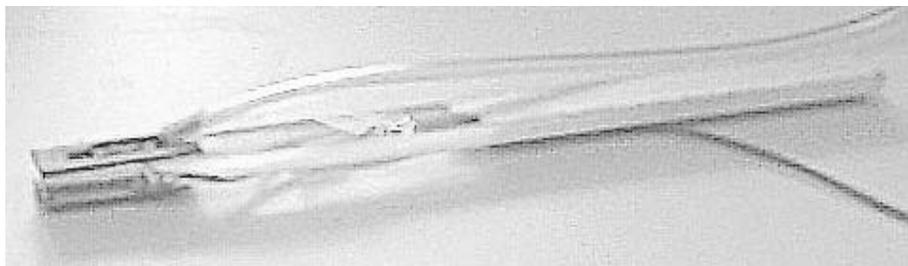
(a) Photograph of the capacitor sensor head comprising of the parallel plate capacitor, acrylic separator/handle and electrical wires.
