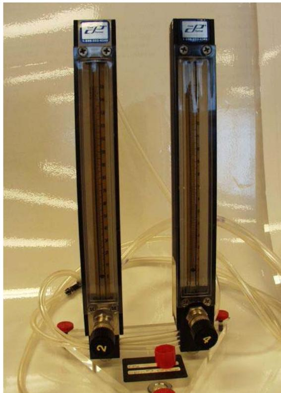
(b) The two flowmeters. The  $CO_2$  flowmeter is on the left with the  $N_2$  flowmeter on the right.
