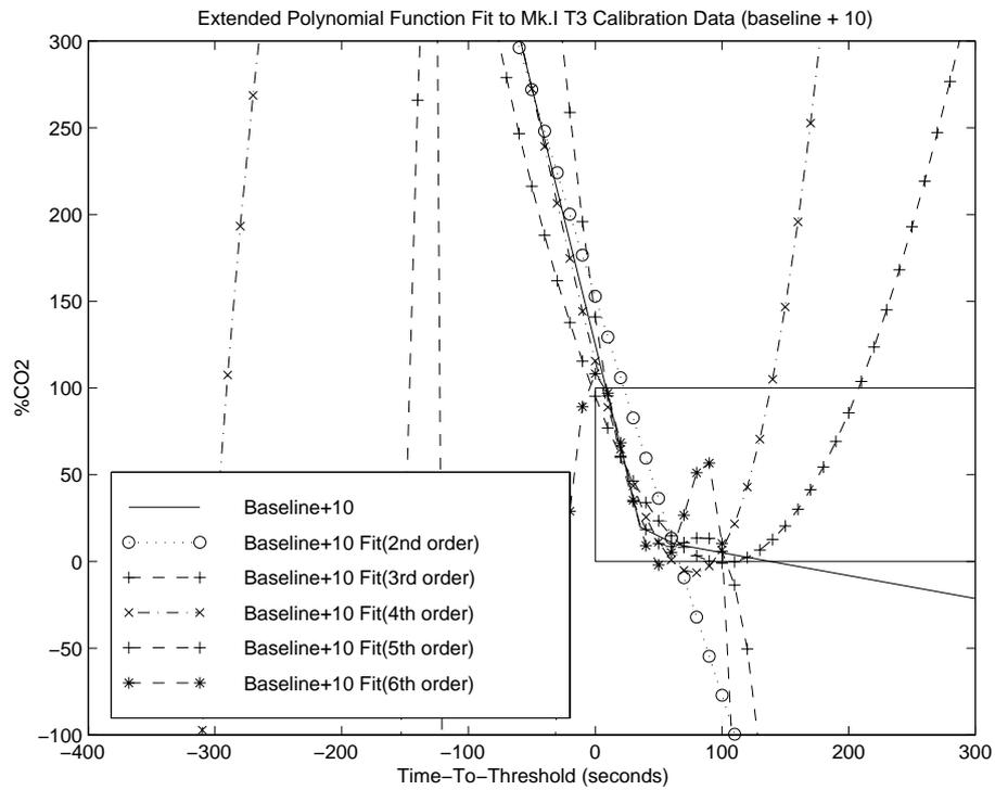
Figure B.5: Example polynomial fit using extended data for the ‘baseline + 10’ data using the MATLAB simulation package. The region of interest constrained by 0 to 100%  $CO_2$  is contained within the box.
