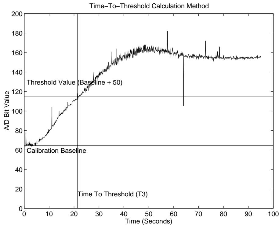
Figure 7.1: Example of a turbidity measurement from the Mk.I prototype for 100%  $CO_2$ . Spikes within the data were the result of noise generated by the gas pump motor during operation.
