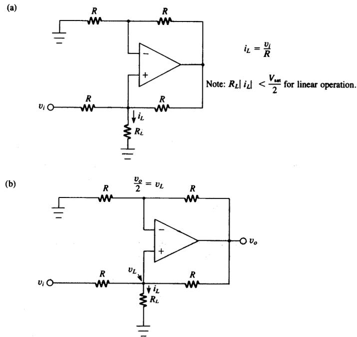
(a) Howland voltage controlled current source example (reproduced from Stanley, 1990, Figure 2-16, p73).
