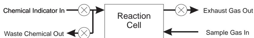
(b) Split input functions on one port with the upstream and one downstream pump (No sample gas contamination).
