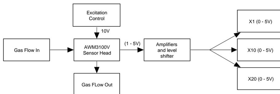
Figure 6.12: Signal flow diagram for the support electronics as part of the precision gas mass-flowmeter.
