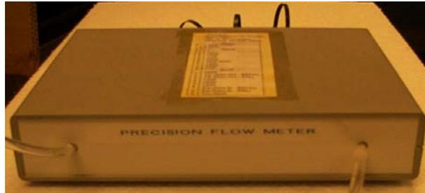
(a) Front view showing the gas interfacing ports.
