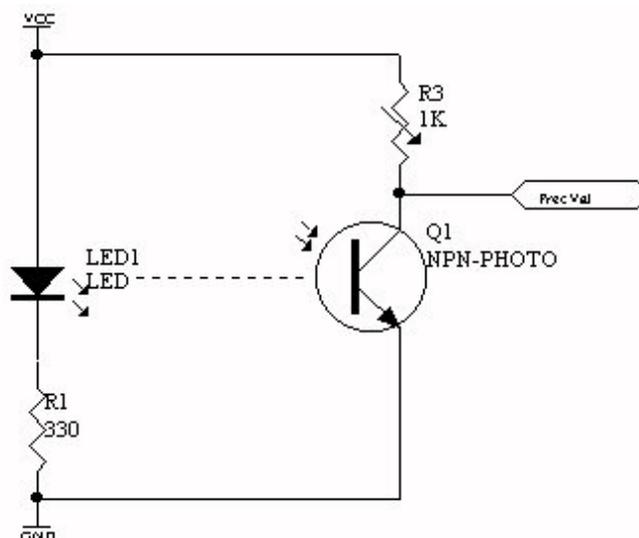
Figure 5.10: Mk.I current drive schematic for the LED emitter and Photodiode detector pair. (Two such emitter/photodiode pairs were installed on the reaction cell - Figure 5.5(a)).
