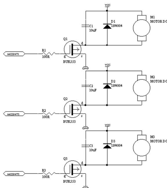
Figure 6.5: Pump motor control schematic showing the three FET switching devices.
