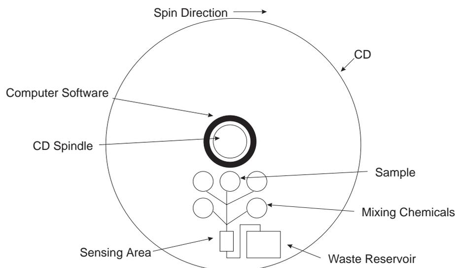
Figure 11.3: Example of a wet chemical sensor on a compact disc (CD) structure, conceptual only (after Madou, 2000). Variations in the disks spin speed controls the valves at the base of each chemical reservoir whilst centrifugal force provides the pumping action. It is possible to have integrated software on the CD providing instrumentation capabilities to a standard personal computers CDROM drive, with the drives laser providing optical measurement capability of the reagents.
