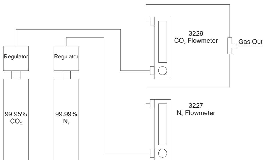
Figure F.1: Connection diagram for the constructed gas laboratory.
