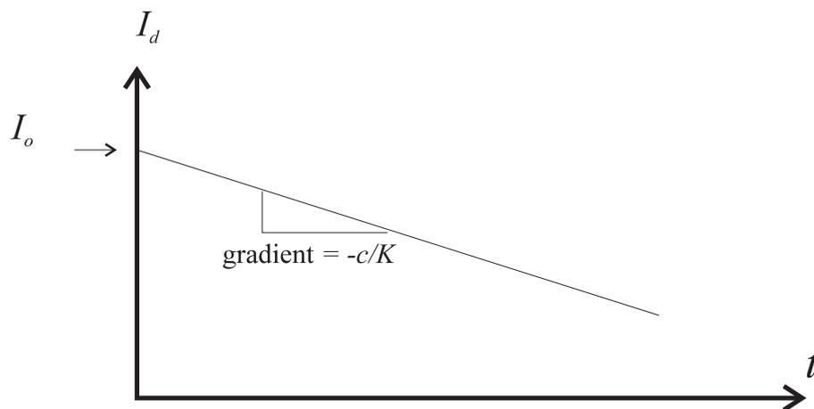
Figure 3.6: Characteristics of  $I_d$  over time  $t$ . Shown is the dependency on the  $CO_2$  concentration and the sensitivity coefficient  $K$  for the final measurement system.
