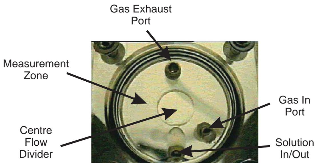
Figure 4.16: The empty circular cell. Visible is the cell void, the center flow divider, and the three ports for the combined indicator chemical in/out (bottom), the sample gas in (towards the left), and sample gas out (top).
