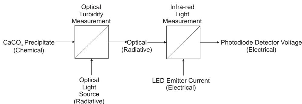
Figure 5.1: Transduction necessary for optical turbidity measurement.
