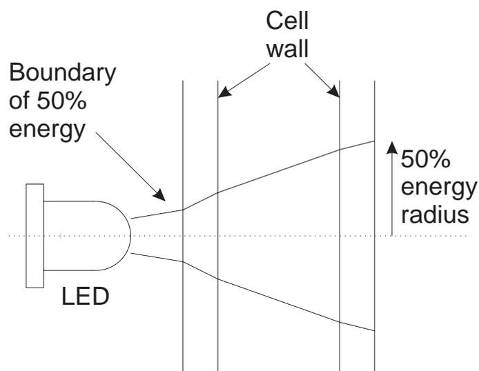
Figure 5.9: Demonstration of the refractive effects on the 50% energy radius through the cell.
