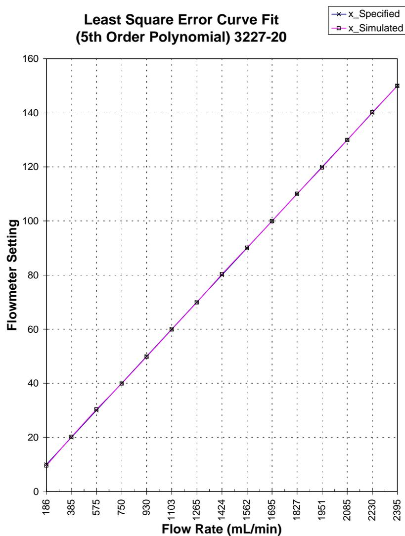
Figure F.5: 3227-20 flowmeter calibration comparison between supplied calibration information and the theoretical calibration model.
