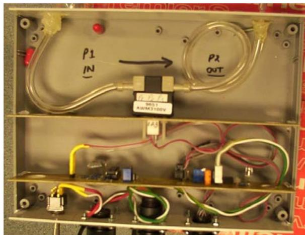
(c) Inside view of the electronics. Shown in the center is the Honeywell AWM3100V sensor.
