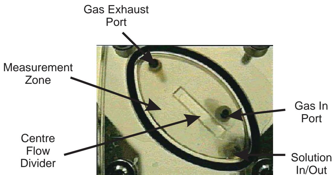
Figure 4.18: The empty oval cell. Visible is the cell void, the center flow divider, and the three ports for the combined indicator chemical in/out, the sample gas in, and sample gas out.
