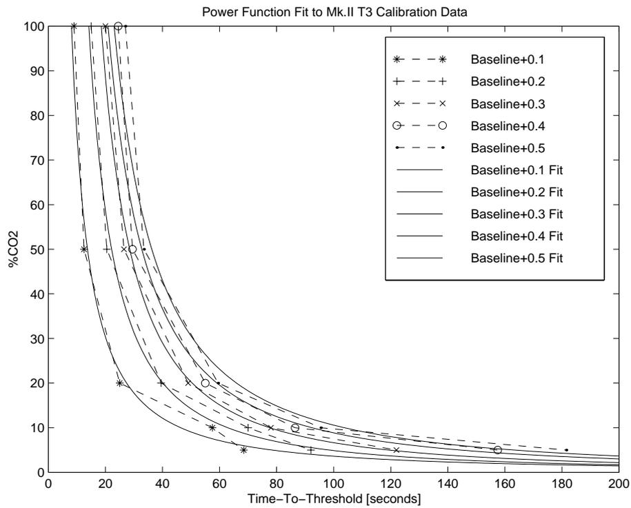
Figure B.10: Power fit curves to measured “T3” threshold times.
