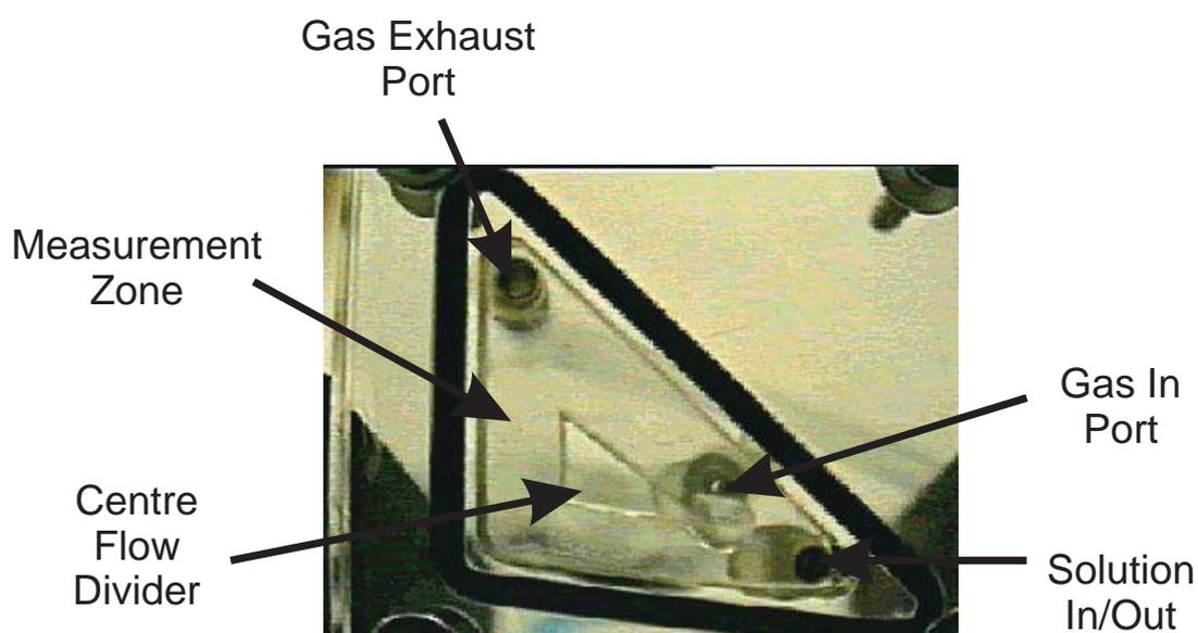
Figure 4.20: The empty triangular cell. Visible is the cell void, the center flow divider, and the three ports for the combined indicator chemical in/out, the sample gas in, and sample gas out.
