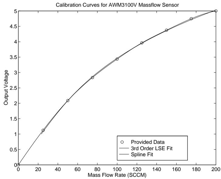
Figure 6.11: Two models used to interpolate the AWM3100V manufacturer provided calibration data.
