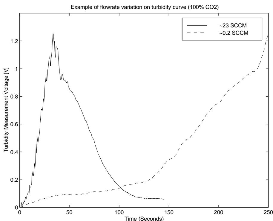
Figure 10.19: An example of how flowrate affects the characteristic turbidity curve.
