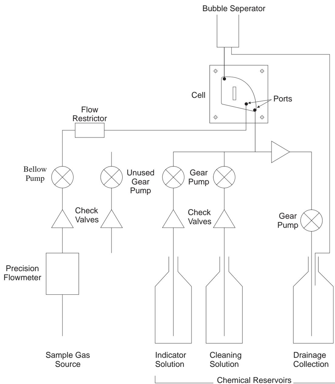
Figure 6.14: Final connection scheme used for the Mk.II prototype. Additional components include the bellow pump, precision flowmeter, and flow restrictor.
