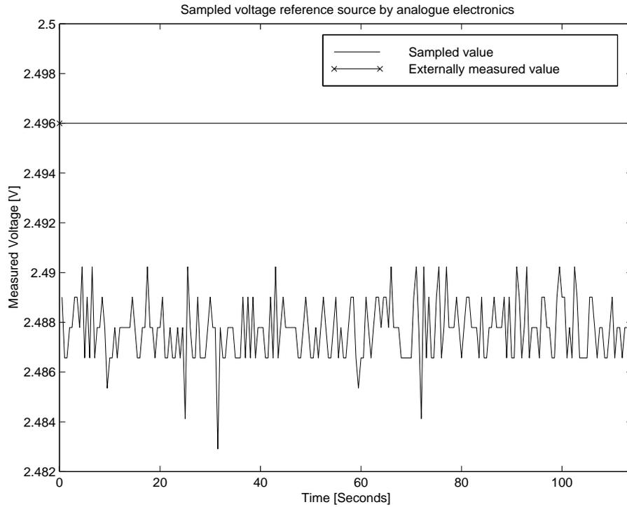
Figure 10.7: A/D converted voltage compared with the voltage of the onboard 2.5V voltage reference source.
