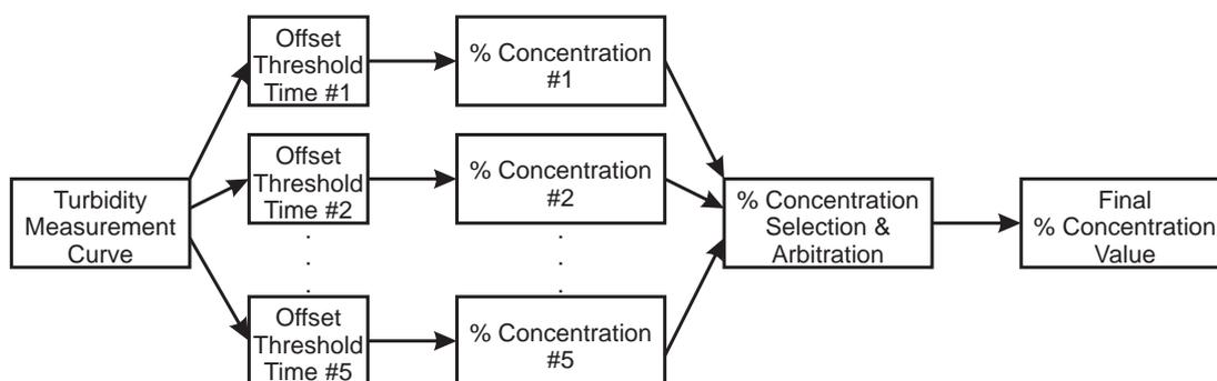
Figure 7.2: The signal flow for the “Time To Threshold” Model.
