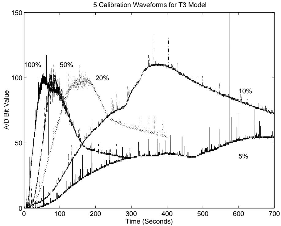
Figure 7.3: The five calibration turbidity waveforms used to generate the ‘Mk.I’ model. Spikes within the data were the result of noise generated by the gas pump motor during operation.
