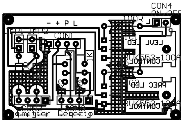
Figure A.19: Optics control sub-system PCB (v2.0).
