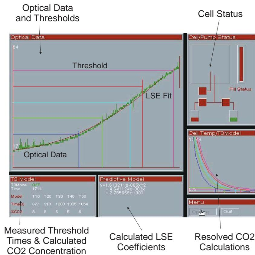
Figure 9.3: Screen capture of the CO2\_SCS software during the processing of some optical data (100% CO<sub>2</sub>). (A clearer presentation of the data of this figure is set out in Figure 9.4.)
