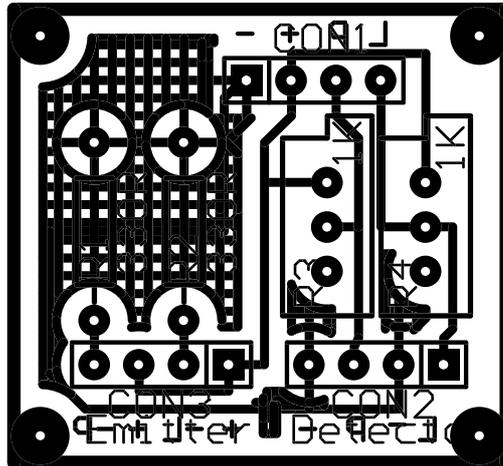
Figure A.18: Optics control sub-system PCB (v1.2).
