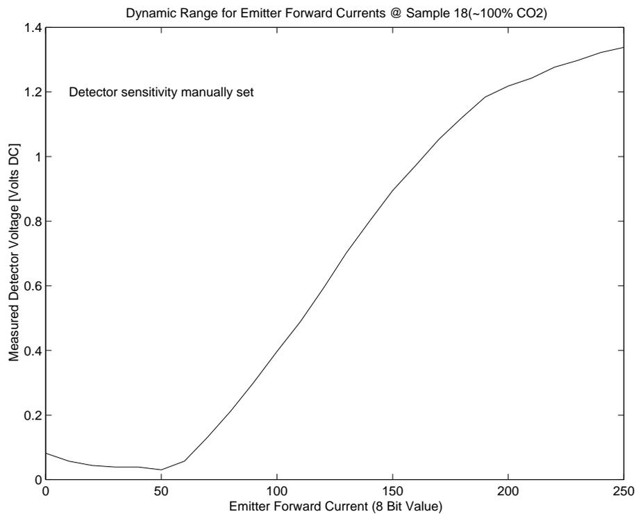
Figure 10.13: Dynamic range of the optics calculated at sample 18 (the peaks of the optical curves) using a baseline reference from the initially acquired optical data at sample 1.
