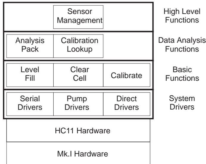
Figure 9.1: Structure of the firmware for the Mk.I Prototype.
