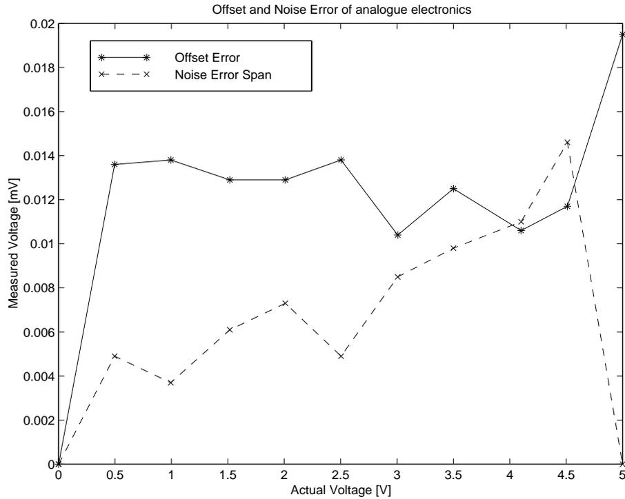
Figure 10.8: Full scale DC offset and noise span errors of the analogue electronics.
