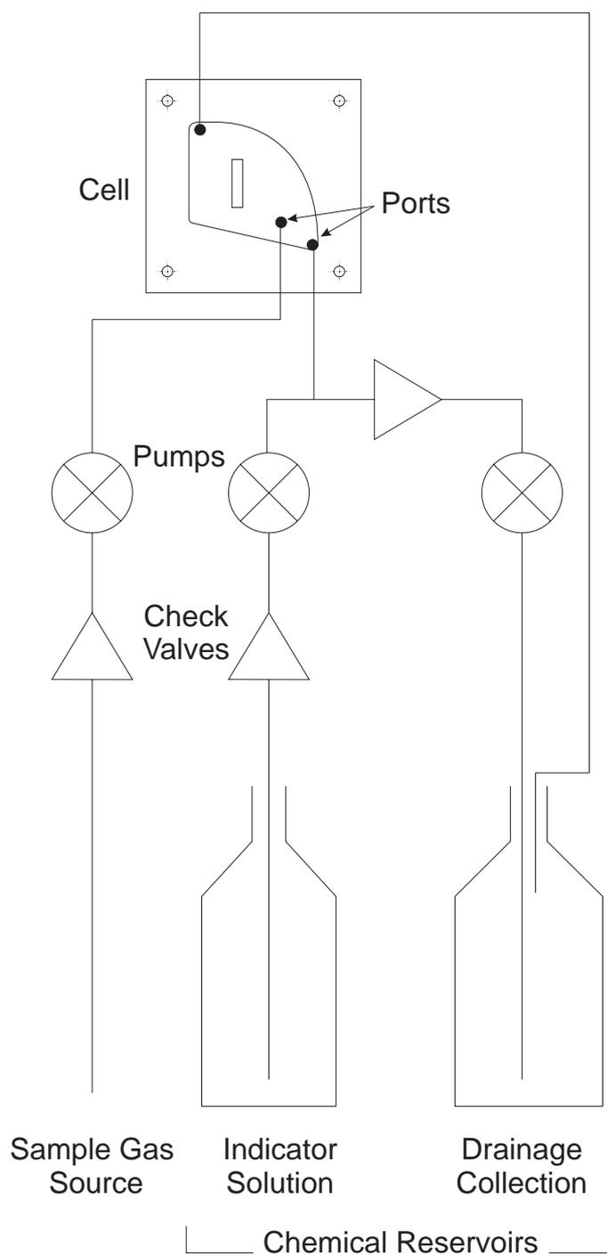
Figure 6.3: Connection scheme used for the Mk.I prototype. Three pumps (two for fluid control, and one for gas control) were connected to the cell using check valves, 'tee' pieces, and 4mm polyurethane tubing.
