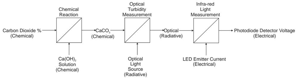
Figure 3.2: Transduction necessary for wet chemical analysis of  $CO_2$  (at each stage the measurement information energy regime is indicated in parenthesis).
