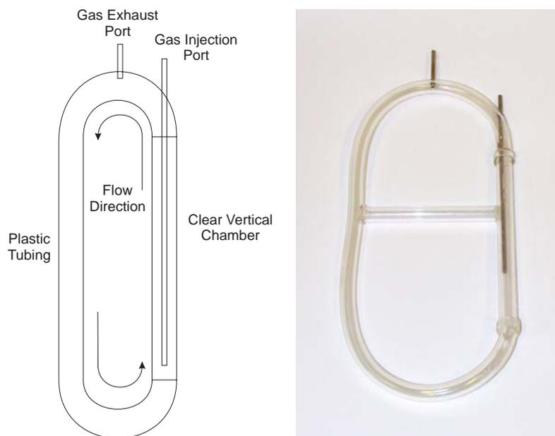
(a) Mechanical construction and expected flow directions.
