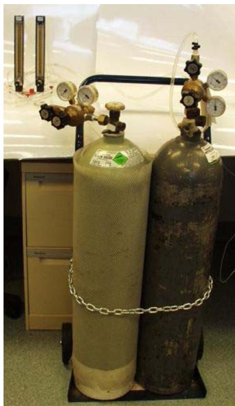
(a) Gas cylinders and flowmeters. The  $CO_2$  gas cylinder is on the left with the  $N_2$  gas cylinder on the right.
