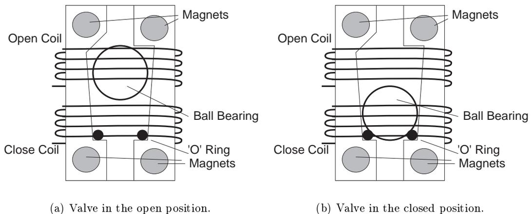
Figure E.2: Microcontroller selectable fluid check valves. Shown are the magnet and coil assemblies as well as the ball bearing and ‘O’ ring seal.
