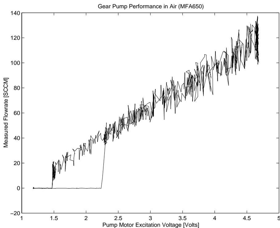
Figure 10.5: Raw data of unloaded flowrate performance of the MFA 650 gear pump for gas.
