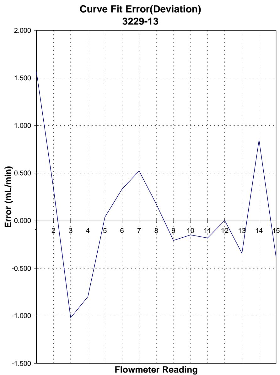
Figure F.8: 3229-13 flowmeter error between supplied calibration information and the theoretical calibration model.
