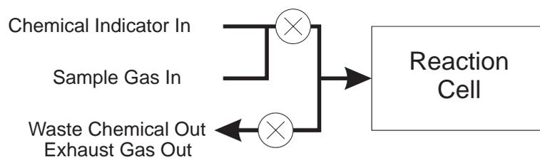
(b) Single port configuration with combined chemical indicator and sample gas input functions through a single pump.
