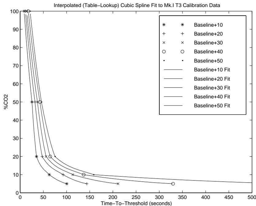
Figure B.8: Interpolated cubic spline fit curves to measured “T3” threshold times.
