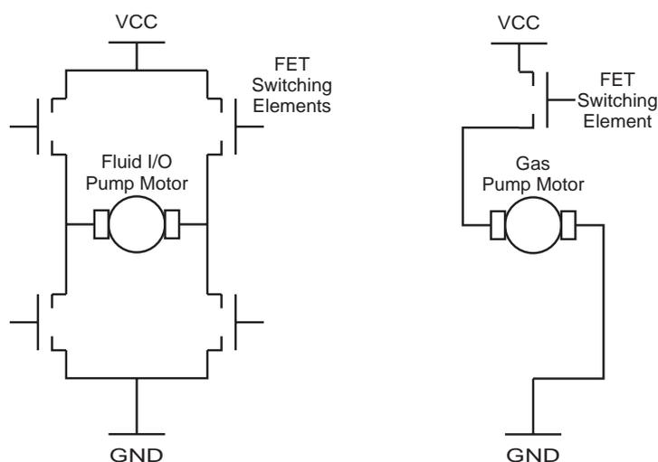
(a) ‘H’ bridge configuration required to control the flow direction of a bi-directional pump.
