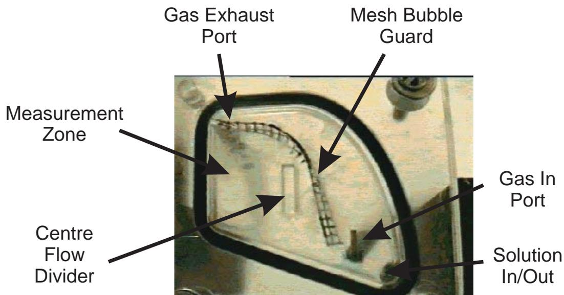
Figure 4.14: The empty 'teardrop' cell with plastic mesh bubble guard. Visible is the cell void, the center flow divider, and the three ports for the combined indicator chemical in/out (right), the sample gas in (towards the left), and sample gas out (top).
