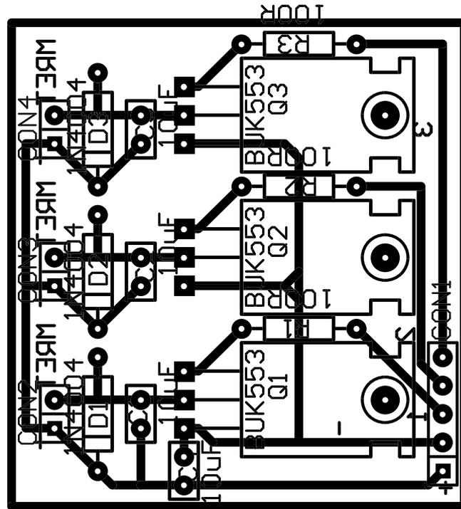
Figure A.15: Motor control sub-system PCB (v2.0).
