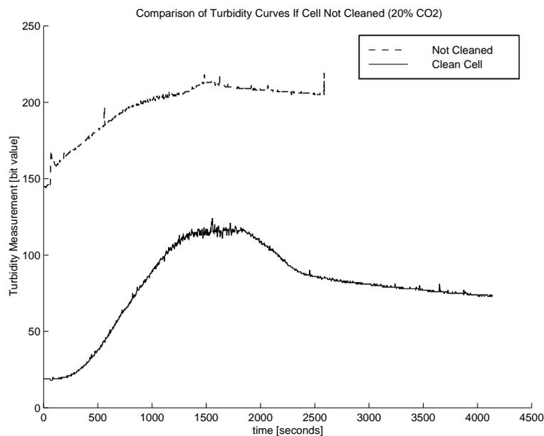
Figure 10.4: Turbidity measurement of 20%  $CO_2$  immediately after the cell was cleaned and then again after several measurements when cleaning was neglected. Shown is the increase in turbidity and the decrease in dynamic range.
