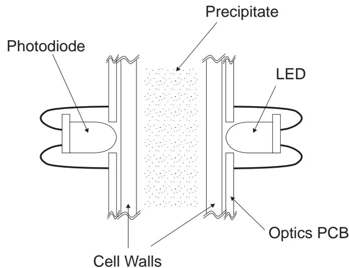
Figure 5.7: Mounting diagram for the optical components being soldered to the alignment PCB. Shown is the method to mount the LEDs and photodiodes to the PCB as well as the required optical-pair alignment desired.
