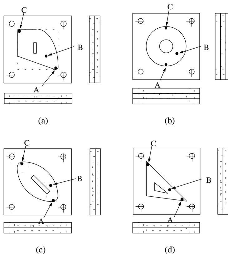
Figure 4.8: The cells, (a) 'teardrop', (b) 'circular', (c) 'oval', and (d) 'triangular'. In each case A is the chemical indicator inlet/outlet port, B is the sample gas inlet port, and C is the sample gas output port(exhaust).
