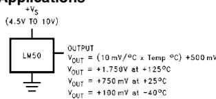
FIGURE 1. Full-Range Centigrade Temperature Sensor ( $-40^{\circ}\text{C}$  to  $+125^{\circ}\text{C}$ )
