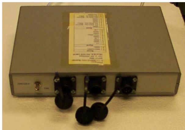
(b) Rear view showing the power switch and electronic interface connectors.
