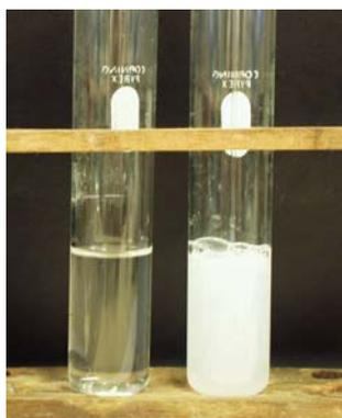
(c) Bubbling process underway. The reaction chamber is continuing to produce  $CaCO_3$  precipitation (after approx 20 seconds).
