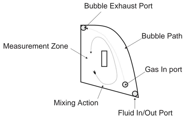
Figure 4.9: Intended fluid flow within the 'teardrop' cell.
