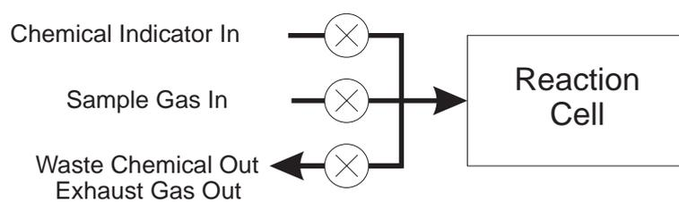
(a) Single port configuration with three separate pumps.
