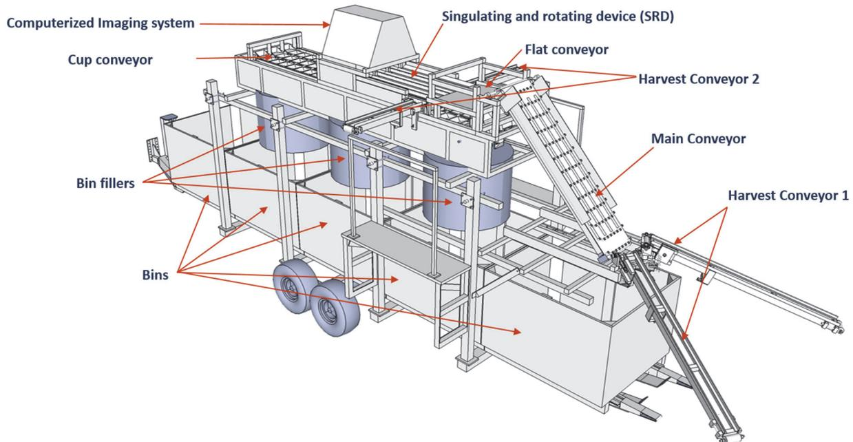
Figure 1. Diagram of the apple harvest and in-field sorting prototype.
