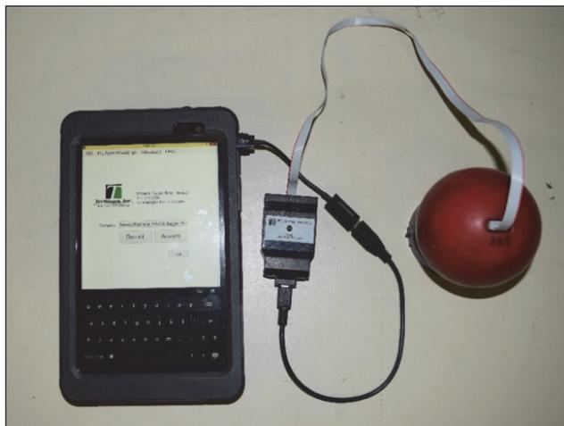
Figure 6. Impact recording device (IRD) connected to the communication interface with a USB communication cable.
