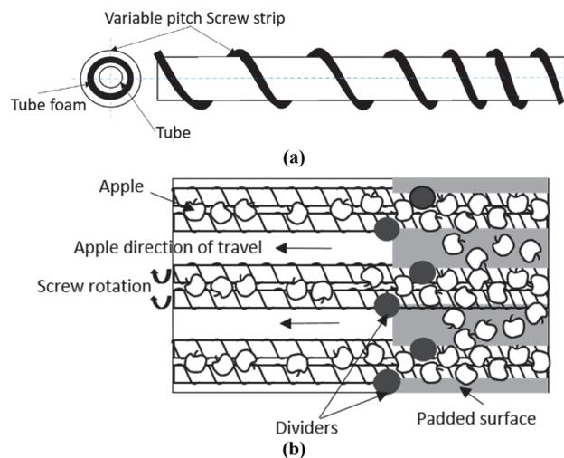
Figure 3. Schematic diagram of (a) single screw and (b) the multi-screw conveyor for singulating and rotating apples.
