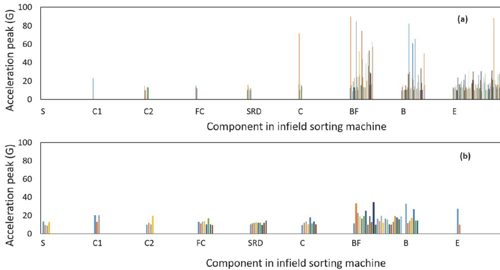
Figure 8. Total impacts occurring at different components in the apple harvest and in-field sorting machine during ten runs of the impact recording device (IRD): (a) empty bin and (b) partially filled bin (S = start, C1 = harvest conveyors, C2 = main conveyor, FC = flat conveyor, SRD = singulating and rotating device, C = cup conveyor, BF = bin filler, B = bin, and E = end).
