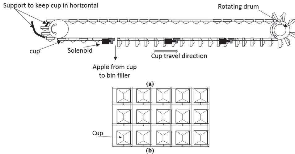
Figure 4. (a) Schematic diagram of the cup conveyor and (b) cup arrangement in three lanes.
