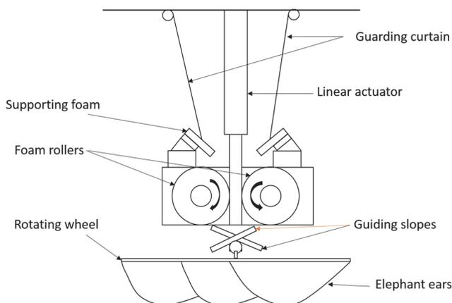
Figure 5. Schematic diagram of the bin filler.
