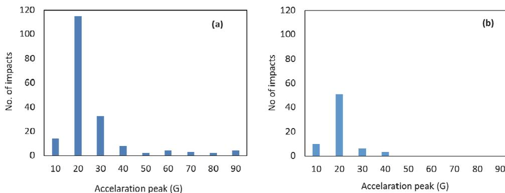
Figure 7. Histogram of impacts recorded by the impact recording device (IRD) during ten runs for different levels of peak acceleration ( $G$ ) for (a) empty bin and (b) partially filled bin.
