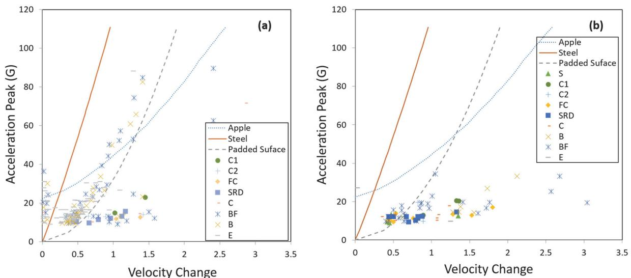
Figure 9. Peak acceleration ( $G$ ) versus velocity change for (a) empty bin and (b) partially filled bin (S = start, C1 = harvest conveyors, C2 = main conveyor, FC = flat conveyor, SRD = singulating and rotating device, C = cup conveyor, BF = bin filler, = bin, and E = end). The dotted, solid, and dashed lines are the bruise damage reference lines for apple, steel, and padded surface, respectively.
