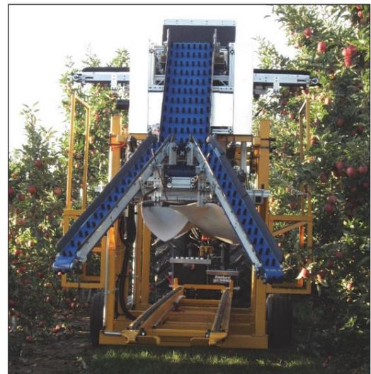
Figure 2. Field testing of the apple harvest and in-field sorting prototype during the 2013 harvest season.
