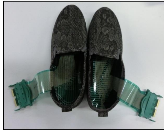
Figure 3. The in-shoe pressure system (Pressure sensor).
