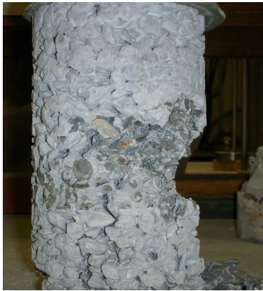
Figure 10. Failure due to non-uniform compaction
