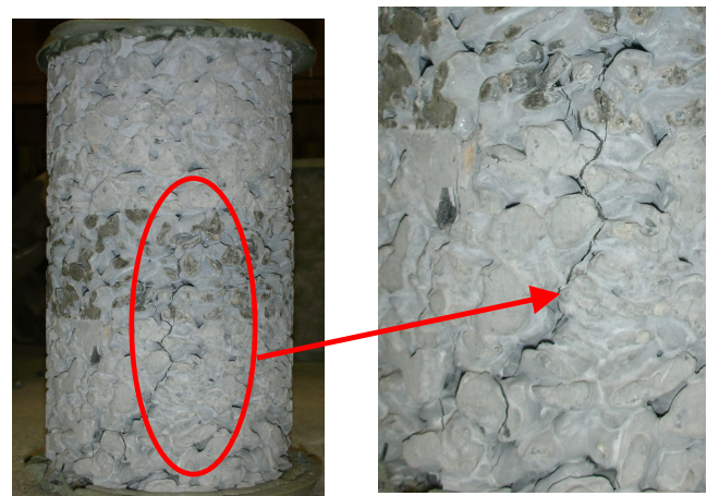
Figure 9. Type 1 failure (polymer mix)
