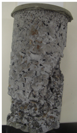
Figure 11. Failure patten for layered mix design
