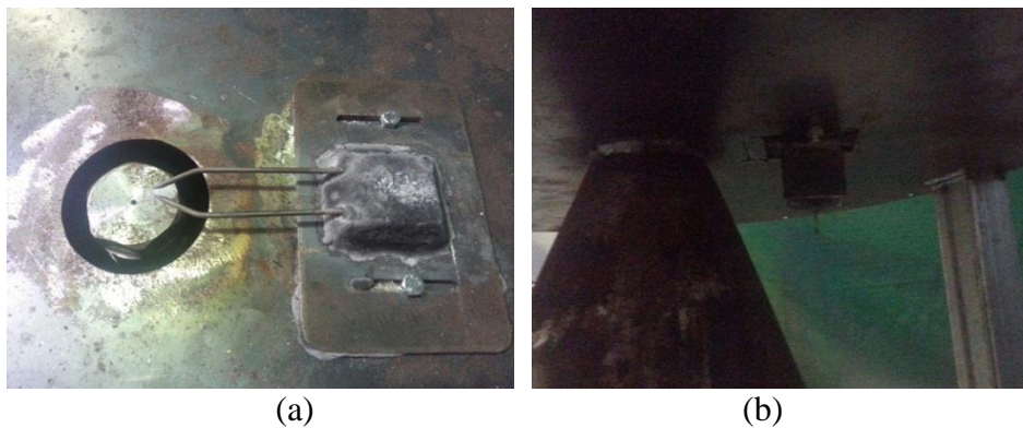
Figure 9. Ignition system (a) ignition lead top view (b) bottom view
