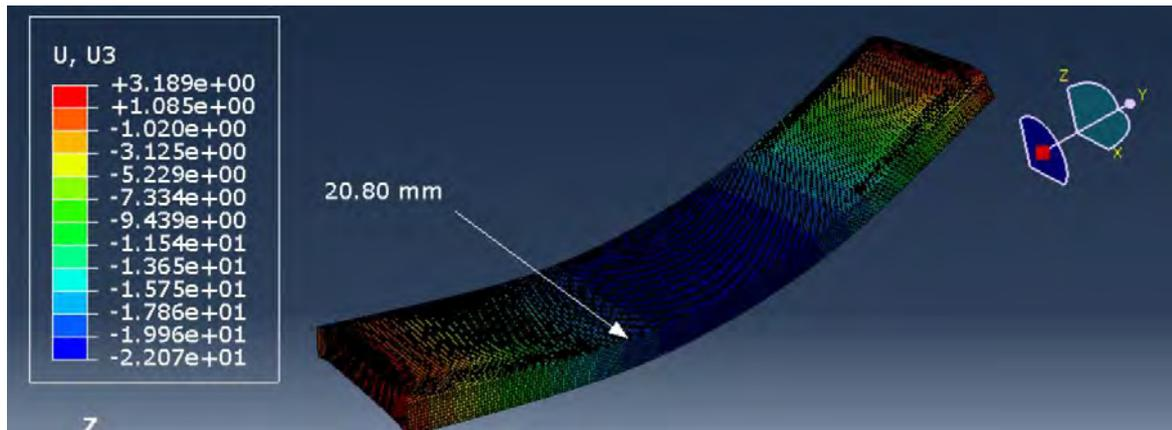
Figure 2: Deflection of SA4L at 125 kN load.
