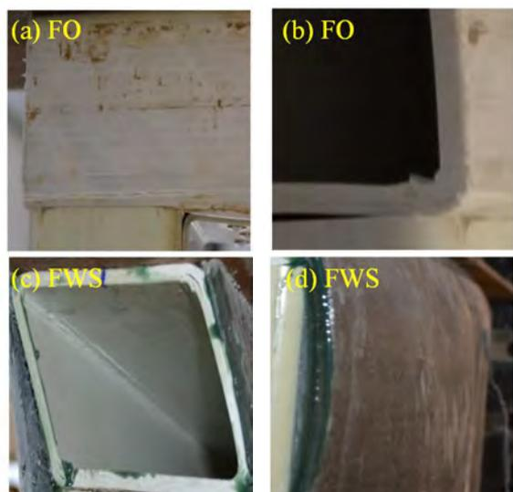
Fig.1. Failure modes of walls (a) Horizontal cracking (b) & (c) Junction failure (d) Sheet debonding
