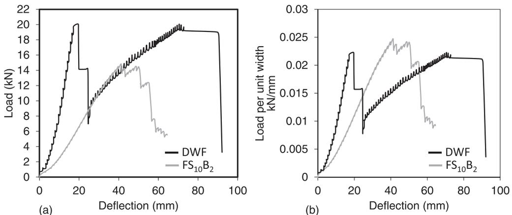
Fig. 11. DWF and FS<sub>10</sub>B<sub>2</sub> wall panels (a) Load deflection behaviour (b) Normalised load with panel width vs deflection of panel.
