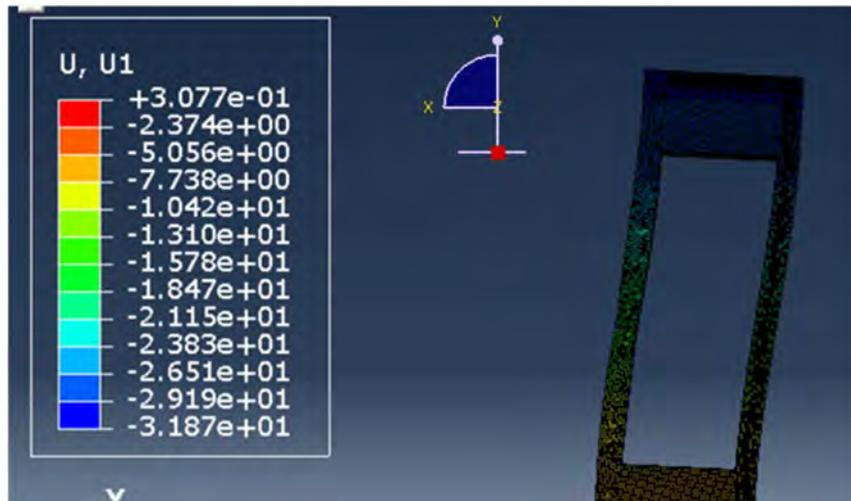
Figure 6: Lateral deformation at 5kN
