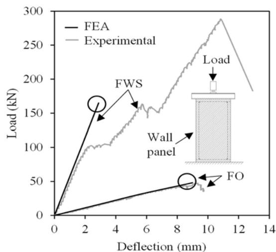
Fig.3. FEA and experimental load-deflection behavior of FO and FWS wall panels
