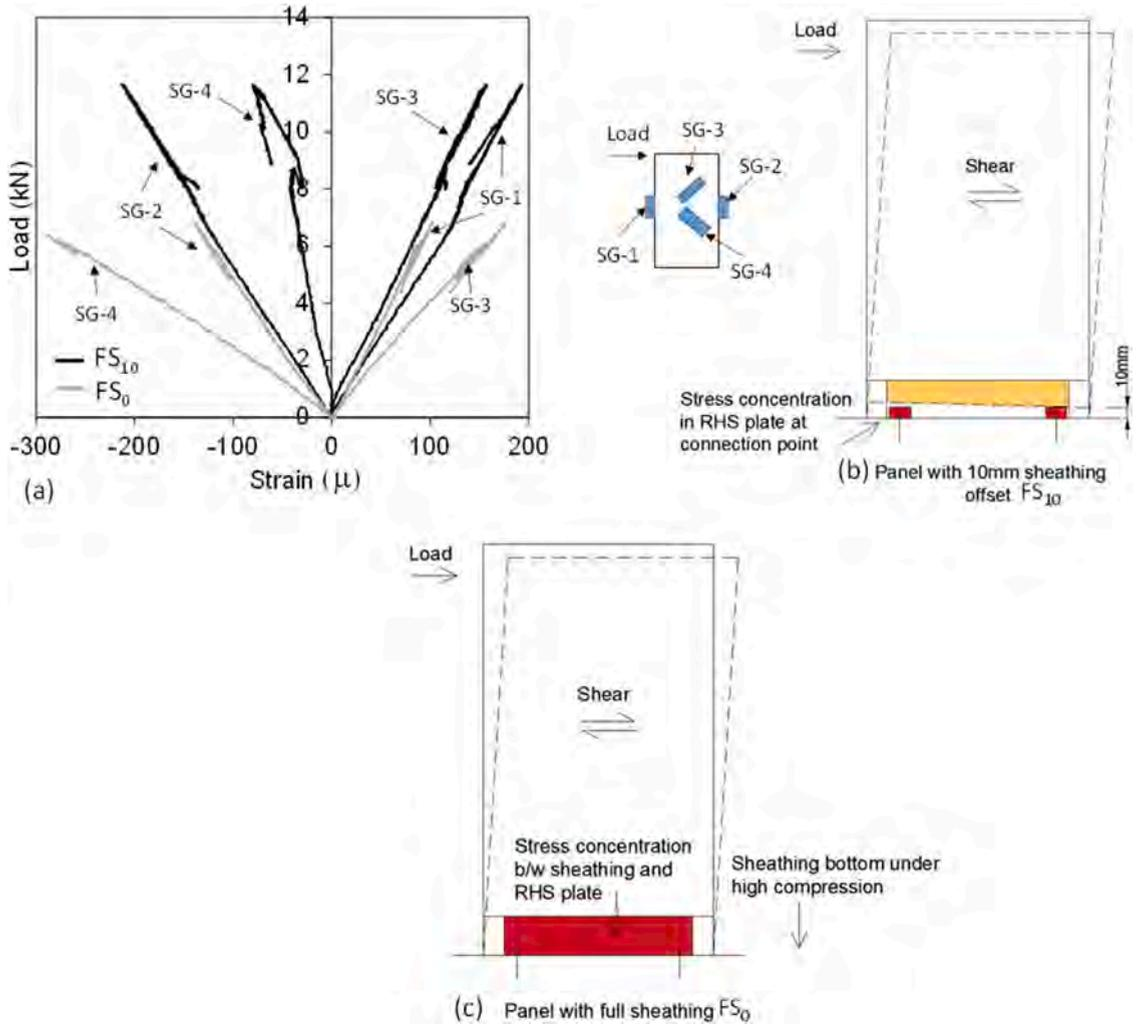
Fig. 6. (a) Load strain behaviour of sheathed wall panels  $FS_{10}$  and  $FS_0$  (b)  $FS_{10}$  failure mechanism (c)  $FS_0$  failure mechanism.
