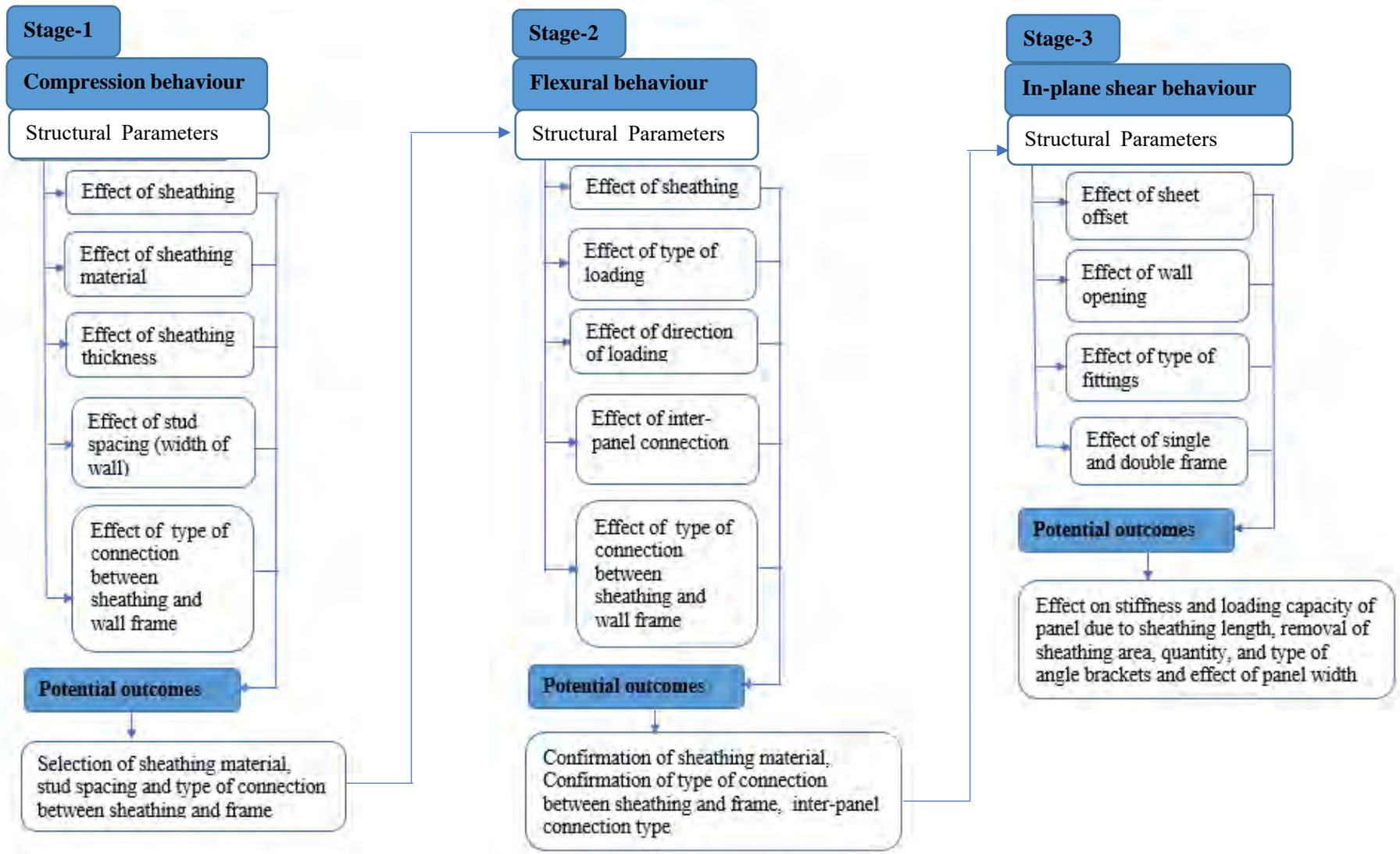
Figure 1: Critical parameter of wall panels under compression, flexural and in-plane shear load.
