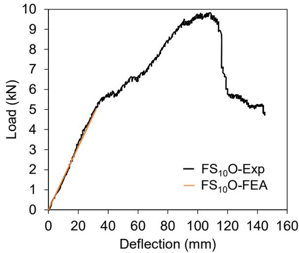
Figure 4: Load deflection behaviour of FS<sub>10</sub>O (with opening)
