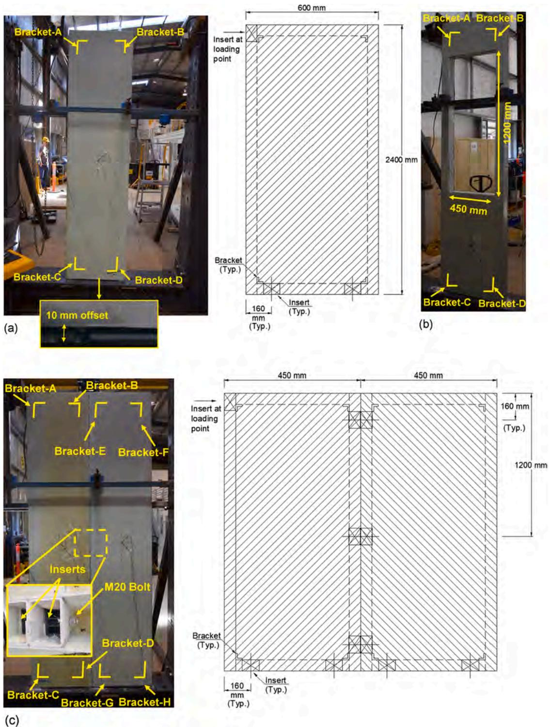
Fig. 1. (a) Single frame (b) Panel with opening (c) Double wall frame.
