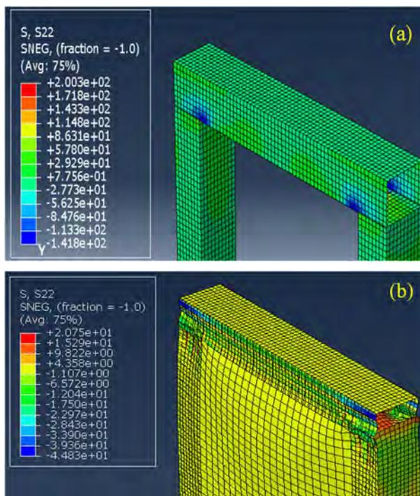
Fig.2. FEA longitudinal stress plots for panels (a) FO (b) FWS
