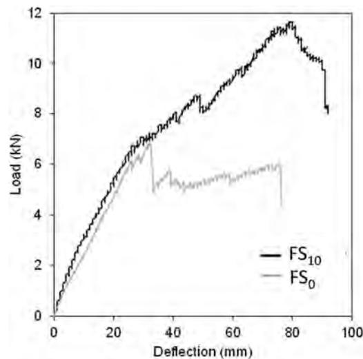
**Fig. 5.** Load deflection for sheathed wall panels FS<sub>10</sub> and FS<sub>0</sub>.
