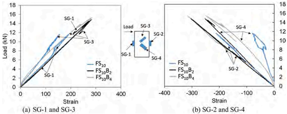
Fig. 10. Load strain behaviour of FS<sub>10</sub>, FS<sub>10</sub>B<sub>2</sub> and FS<sub>10</sub>B<sub>4</sub> wall panels.
