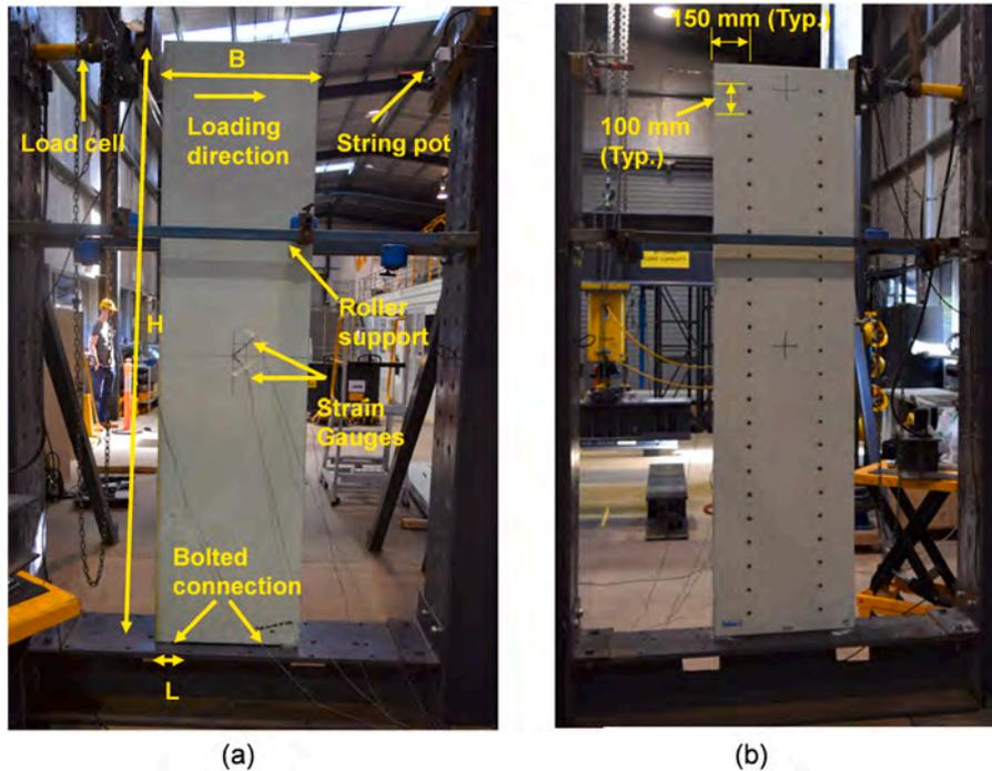
Fig. 3. (a) Test setup (b) Marking for DIC measurement.
