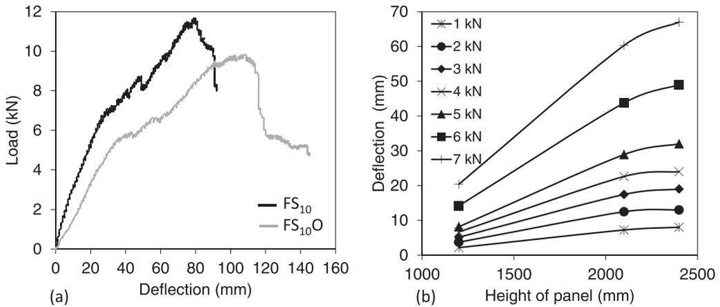
Fig. 7. (a) Load deflection behaviour of  $FS_{10}$  and  $FS_{0O}$  wall panels (b) DIC lateral displacement around window opening.
