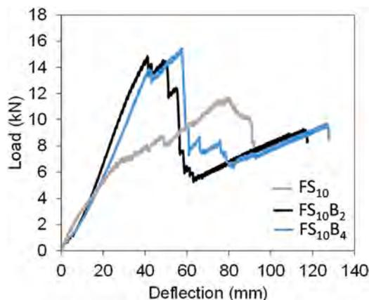
Fig. 9. Load deflection behaviour of  $FS_{10}$ ,  $FS_{10}B_2$  and  $FS_{10}B_4$  wall panels.
