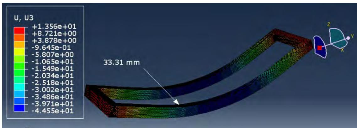
Figure 3: Deflection in SF4L at 79 kN load.
