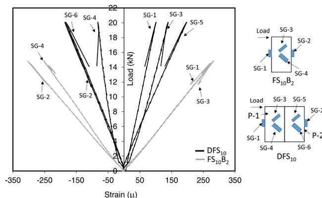
Fig. 12. Load strain behaviour of DFS<sub>10</sub> and FS<sub>10</sub>B<sub>2</sub> wall panels.
