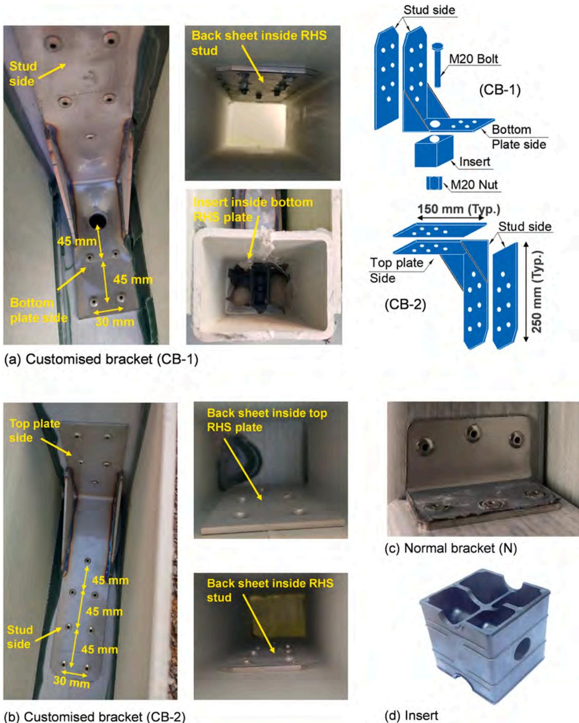
Fig. 2. (a), (b) and (c) Details of angle brackets used in composite wall panels (d) Anti-crush insert [43].
