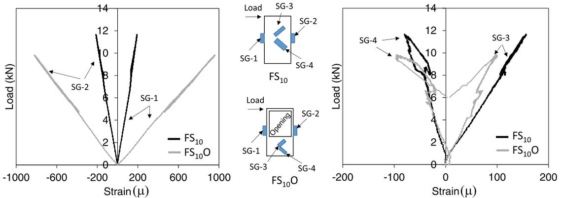
Fig. 8. Load strain behaviour of FS<sub>10</sub> and FS<sub>10</sub>O wall panels.
