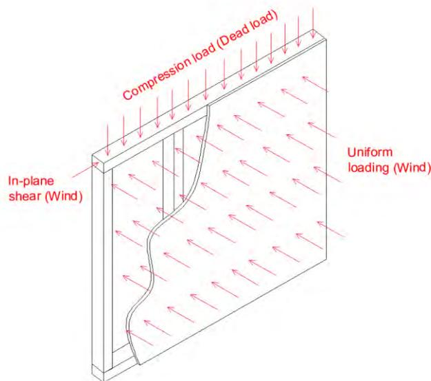
Figure 6: Typical loads acting on load bearing wall system
