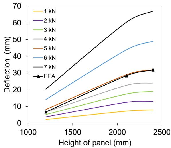
Figure 5: Lateral deformation along the height of FS<sub>10</sub>O panel from DIC and FE analysis
