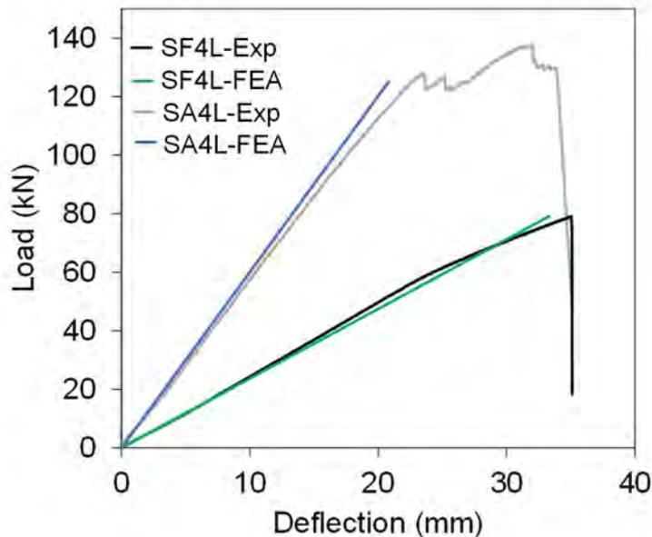
Figure 1: Load deflection behaviour of SF4L (without sheathing) and SA4L (with GFRP sheet) panels
