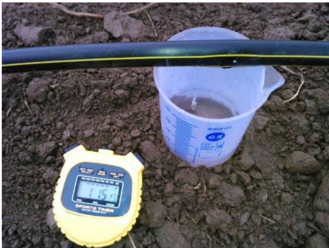
Figure 4.13: Water flow measurement using catch can and stopwatch.
