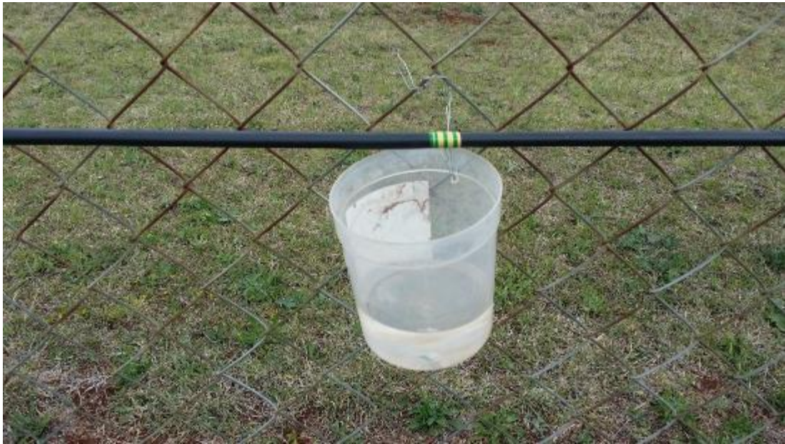
Figure 3.20: View of water dripping down from the emitter into the catch can.
