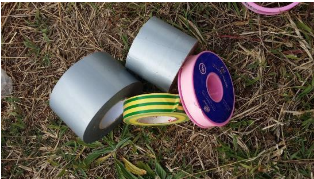
Figure 3.12: Duct tape used to block the emitters and to tie the dripline to the mesh fence.
