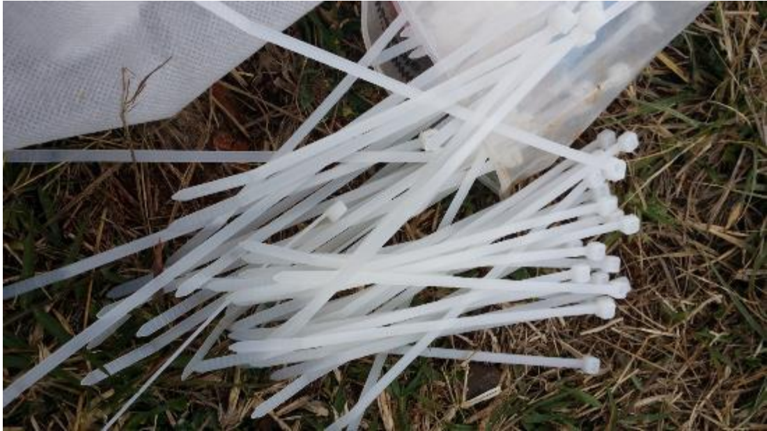
Figure 3.13: Zip ties used to attach the dripline to the fence at the field test site.
