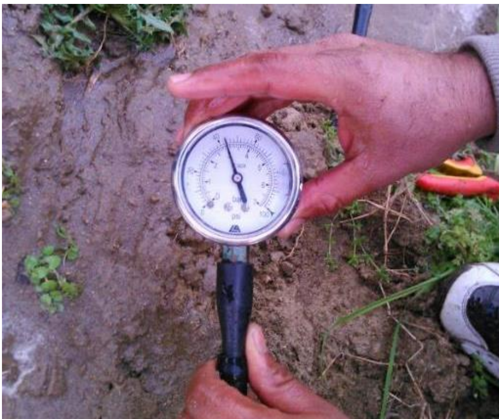
Figure 4.21: Measuring pressures at the end of dripline using pressure gauge.
