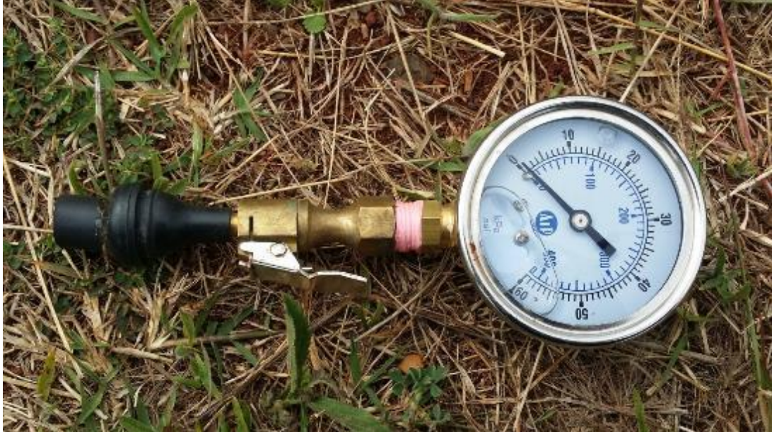
Figure 3.1: Specially designed handmade pressure gauge used to measure the individual emitter pressure at field test site.
