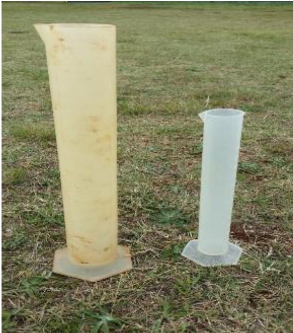
Figure 3.3: Measuring beakers used to measure the volume of water collected in each catch can.
