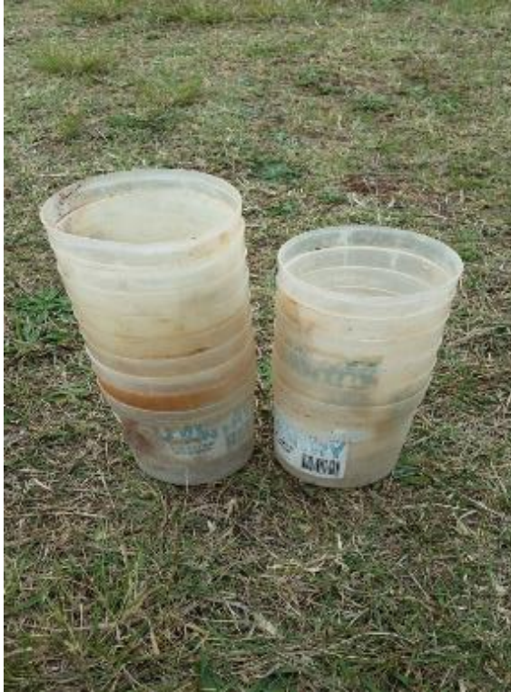
Figure 3.4: Catch cans used to measure the volume of water.
