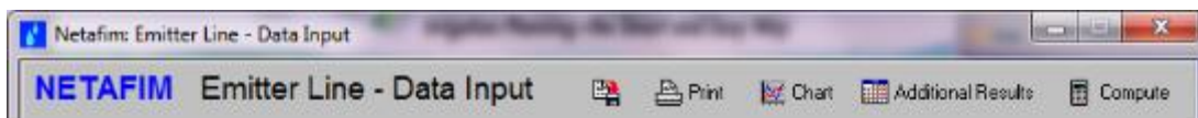
Figure 3.60: Emitter line data input bar showing save, print, chart, additional results and compute button.
