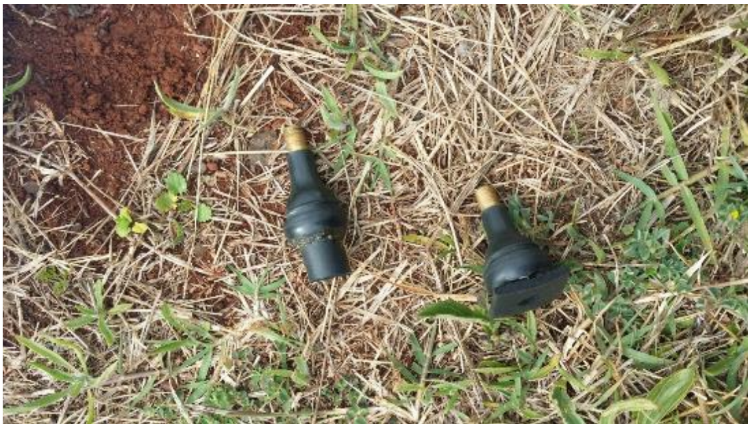
Figure 3.2: Handmade fittings connected to the pressure gauge to measure the individual emitter pressure.
