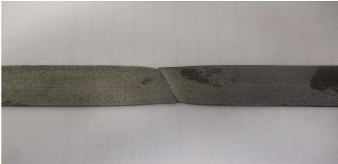
(a) Specimen with no hole after failure
