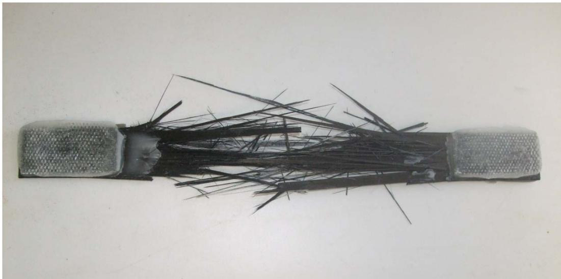
Figure 3.1: Picture of CFRP specimen after failure
