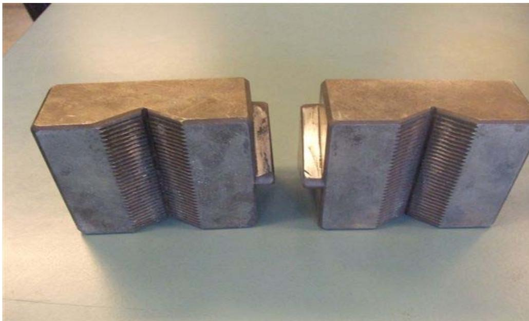
(a) The original jaws of the tensile machine
