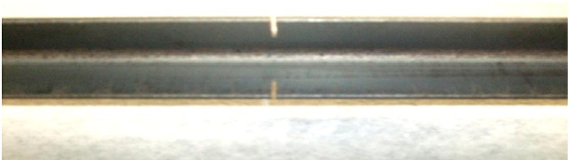
Figure 3.14: Notched steel angle
