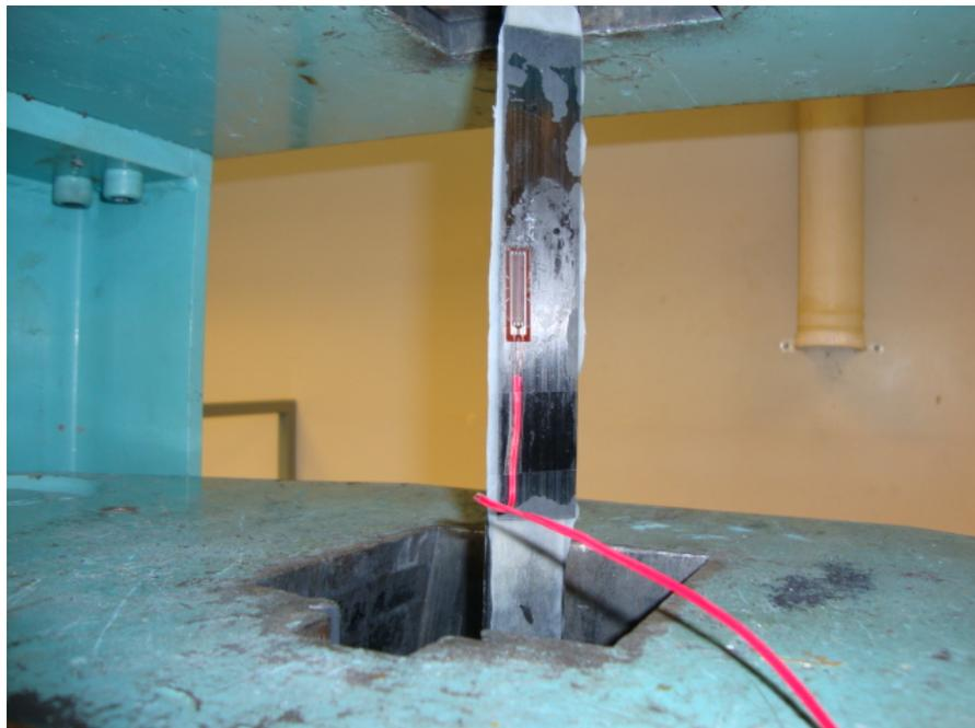
Figure 4.8: Attaching of strain gauge to CFRP strip
