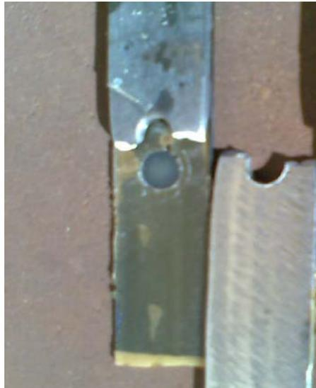
Figure 3.10: Reinforcing steel specimens after failure
