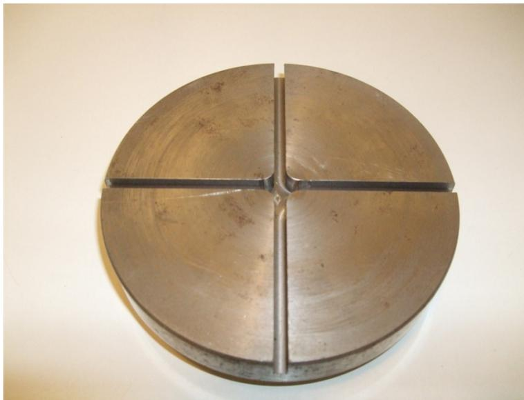
Figure 3.5: Grooved steel disc used in compression test
