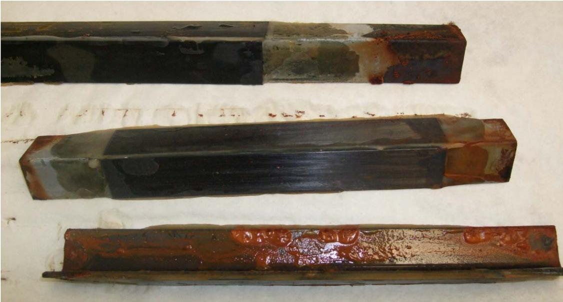
Figure 3.16: Angle specimens after 1000 hours under water
