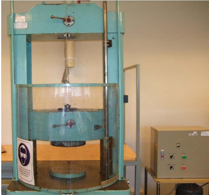
Figure 3.3: The tensile and compression testing machine used for angles
