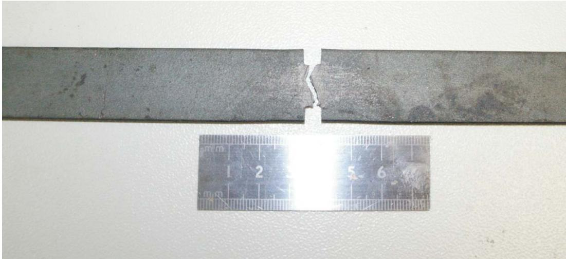
(c) Specimen with edge notch after failure
