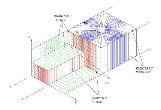
Figure 1: Lines Representation (3-D) of the Fields of  $\text{TE}_{10}$  Mode in a Rectangular Waveguide
