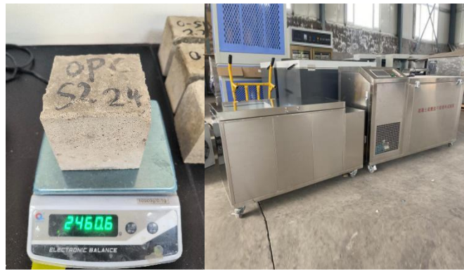
Figure 4- 7 Sulphate attack resistance test.
