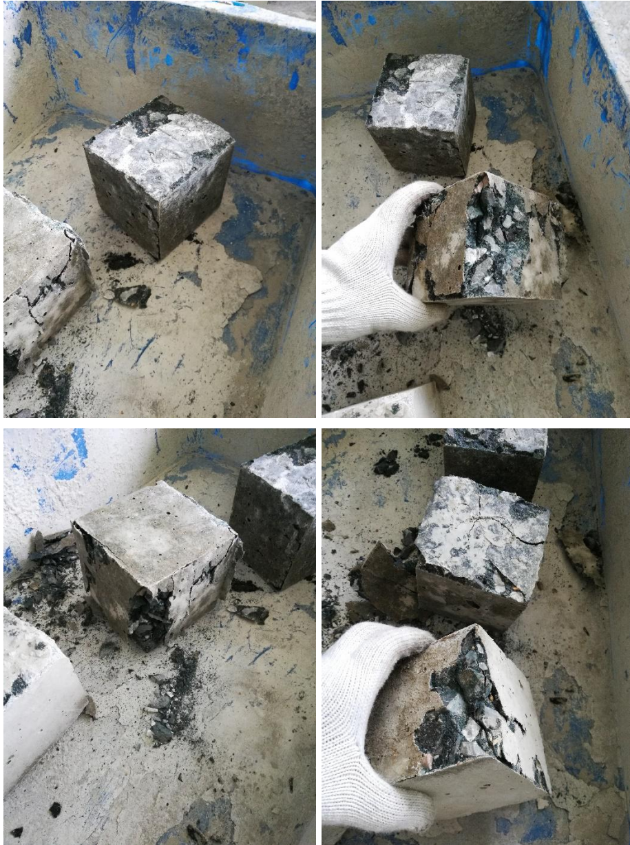
Figure E- 1 Durability of hybrid alkaline cement on compressive strength.
