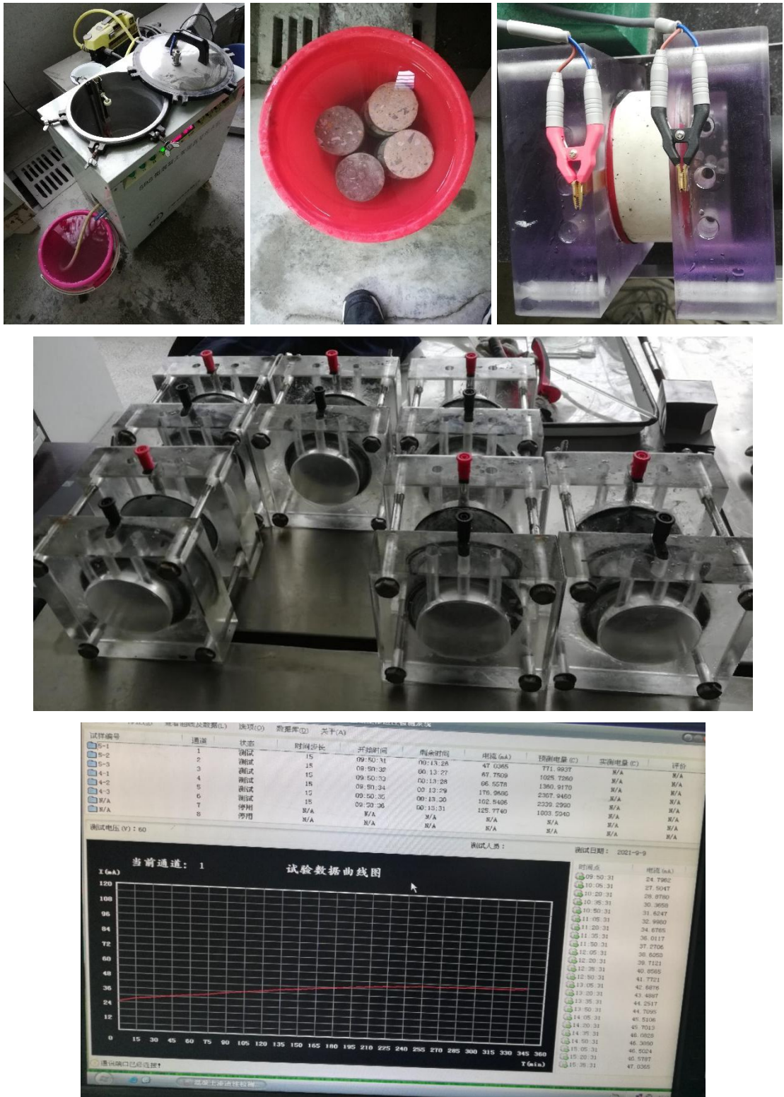
Figure F- 1 Durability of hybrid alkaline cement to chloride penetration.
