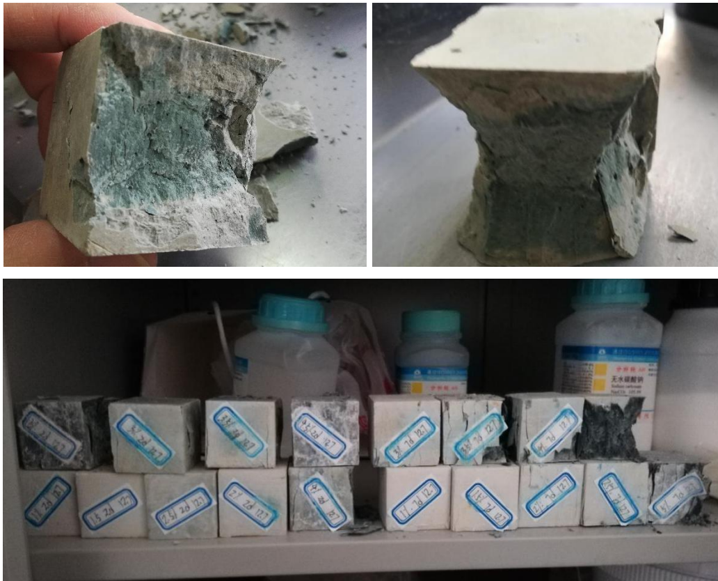
Figure B- 1 Mechanical strength preparation and test for HAC past.
