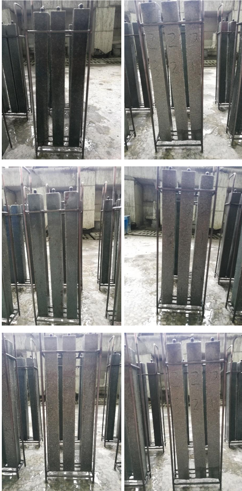
Figure H- 1 Durability of hybrid alkaline cement to alkali-aggregate reaction.
