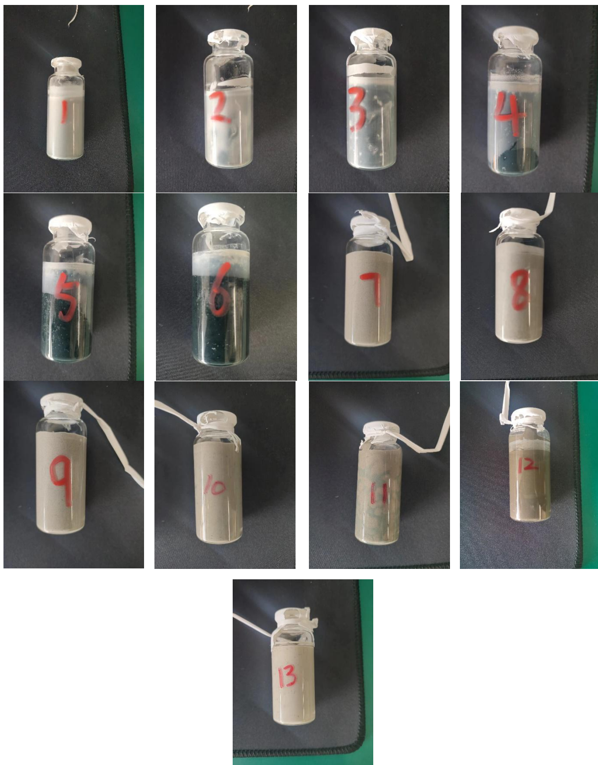
Figure C-1 ^1\text{H} NMR testing of all binder systems during the setting period.
