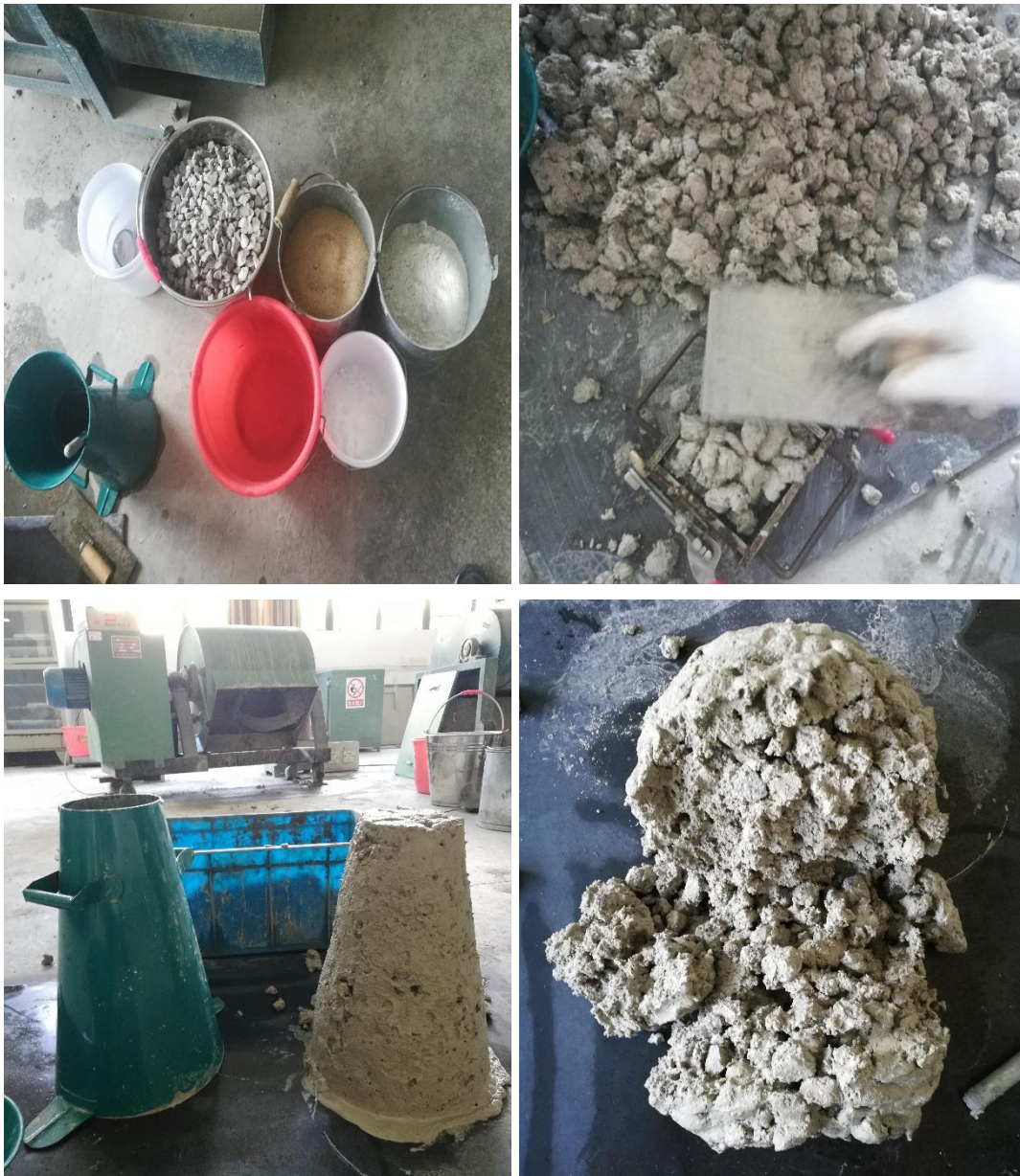
Figure D- 1 Poor workability of HAC fresh concrete.
