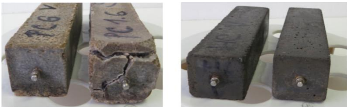
(a) OPC mortar immersed 4 years in \text{Na}_2\text{SO}_4
