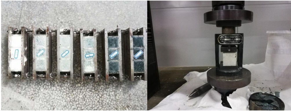
Figure 4-3 HAC paste specimens preparation and mechanical test.
