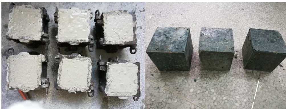
Figure 4-4 HAC concrete specimens preparation and mechanical test.
