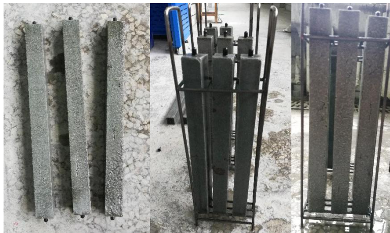
Figure 4-8 Resistance to the alkali-silica reaction test.
