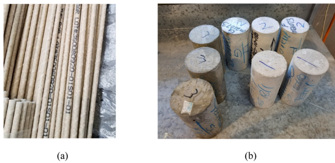
Fig. 2. (a) #3 GFRP Bars; (b) Cylindrical concrete samples.
