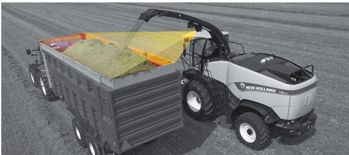
Figure 11: New Holland IntelliFill™ imaging system (New Holland Agriculture, 2020a)
