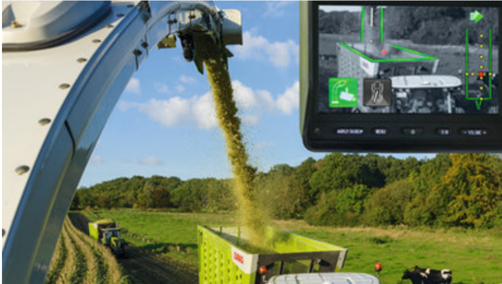
Figure 15: CLAAS AUTO FILL operation (CLAAS, 2020a)
