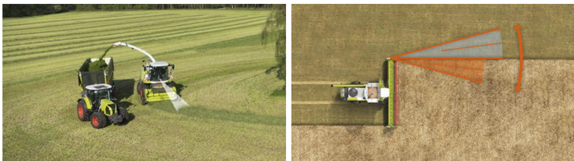
Figure 14: CLAAS CAM PILOT sensor operation and LASER PILOT visualisation (CLAAS, 2020b & CLAAS, 2020e)
