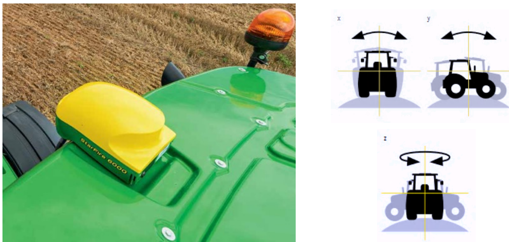
Figure 2: Starfire 6000 guidance system and terrain compensation (John Deere, 2019)
