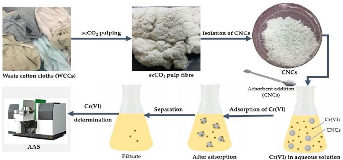
Fig. 4 CNCs have demonstrated remarkable effectiveness as adsorbents in the process of wastewater treatment [102]
