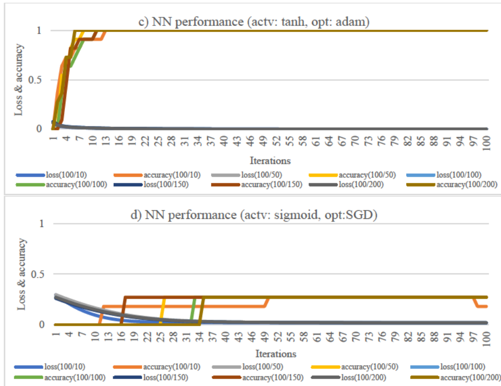
Figure 32 – NN’s performance with varying epoch and batch size against different activation functions and optimizers
