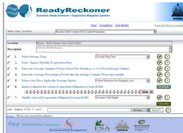
Figure 5: Ready Reckoner to determine the economics of evaporation mitigation systems
