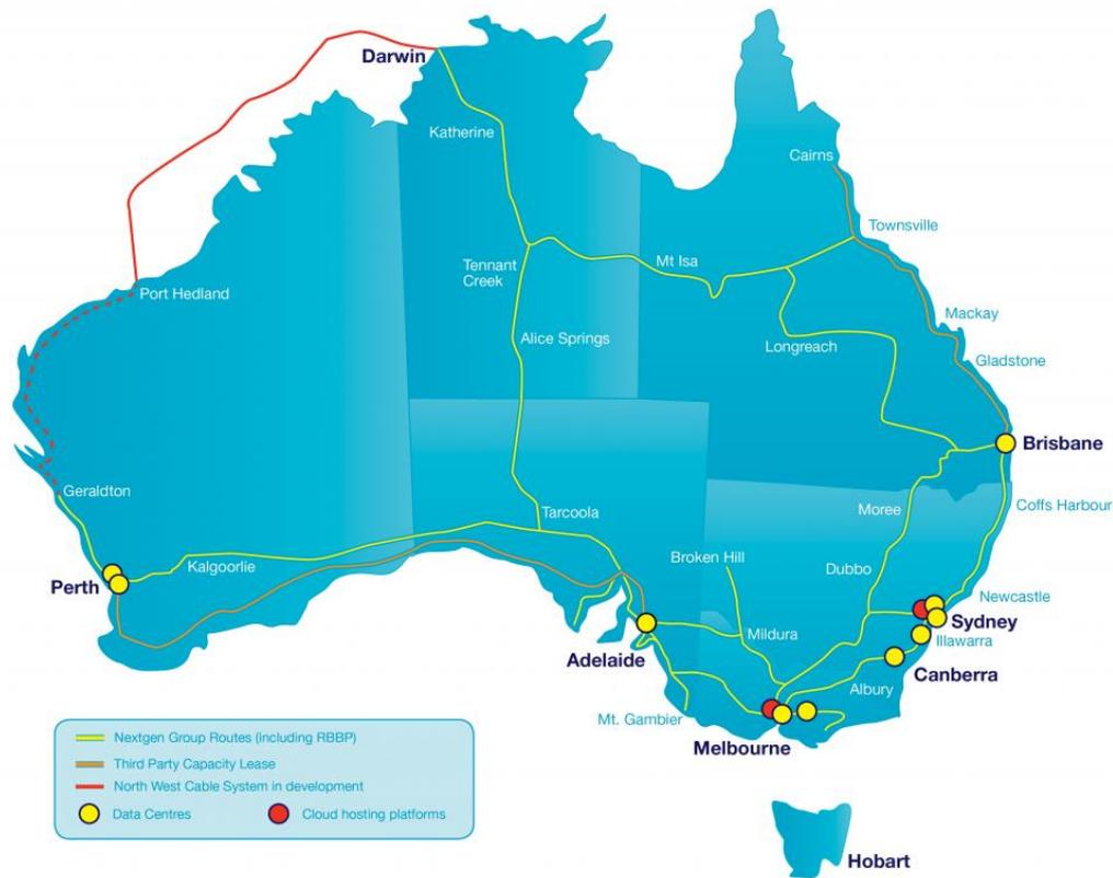
Figure 4-25 NextGen group fibre optic backbone network
