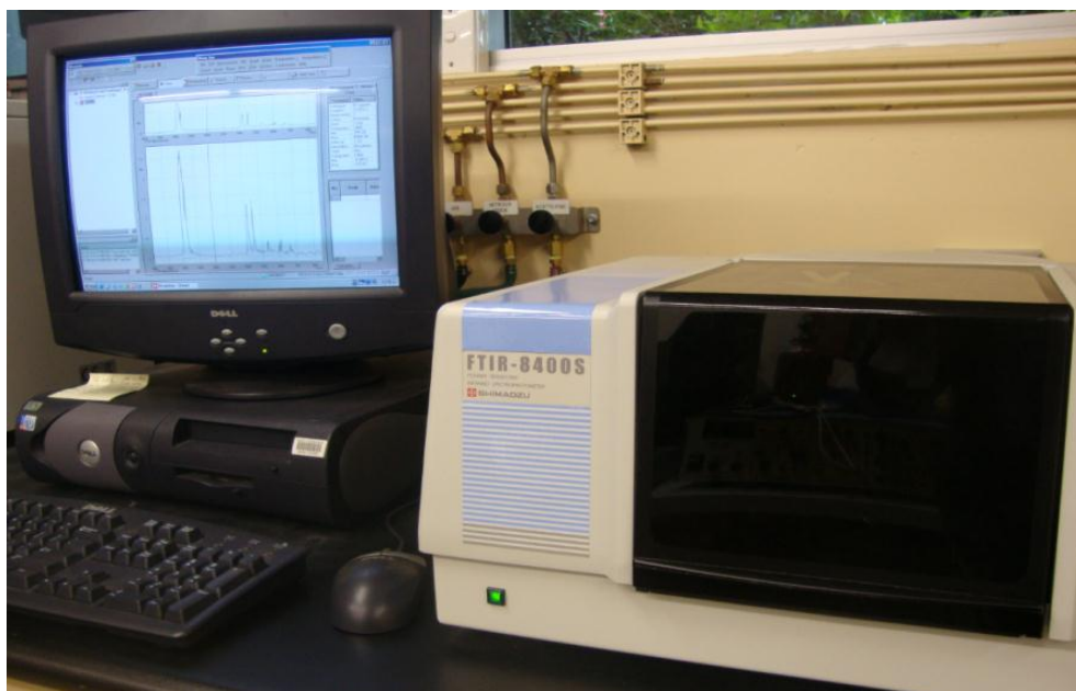
Figure 3.16: The FTIR spectrophotometer employed in measuring the IR absorption of the dosimeters.
