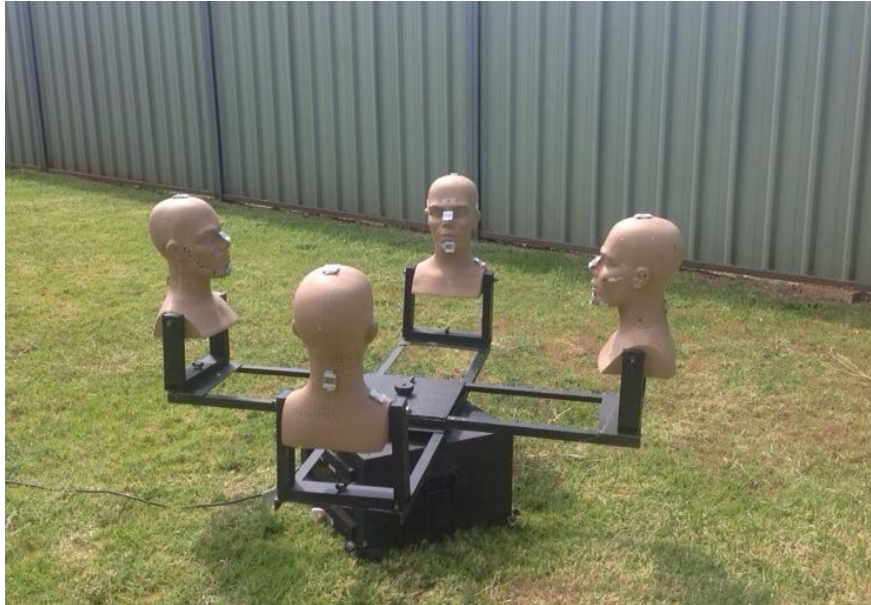
Figure 5.1: The experimental set-up for the anatomical exposure measurements showing the PVC and PPO dosimeters attached to chosen spots on manikins that were mounted on a rotating platform.
