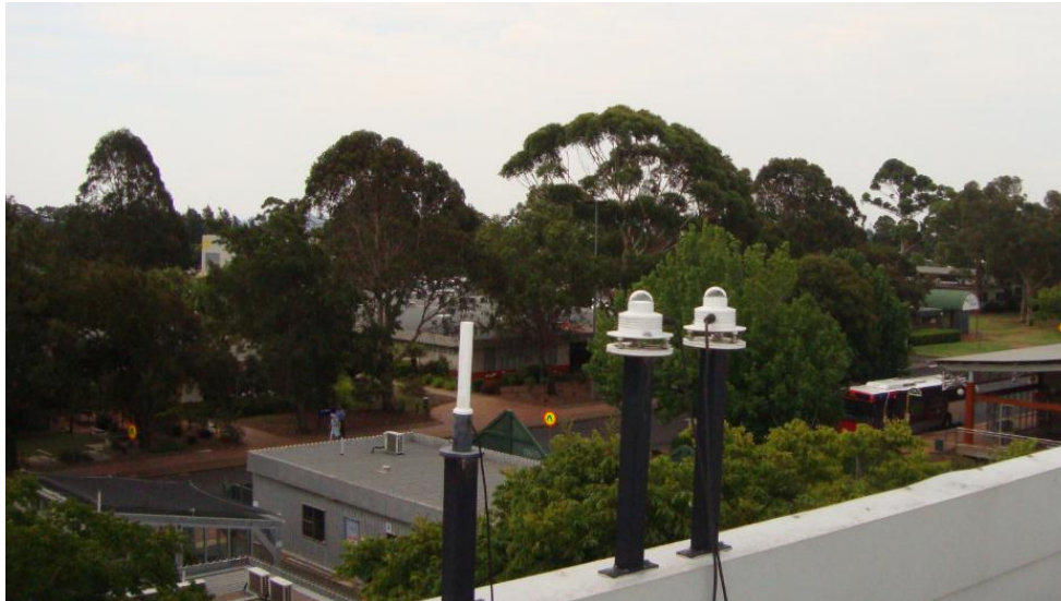
Figure 3.15: The outdoor UVB Biometer mounted on the roof of a USQ building.
