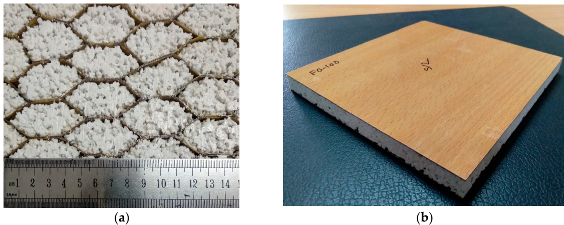
Figure 5. Photograph of (a) perlite/sodium silicate foam-filled paper honeycomb core and (b) sandwich structure made of perlite/sodium silicate foam core with Formica sheet as skin.
