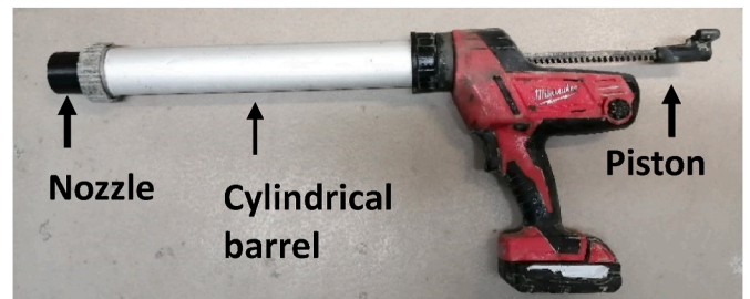
Fig. 4. A customised 3D printer consists of a piston-type extruder.
