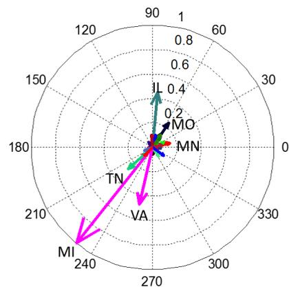
FIGURE 14. Mode shape of the 1.2 Hz Inter-area mode (65% PV).
