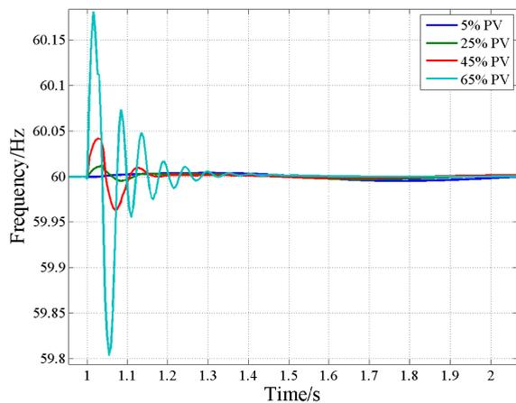
FIGURE 9. Local oscillation changes as PV penetration increases (TN).
