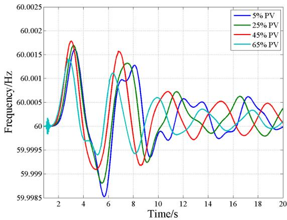
FIGURE 8. Oscillation frequency change as PV penetration increases (CT).
