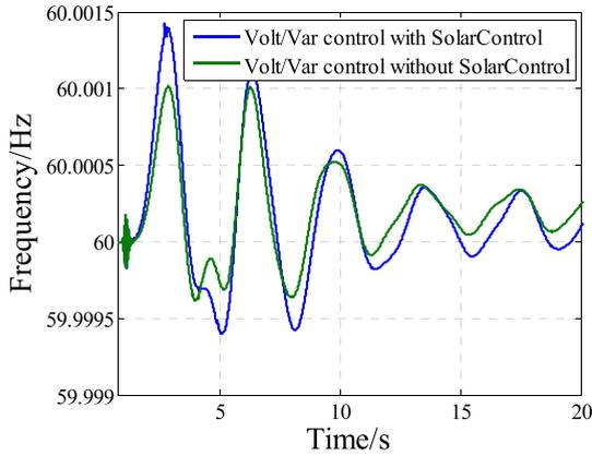
FIGURE 11. Oscillation frequency in CT under different PV power plant control strategies (65% PV).
