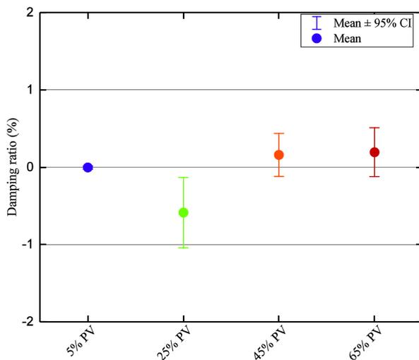
**FIGURE 16.** Damping ratio change with PV penetration (1.2 Hz mode).
