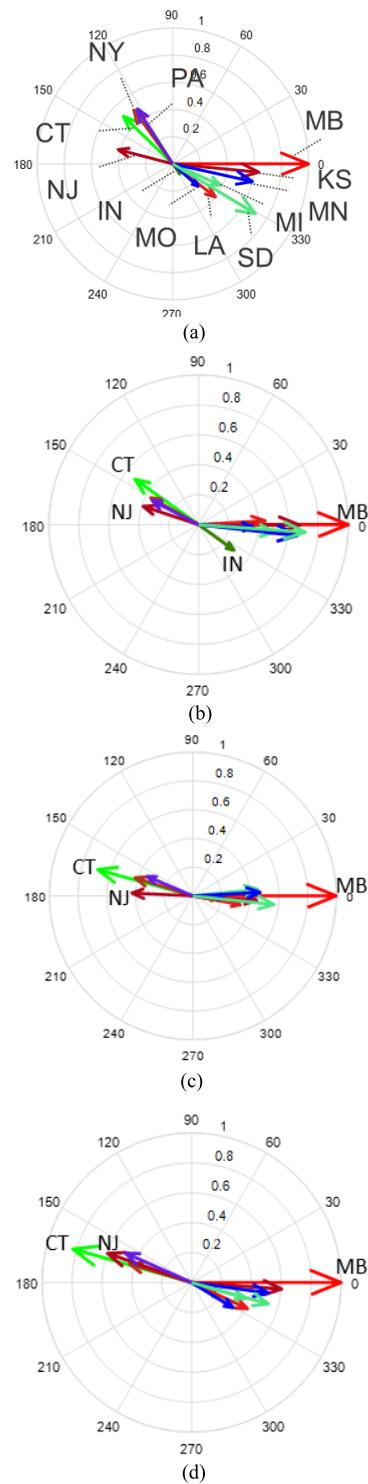
FIGURE 10. Mode shape change with PV penetration. (a) 5% PV. (b) 25% PV. (c) 45% PV. (d) 65% PV.
