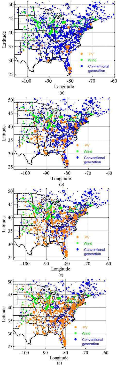
**FIGURE 4.** PV distribution in different scenarios. (a) 5%PV + 15%WT. (b) 25% PV + 15%WT. (c) 45%PV + 15%WT. (d) 65%PV + 15%WT.
