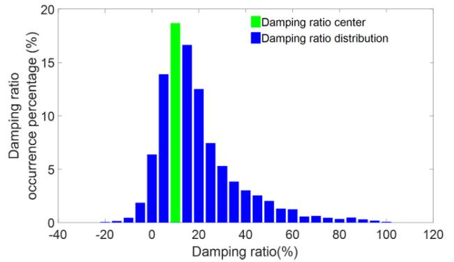
FIGURE 2. Damping ratio distribution of inter-area oscillations.
