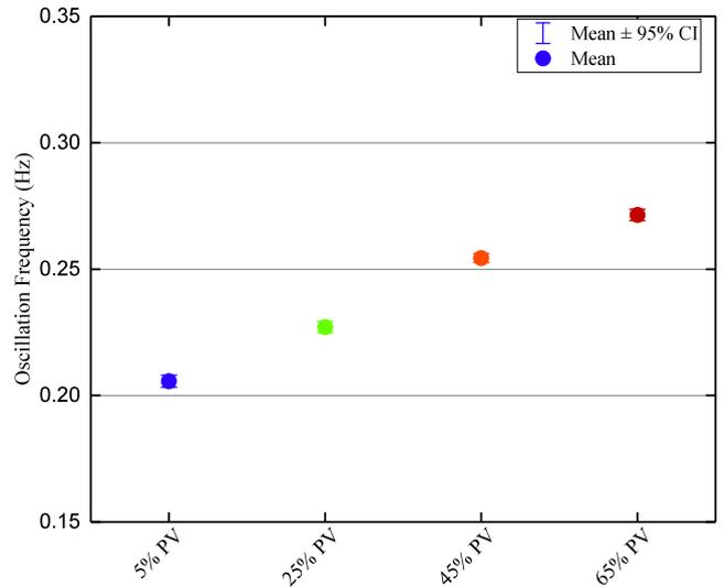
**FIGURE 6.** Oscillation frequency change as PV penetration increases.
