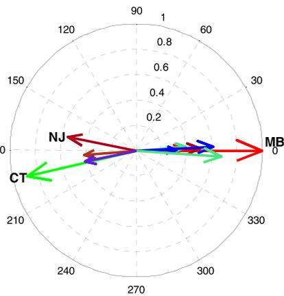
FIGURE 12. Oscillation mode shape at 65% PV (Control Strategy 2).
