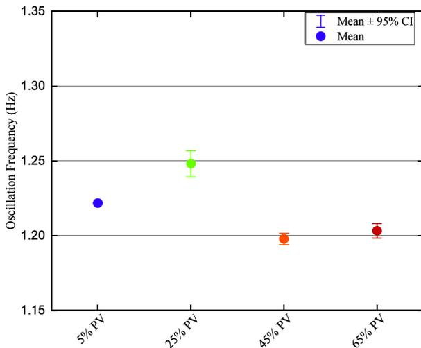
**FIGURE 15.** Oscillation frequency change with PV penetration (1.2 Hz mode).
