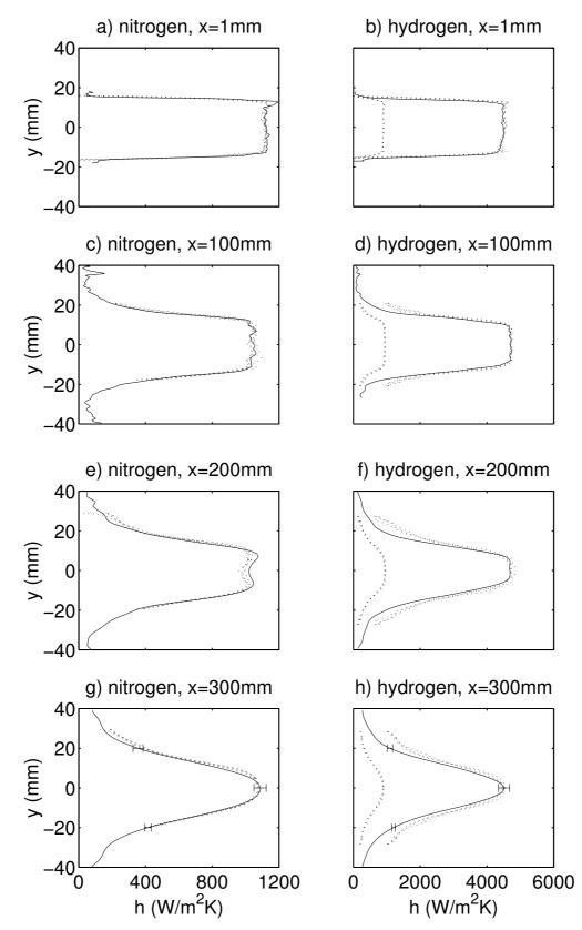
Fig. 8 Time-averaged heat transfer coefficient results at 4 stations downstream of injection. Solid lines: thin film probes; dots: Pitot probe predictions
