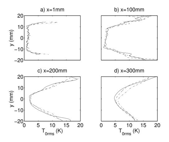
Fig. 10 Stagnation temperature fluctuations at 4 stations downstream of injection for three different values of  $T_0$ - $T_w$
