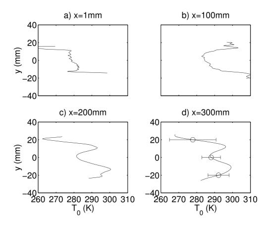
Fig. 7 Time-averaged stagnation temperature measurements in the hydrogen jet at 4 stations downstream of injection
