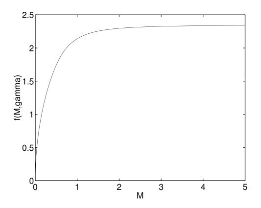
Fig. 2 Sensitivity of heat transfer coefficient to Mach number as indicated by  $f(M_{\infty}, \gamma)$  for  $\gamma = 1.4$
