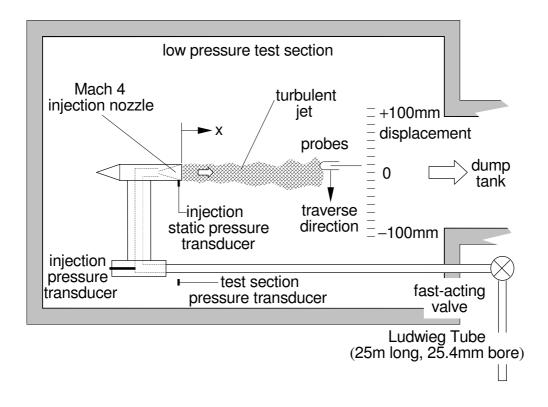
Fig. 4 Illustration of the Mach 4 free jet arrangement
