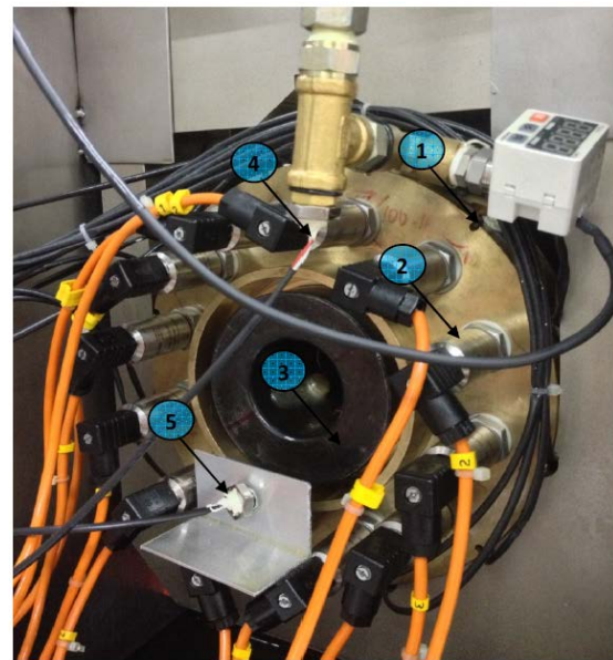
Fig. 2: Housing with pressure and temperature sensors. (1) Temperature sensor (2) Pressure sensor (3) Shaft (4) Temperature inlet (5) Temperature outlet
