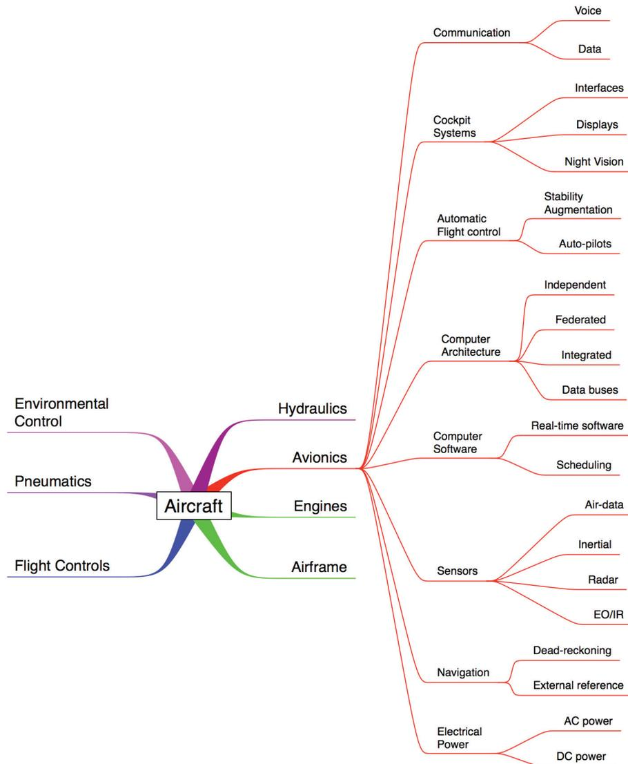
**Figure 6-8.** Expanded avionics system detail to support development of learning objectives
