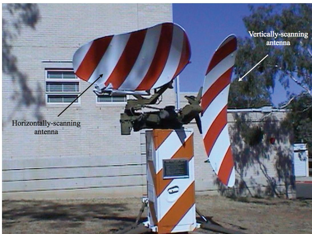
**Figure 5-7.** Static radar system display of a ground-controlled precision approach radar with vertically and horizontally scanning antennas.
