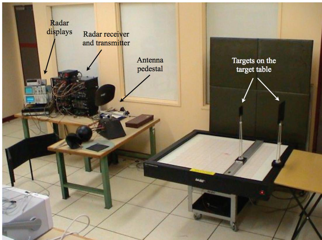
**Figure 5-6.** The indoor radar trainer consisting of the transmitter, antenna, target, receiver and display.
