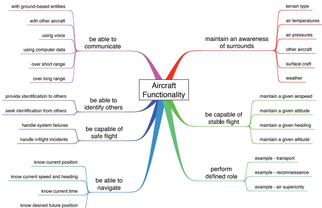
**Figure 6-5.** Expanded aircraft functionality mind map.
