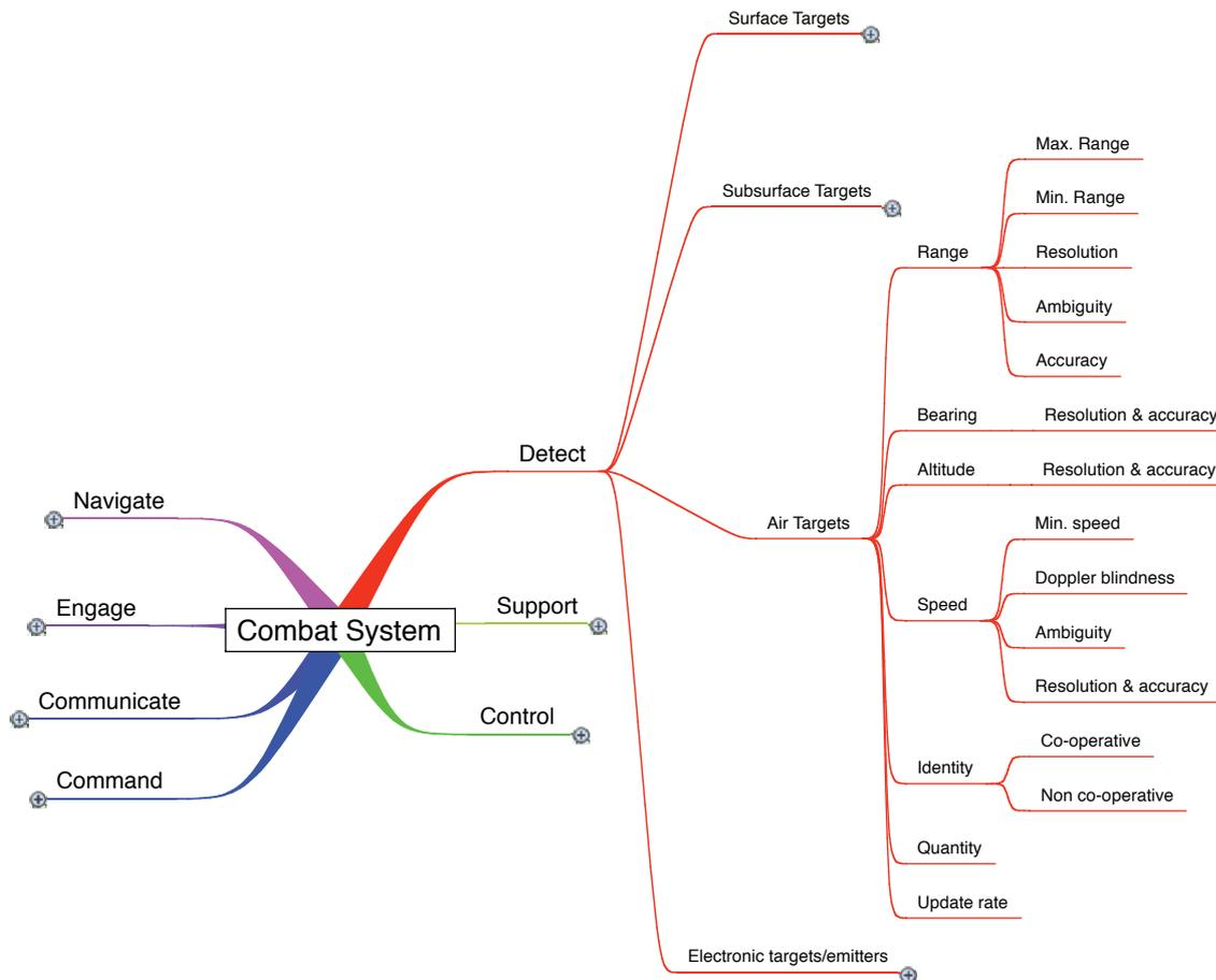
Figure 5-5. Radar-related issues pertaining to air targets
