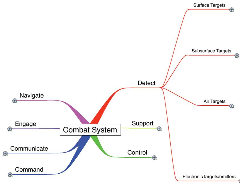
**Figure 5-3.** Detect functionality
