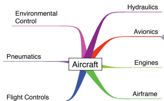
**Figure 6-6.** Avionics systems in context with the other aircraft systems.
