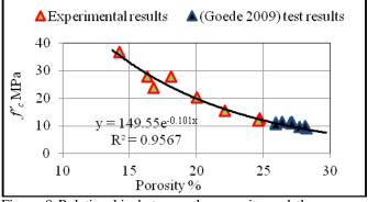
Figure 8 Relationship between the porosity and the compressive strength.
