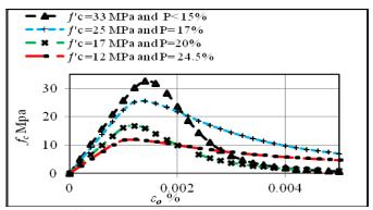
Figure 6 Effect of porosity on the stress-strain curve of the permeable concrete specimen.
