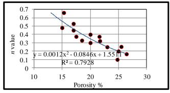
Figure 7 Relationship between the porosity and the material parameter (n).
