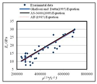
Figure 5. The relationship of experimental and calculated  $E_o$  versus  $\rho^{1.5} \times f_c^{0.5}$
