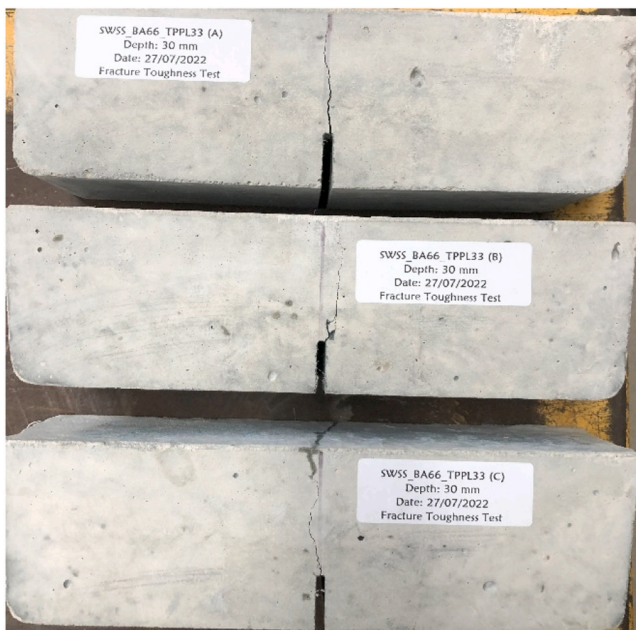
Fig. 4. Typical fracture toughness failure mode.
