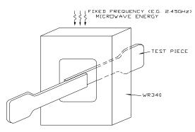
a) 2.45 GHz Microwave Energy launched into a Single Mode Applicator
