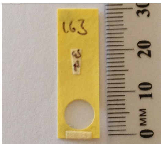
Figure 1 – Photograph of a fabricated miniaturized UVA dosimeter.
