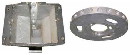
Base of the seed box (air jet removed) A plate with conical shaped cells
