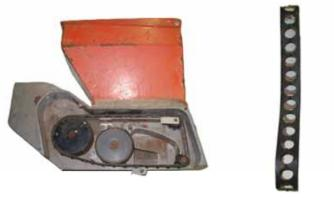
Side view of belt type precision meter Metering belt
