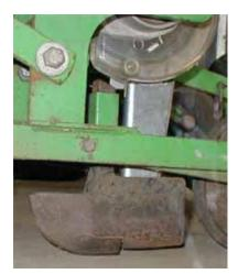
Figure 201: Seed delivery by gravity drop through a short dropper tube
