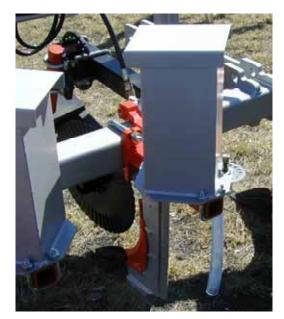
Figure 166: An example of a stationary opening type seed meter used for pasture renovation
