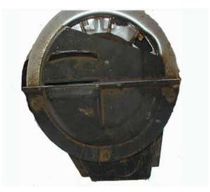
Figure 199: An example of a finger pick-up type precision seed meter
