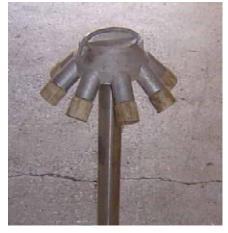
Figure 210: A simple moulded plastic dividing head
