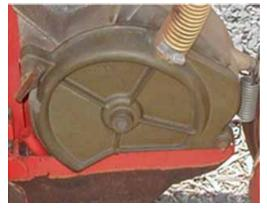
Figure 200: Seed delivery by gravity drop through the rear, split cavity of a runner opener
