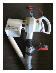
Figure 2: Hand piece, venturi, conveyance tube, and air splitting control valve
