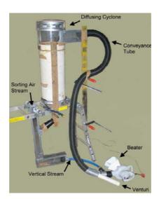
Figure 3: The full prototype test system as built. It is noted that the venturi in this picture has not been connected to the beater handpiece.
