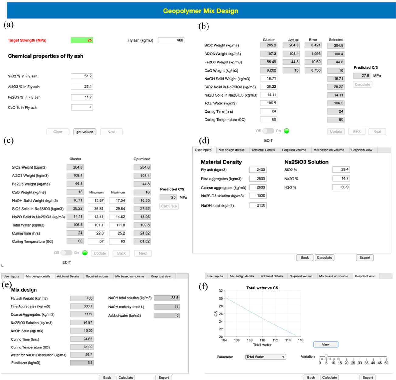
Fig. 9 User interface for mix design calculation: a obtaining user input, b selecting optimum cluster, c parameter optimization, d material density input, e mix design output, and f parameter sensitivity
