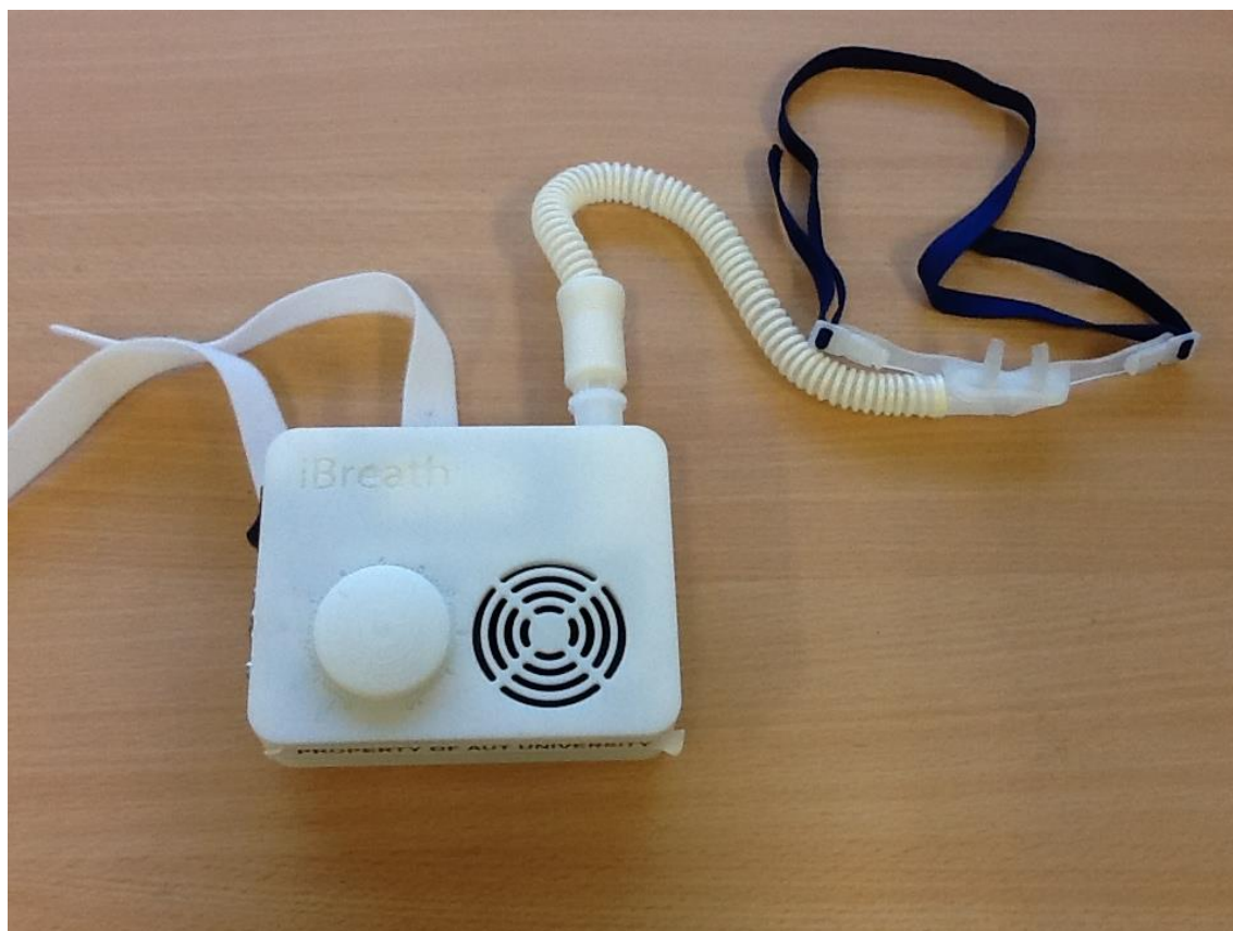
Figure 1. The non-invasive ventilation device used during everyday tasks in thermo-neutral and hot-humid conditions.
