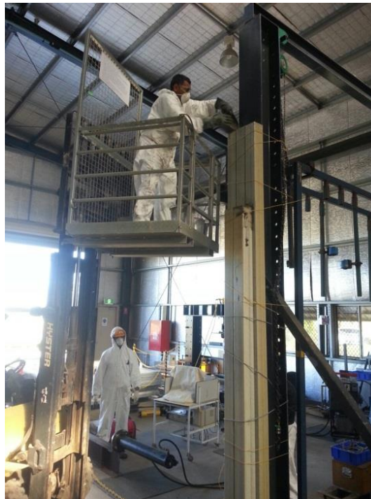
Figure 2. Filling process of the pultruded beams with concrete.
