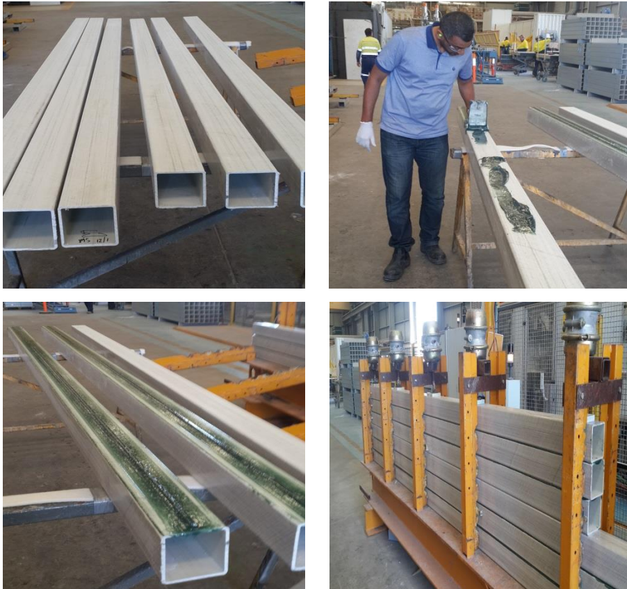
Figure 1. Preparation process of pultruded sections assembly.
