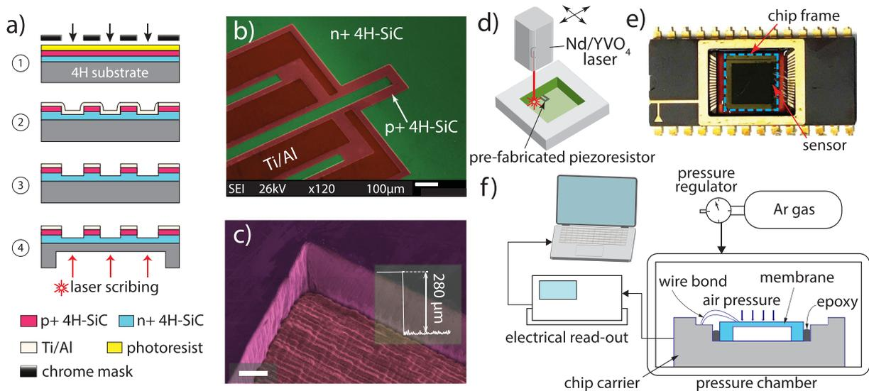
Fig. 2. a) Fabrication process of 4H-SiC pressure sensor. b) SEM image of the sensor on the top surface of a diced chip. c) SEM image of the back side of the diaphragm after laser scribing. Scale bar, 100 μm. d) Alignment of laser scribing on the back side with respect to the pre-fabricated sensor on the front side. e) Sensor chip attached to a chip carrier with bonding wire. f) Experimental setup for the pressurising characterization.
