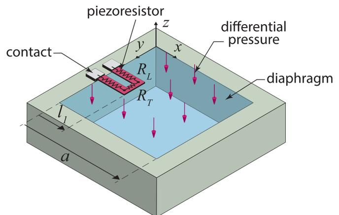
Fig. 1. Design and configuration of 4H-SiC pressure sensor.
