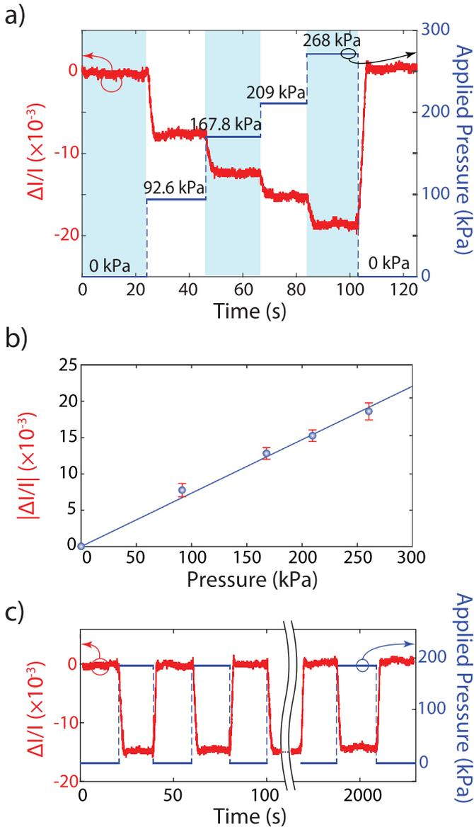
**Fig. 3.** a) Real-time measurement of output signal at varying applied pressure ranging from 0 to nearly 270 kPa. b) Linear resistance change upon the application of pressure. c) Output signal at a cyclic applied pressure of 186 kPa, high signal-to-noise ratio and the excellent repeatability without significant signal drift were obtained.
