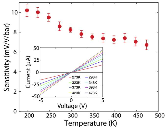
**Fig. 4.** The measured sensitivity at various temperature ranging from 198 K to 473 K. It is worth noting that the decreasing of sensitivity with increasing temperature is in good agreement with the hole transfer mechanism under strain with the varying temperature. Inset: Linear current-voltage characteristics of the sensor measured at various temperatures.
