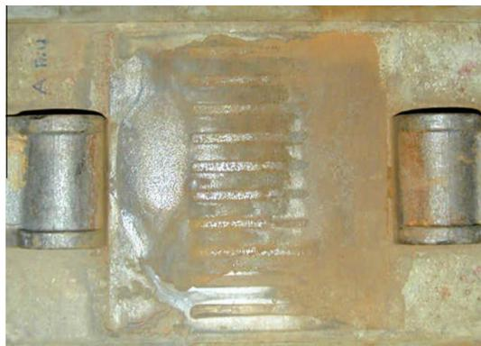
Fig. 23. Steel plate covering rail-seat after 10 million cycles [56].
