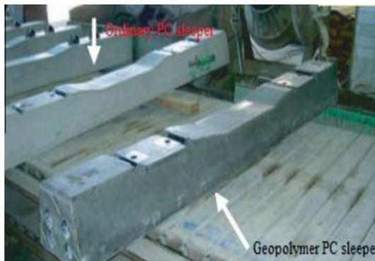
Fig. 25. Ordinary and geopolymer prestressed concrete sleepers [72].
