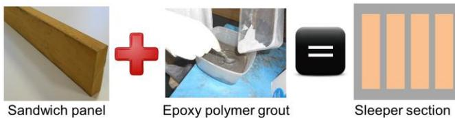
Fig. 2: Composite sleeper concept
