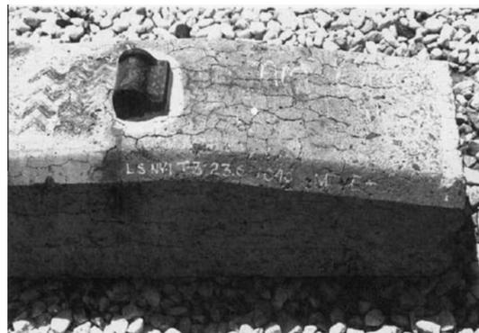
Fig. 14. Cracking of prestressed concrete sleeper due to DEF [40].
