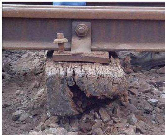
**Fig. 2.** Failure of timber sleeper due to fungal decay [6].
