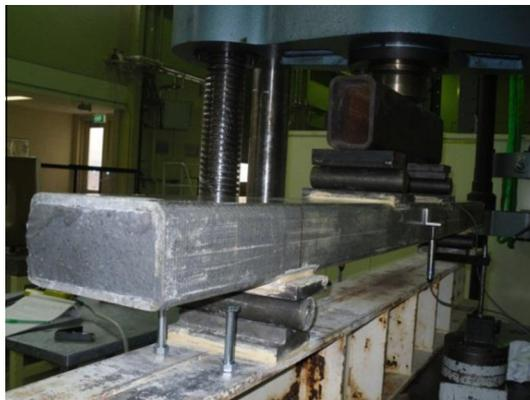
Fig. 26. Geopolymer concrete-filled pultruded composite sleeper [74].
