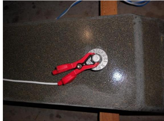
(b) applying voltage between two rail-seats
