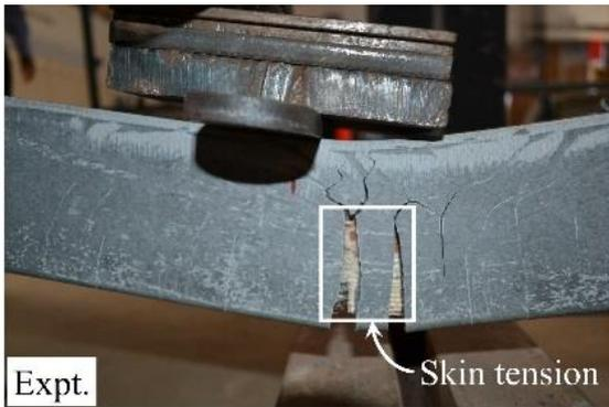
(e) VF-A<sub>400</sub> at 40.1 kN
