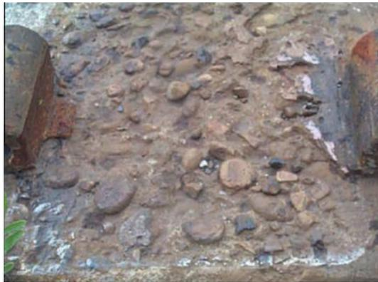
Fig. 6. Failure of concrete sleeper due to rail-seat abrasion [23].
