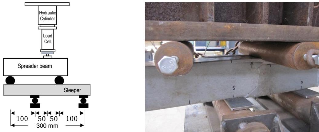
(a) asymmetrical beam shear test setup
