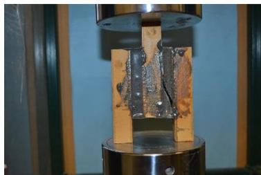
(e)  $F_{40}l_{70}t_{m10}b_{20}$  (Cohesive)
