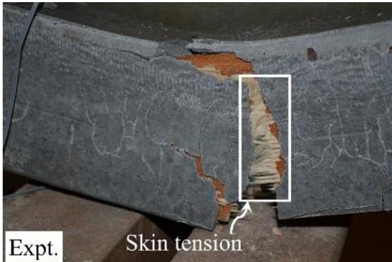
(f) VF-A<sub>200</sub> at 76.4 kN
