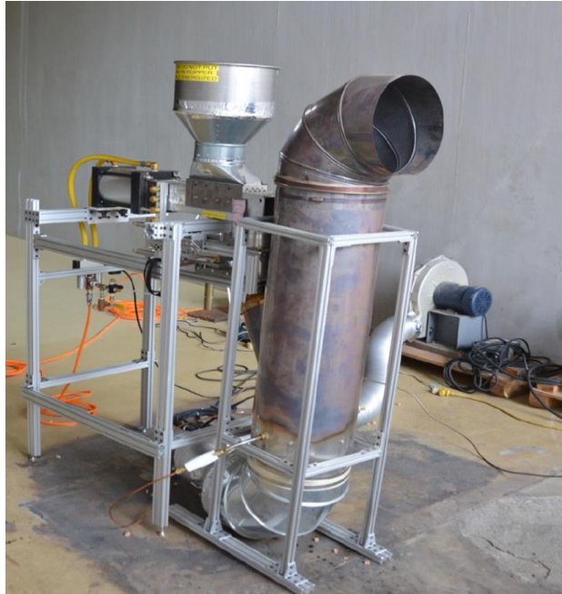
Figure 2.7 Picture of NIST continuous feed firebrand generator for full scale experiments (Manzello & Suzuki 2013).
