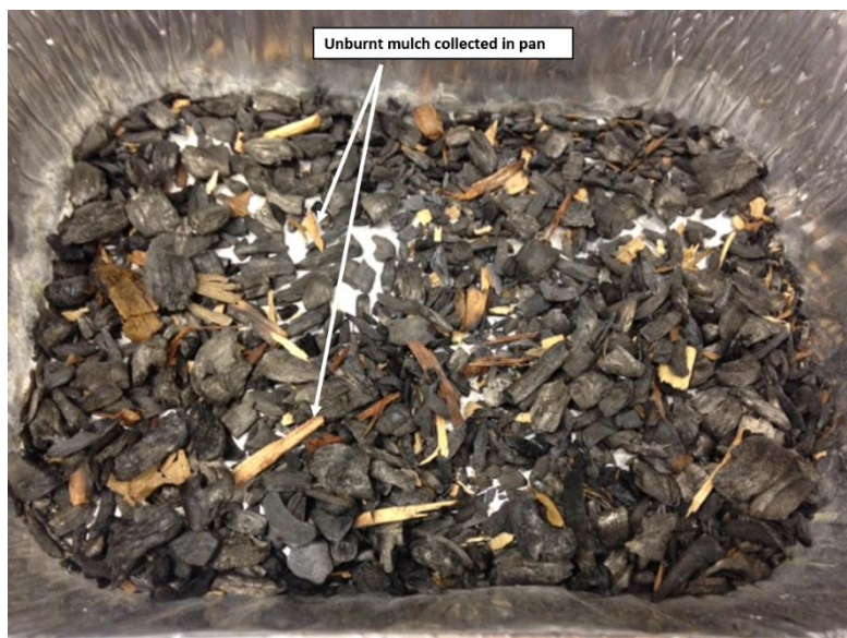
Figure 4.15 Collected firebrands in experiments with flap of 150 mm and high wind speed.
