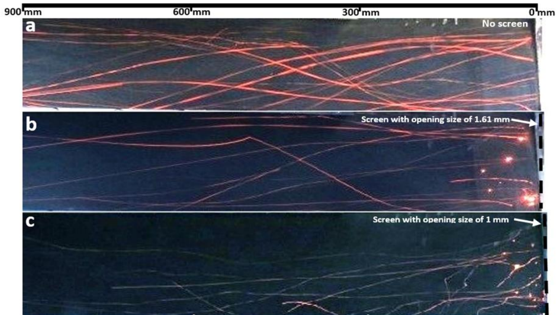
Figure 5.13 Captured pictures of firebrand traces in the test section of the wind tunnel at wind speed of 10 m/s under the experimental conditions of; a) no-screen, b) screen with the opening size of 1.6 mm, and c) screen with the opening size of 1 mm.
