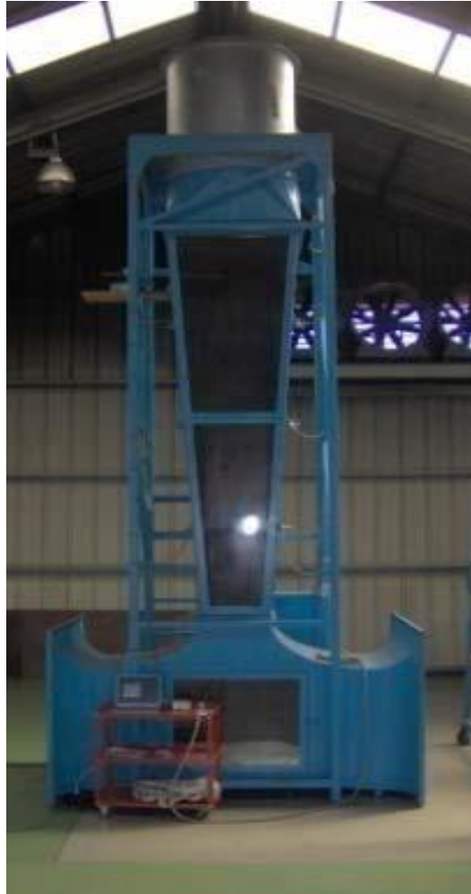
Figure 2.4 Vertical wind tunnel used by Almeida et al. for experiments on firebrands (Almeida et al. 2009).
