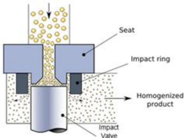
*Figure 7: Diagrammatic disintegration of waste activated sludge by high-pressure homogenisation (Genizer 2009)*
