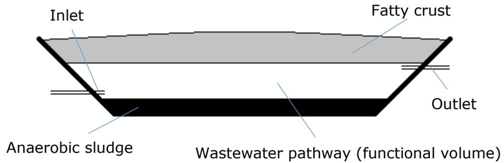
*Figure 4: Illustration of dead space contributed by crust and sludge volume resulting in a large reduction in functional pond volume.*
