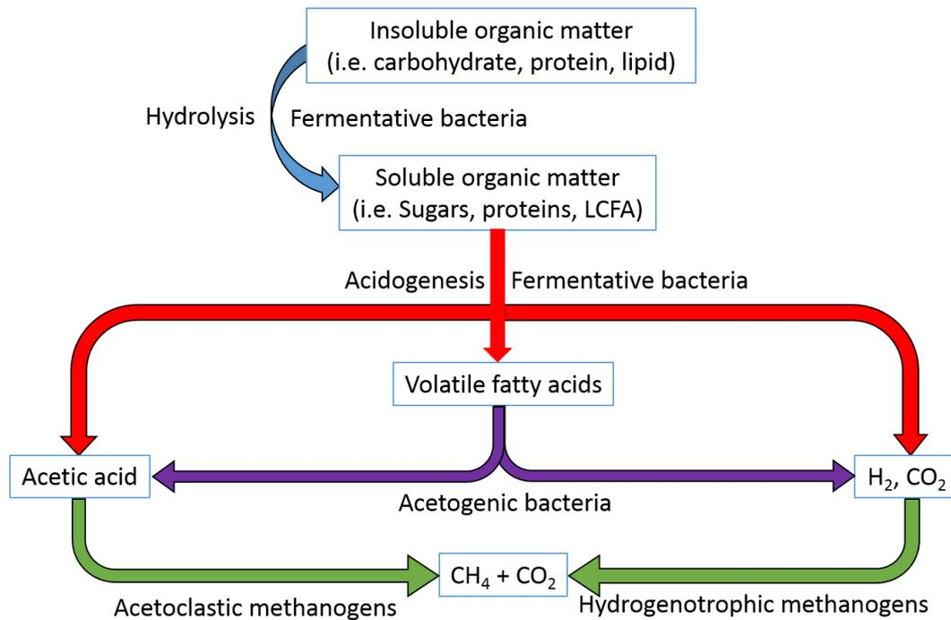
Figure 2: Stages of anaerobic digestion, modified from Appels *et al.* (2008).
