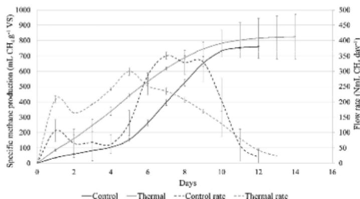
Fig. 1. Specific methane production and flow rates for controls and thermobaric treated DAF sludge measured during biochemical methane potential test. (Avg  $\pm$  SD; Control  $n = 3$ , thermobaric  $n = 6$ ).
