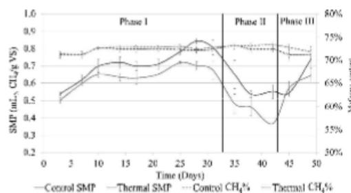
Fig. 2. Gas flow rates and methane content. Values are the average of 3, with error bars representing one standard deviation.
