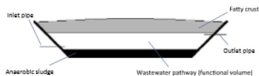
Fig. 2. Illustration of dead space contributed by crust and sludge volume resulting in a large reduction in functional pond volume.
