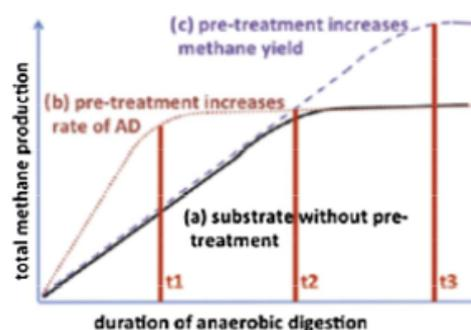
**Fig. 4.** Effect of pre-treatments on rate of anaerobic digestion and increase the methane yield [51].
