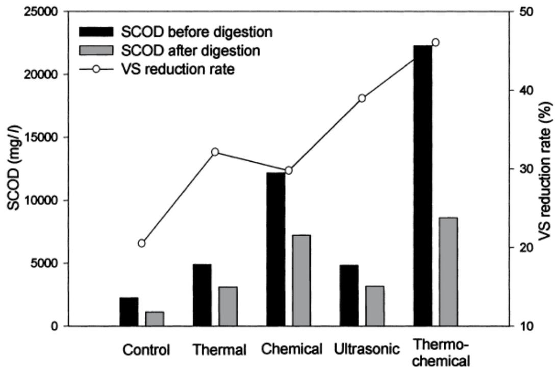
Figure 8: sCOD removal efficiency and VS reduction rate for pre-treated WAS (Kim *et al.* 2003).
