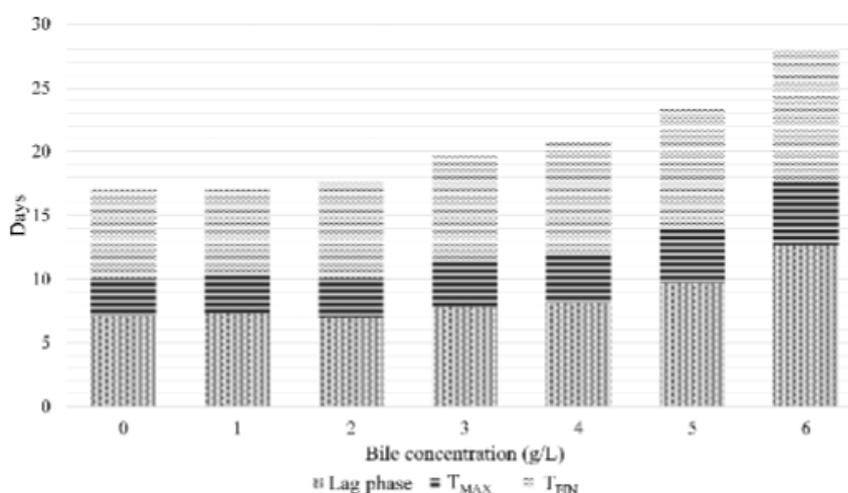
Fig. 4. Inhibition period with respect to bile addition in BMP testing.  $T_{MAX}$  represents the time between recovering from lag phase inhibition and achieving maximum methane production rate.  $T_{FIN}$  represents the time between achieving  $T_{MAX}$  and completing digestion with methane production < 1% of total yield.
