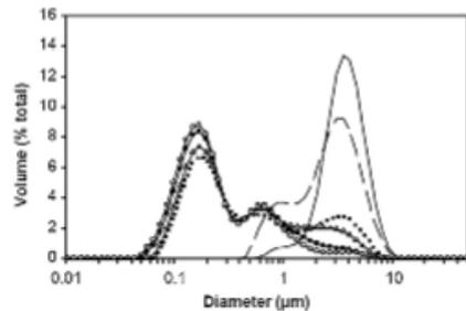
Fig. 7. Effect of homogenisation pressure on the size distribution of fat globules in milk, at an inlet temperature of 4 °C: 0.1 MPa (Control) (—), 100 MPa (---), 150 MPa (···), 200 MPa ( $\Delta$ ), 250 MPa ( $\square$ ), and 300 MPa ( $\circ$ ). Clustering was not observed at any homogenisation pressure used [72].
