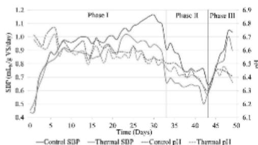
**Fig. 4.** Digester response to reduced pH, and recover with Mg(OH)<sub>2</sub>. Phase I involved the digestion of the first batch of substrate. Phase II indicates the change to a new batch of substrate on day 33. Phase III indicates the addition of Mg(OH)<sub>2</sub> on day 43.
