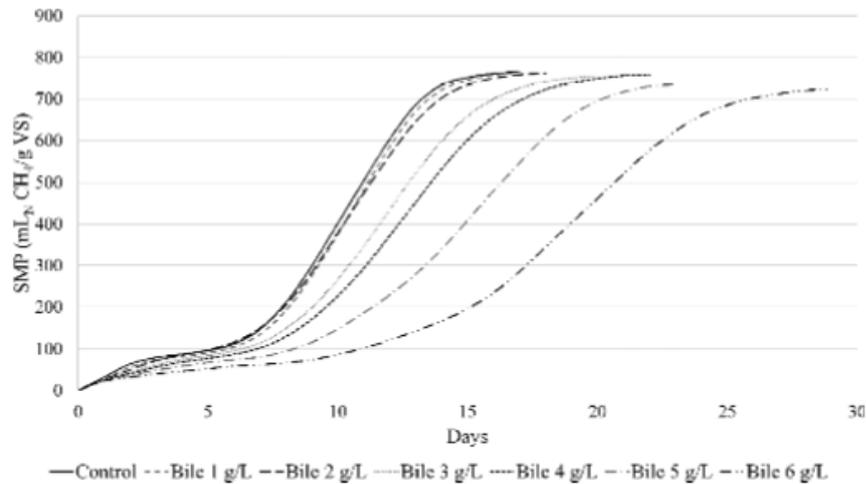
Fig. 2. Effect of high-dose bile on SMP and anaerobic digestion profile of DAF sludge.
