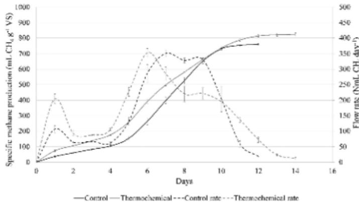
Fig. 3. Specific methane production and flow rates for controls and thermochemical DAF sludge measured during biochemical methane potential test. (Avg  $\pm$  SD;  $n = 3$ ).
