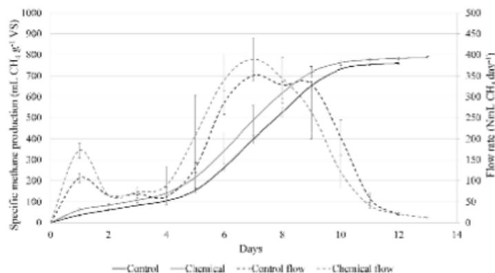
Fig. 2. Specific methane production and flow rates for controls and chemical-treated DAF sludge measured during biochemical methane potential test. (Avg  $\pm$  SD;  $n = 3$ ).
