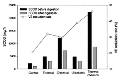
Fig. 9. SCOD removal efficiency and VS reduction rate for pre-treated WAS [50].
