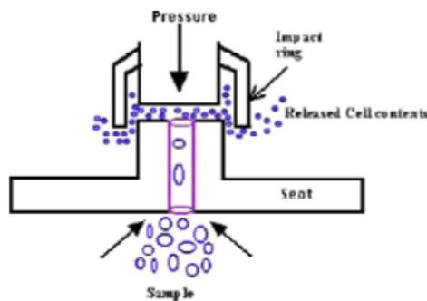
**Fig. 6.** Diagrammatic disintegration of waste activated sludge by high-pressure homogenisation [70].
