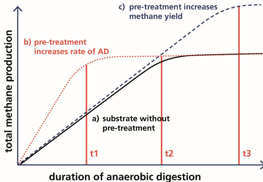
Figure 5: Effect of pre-treatments on reaction rate and methane yield from anaerobic digestion (Montgomery & Bochmann 2014).
