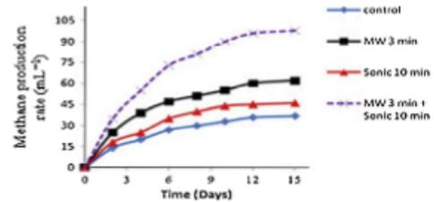
Fig. 8. Rate of methane production after microwave and ultrasonic pre-treatment [75].
