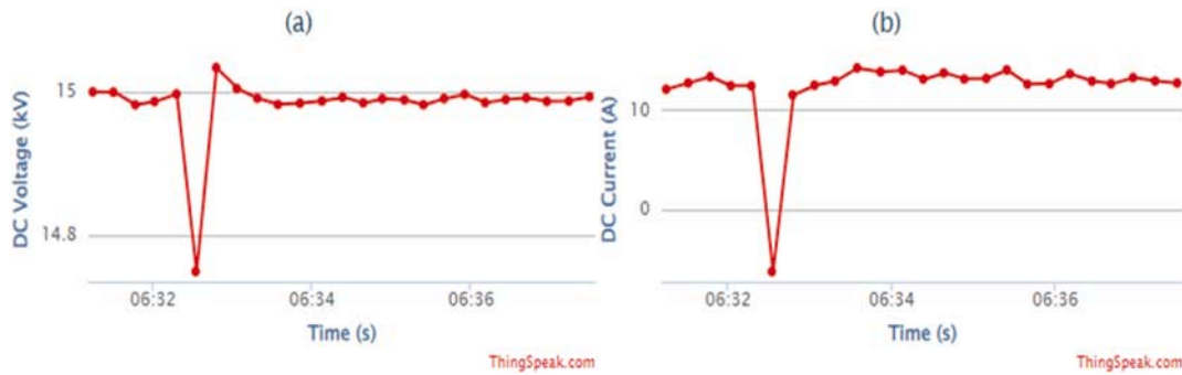
Fig. 13. MTDC condition monitoring during AC fault: (a) voltage “DC”; (b) current “DC”.
